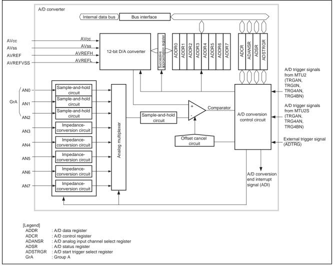
Figure 1 Block Diagram of the 12-Bit A/D Converter
