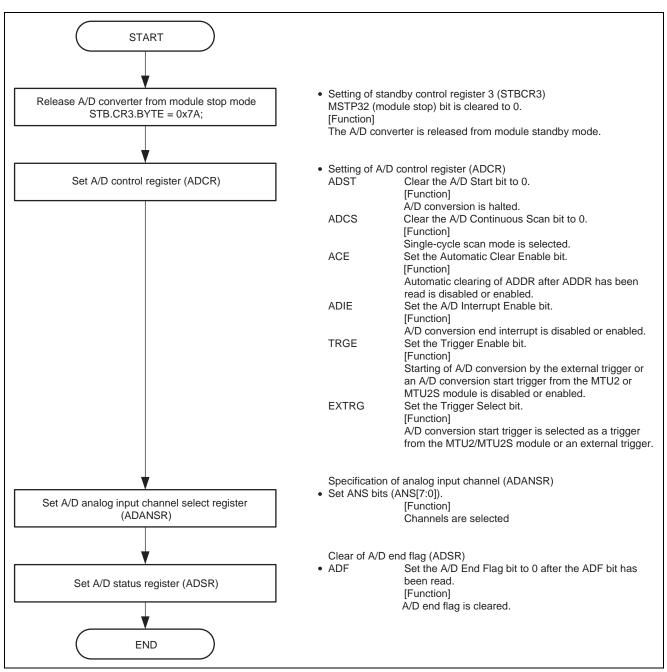
Figure 2 Initialization Sequence for 12-Bit A/D Conversion
