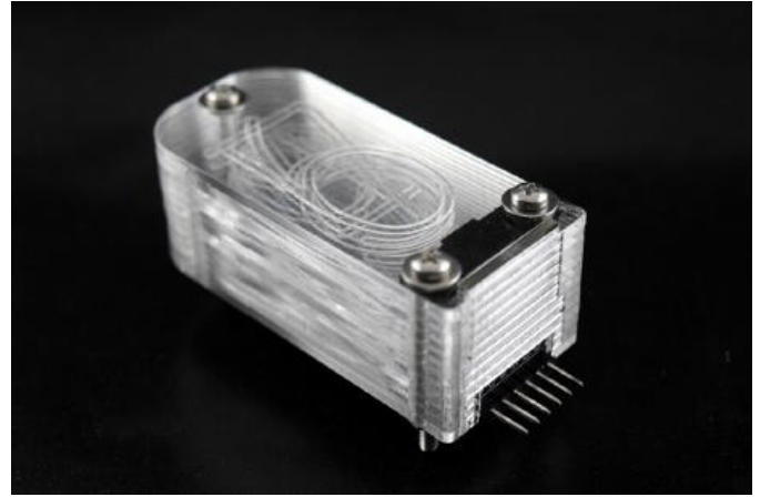
Figure 14. Completed tube showing 6 I/O pins
