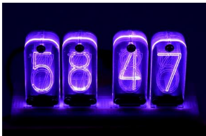
Figure 17. Four pseudo Nixie digits of a digital clock showing 58:47. These are mounted on a breadboard
