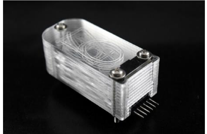
Figure 14. Completed tube showing 6 I/O pins
