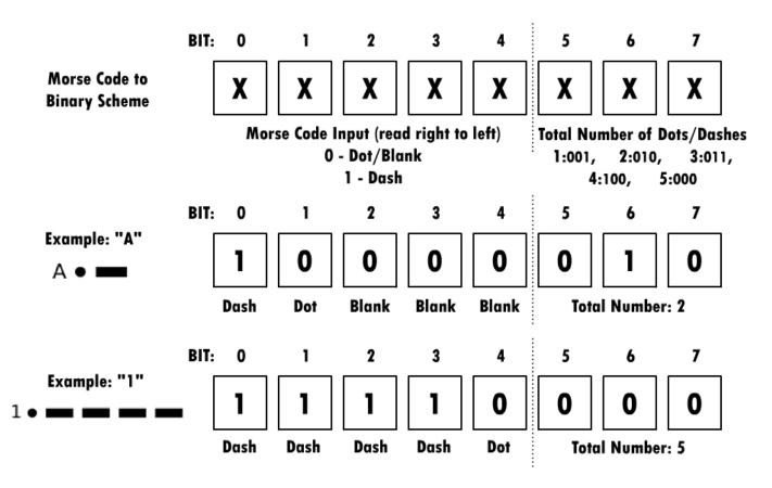
Figure 2. Conversion from Morse Code input to byte of alphanumeric data
