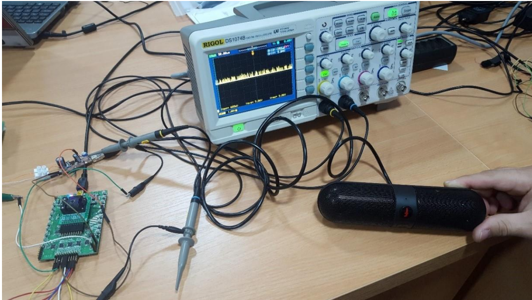
Figure 26. Boost implementation test charging Bluetooth speaker
