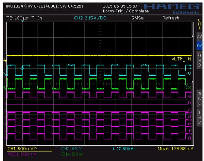
1. 90 mV on ADC input ('0' and '9' are displayed)
