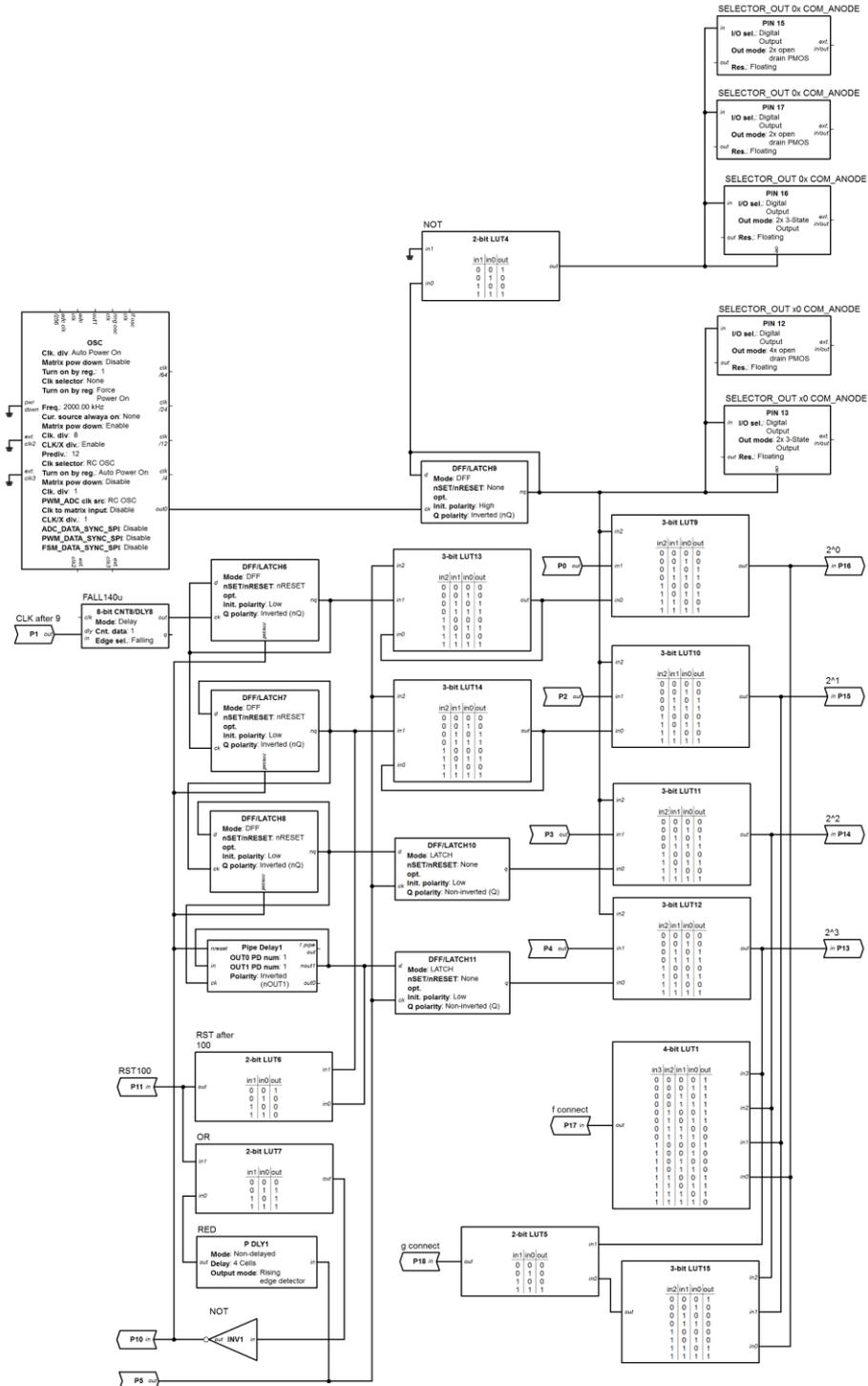
Block Diagram for Design. Matrix1 Part 3. Voltmeter architecture
