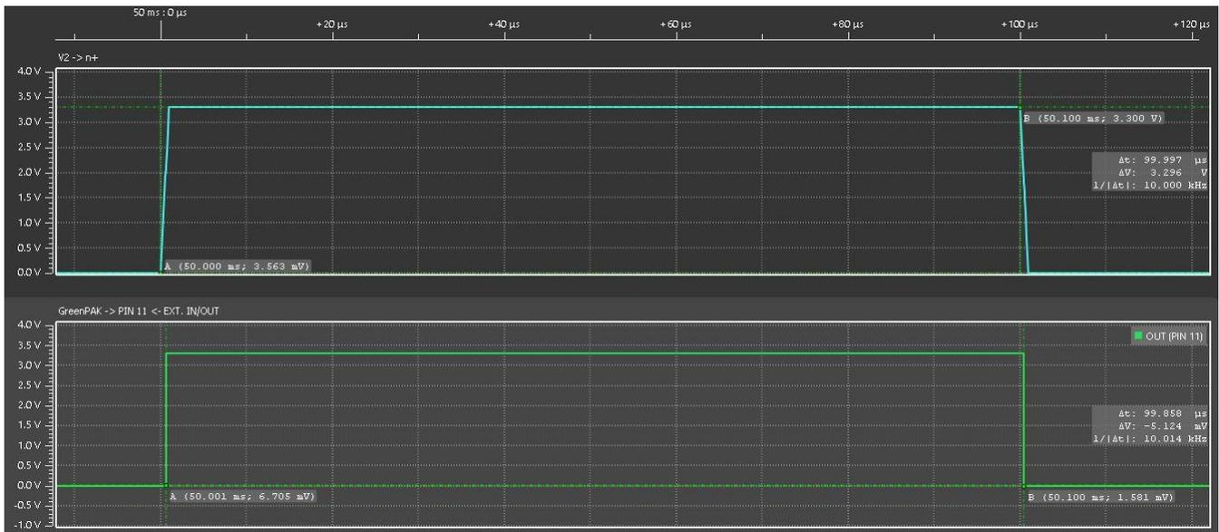
Figure 8. Pulse width is too short simulation case - Input signal is on top and, output signal is on bottom
