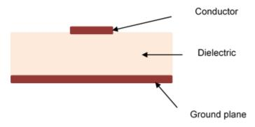
Microstrip is a planar transmission line, consisting of a conducting layer and a ground plane separated by dielectric. As there is no dielectric above the conducting layer, this structure is usually used at the top or bottom of the PCB.
