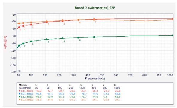
While there are some variations in the reflection coefficients when comparing Board 1 and Board 2, these variations are not significant enough to have a notable effect on the transmission coefficients.
