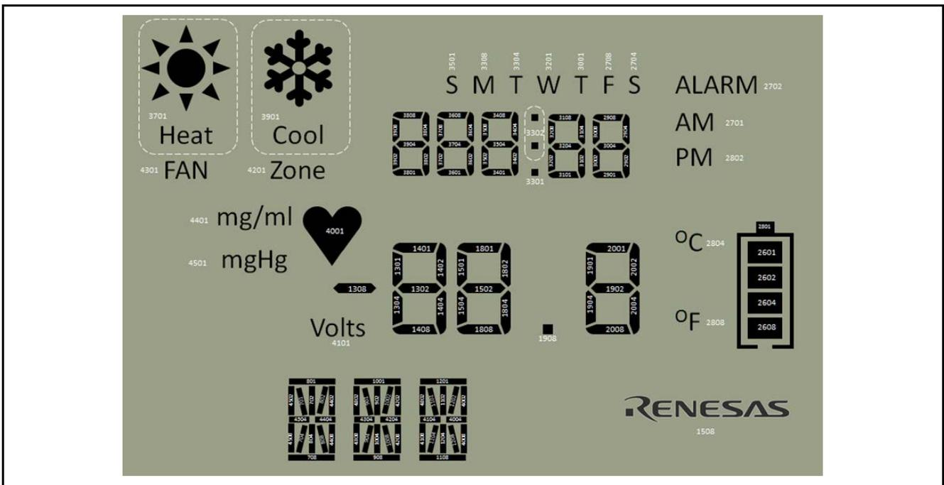
Figure 4. Segment LCD panel – segment numbering
