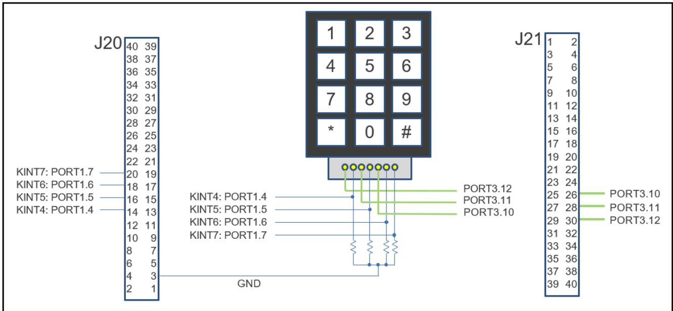
**Figure 4. Connecting the Keypad to the SK-S7G2 board**
