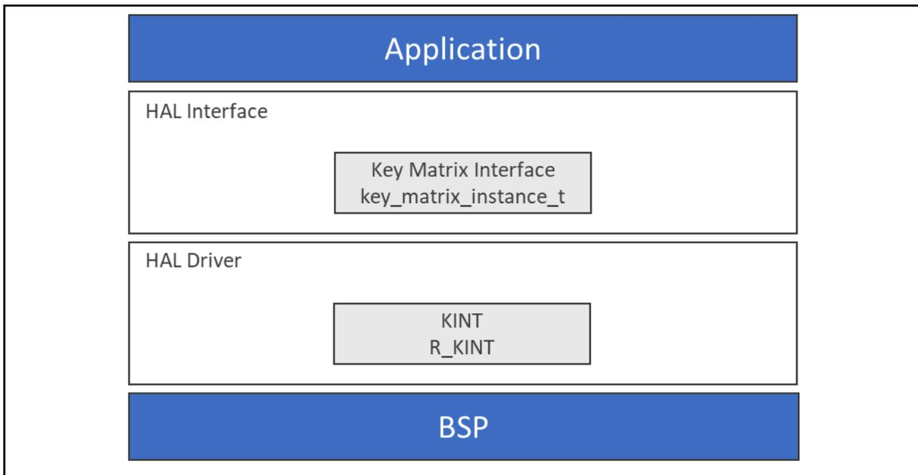
Figure 1. Key Matrix HAL Module Block Diagram
