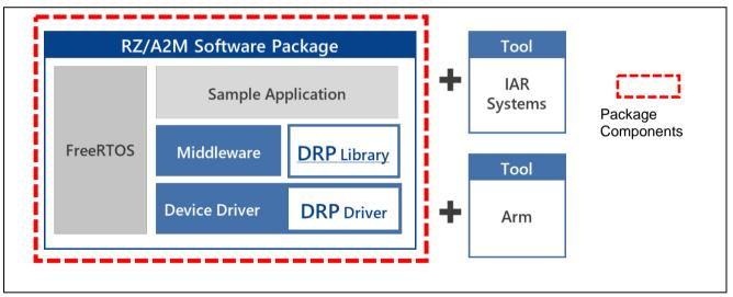
Figure 1. Multi-compiler development environment for the RZ/A2M Software Package
