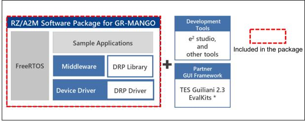
Figure 1 Components of the RZ/A2M Software Package for GR-MANGO
