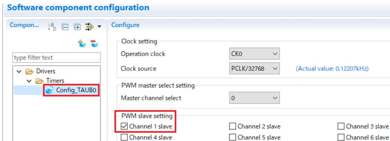
The following code is generated in the void R\_Config\_TAUB0\_Create(void) function of Config\_TAUB0.c, setting an incorrect value (red) to the TAUB0.TOM register.
