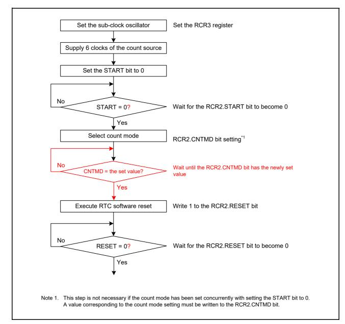
Figure 21.3 Clock and Count Mode Setting Procedure
