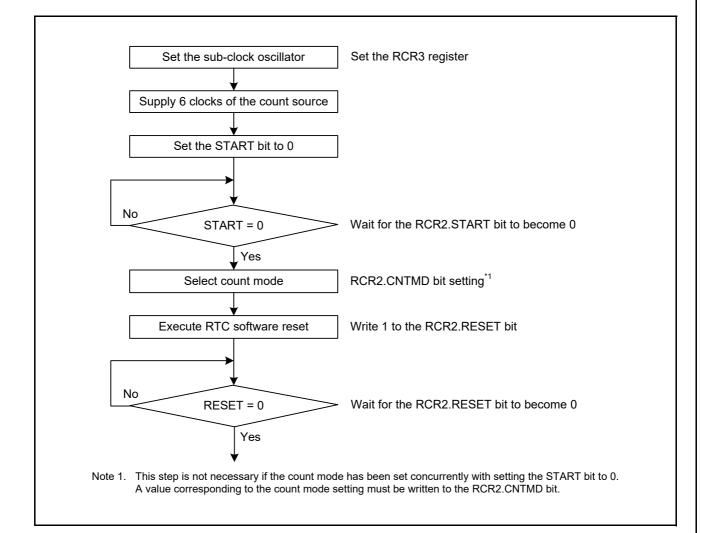
Figure 21.3 Clock and Count Mode Setting Procedure
