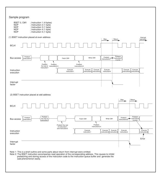
Figure 1. Program example and operation timing of the behavior described in "1. Usage precaution."
