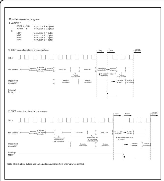
Figure 2. Countermeasure program example and operation timing (Example 1)
