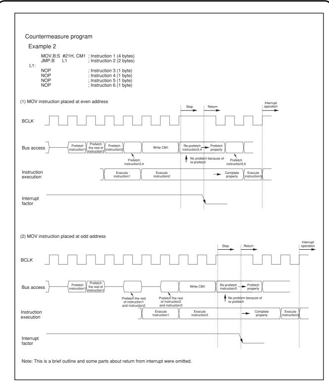
Figure 3. Countermeasure program example and operation timing (Example 2)
