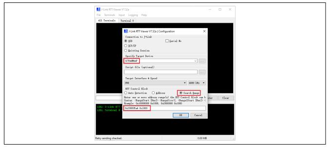
The first address of "Search Range" can be found in "\*.map" file after the demo code is built. Please open "\*.map" file and search "\_SEGGER\_RTT", then copy the address assigned by compiler to this place.
