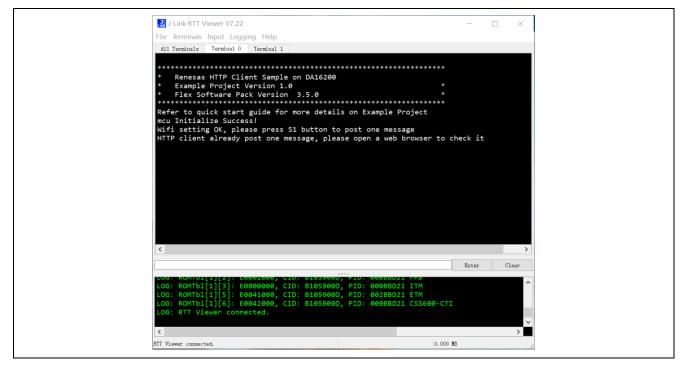
After Wi-Fi setting is completed, press S1 on EK-RA6M4 to post a message of "This is stream data from DA16200 Wi-Fi module / number is xx" to the HTTP server. POST command message can be found in the command prompt window for HTTP server as below.
