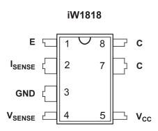
Figure 4.1: 7-Lead PDIP Package
