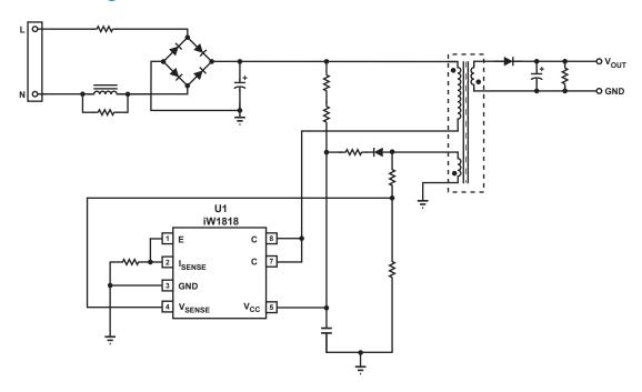
Figure 3.1: iW1818 Typical Application Circuit
