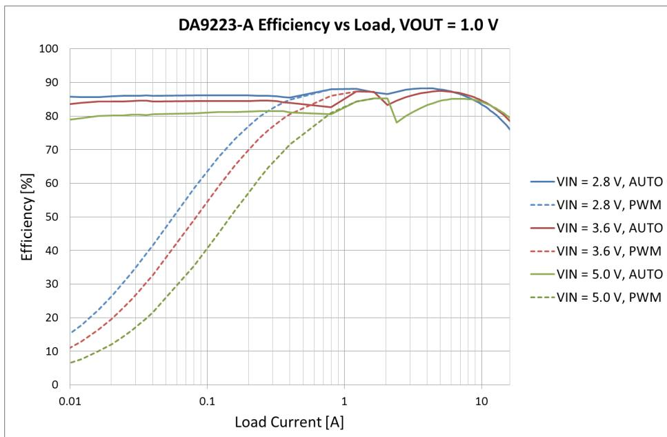
Efficiency Diagram DA9223-A, measured using 2520 size
