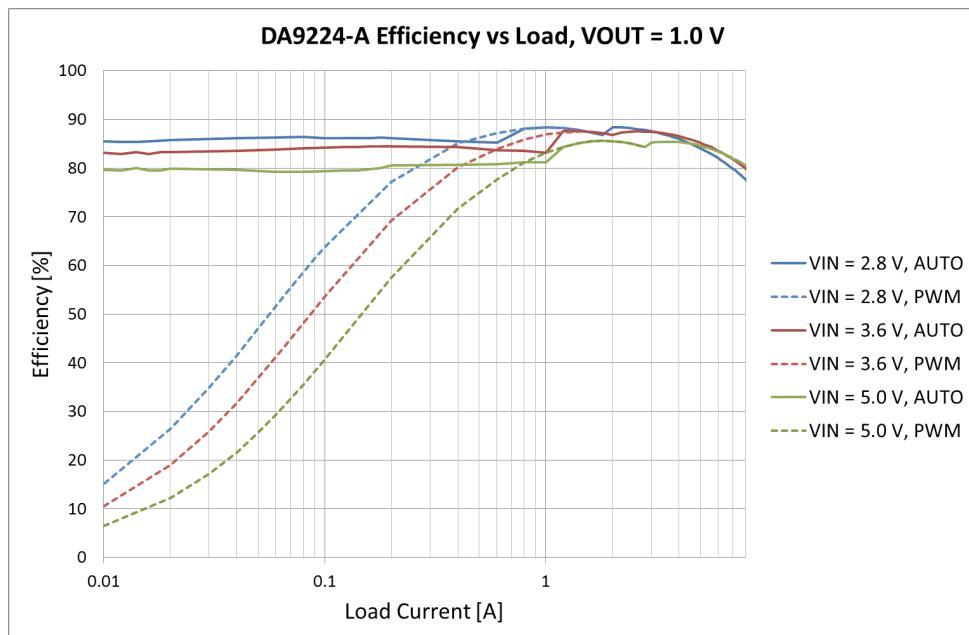
Efficiency Diagram DA9224-A, measured using 2520 size
