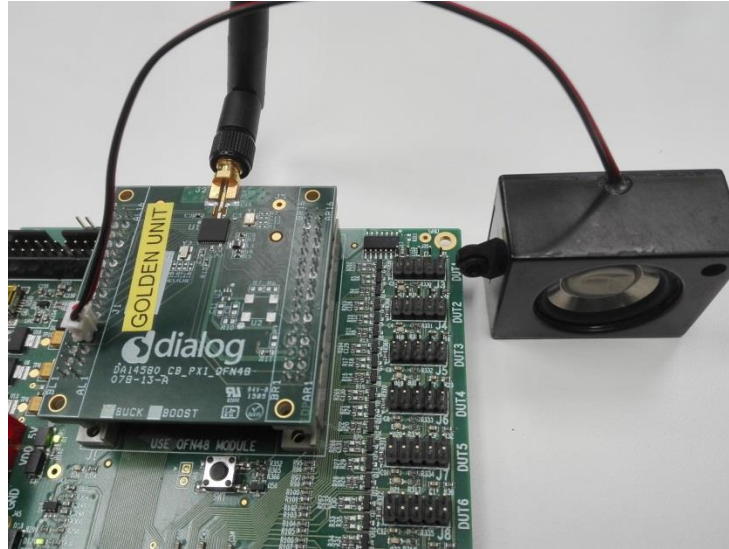
Figure 169: Speaker Connection for Audio Test.
