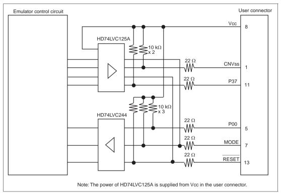
Figure 3.6 Interface Circuit in the Emulator (Reference)
