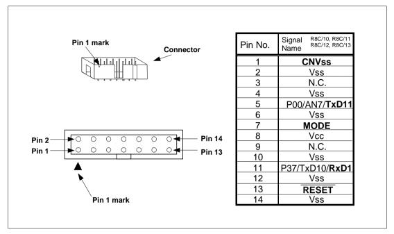
Figure 2.1 Pin Assignments of the E7 Connector
