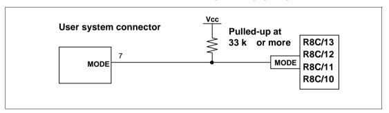
Figure 3.3 Connection of E7 Emulator and MODE Pin
