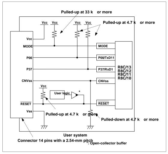
Figure 3.1 Example of E7 Connection
