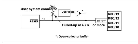
Figure 3.5 Example of a Reset Circuit
