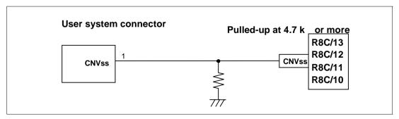
Figure 3.4 Connection of E7 Emulator and CNVss Pin
