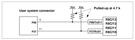
Figure 3.2 Connection of E7 Emulator and MCU
