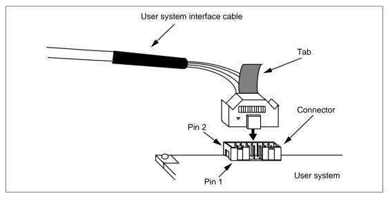
Figure 1.1 Connecting the User System Interface Cable to the User System
