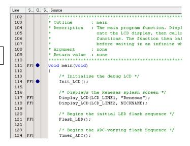
It is also possible to set breakpoints by selecting the line to stop at and pressing the [F9] key.
