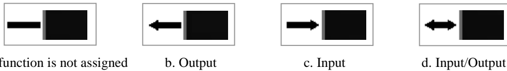
Figure 3.22 Display of input/output direction
