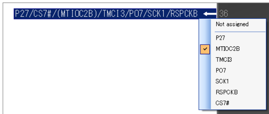
Figure 3.20 Pin function selection
