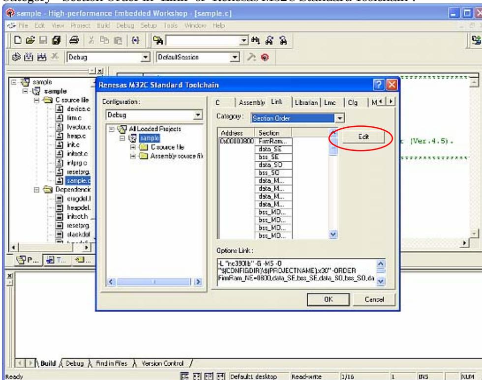
If you added a new section with `#pragma SECTION`, click the [Edit] button in (1) to open the Section window.
