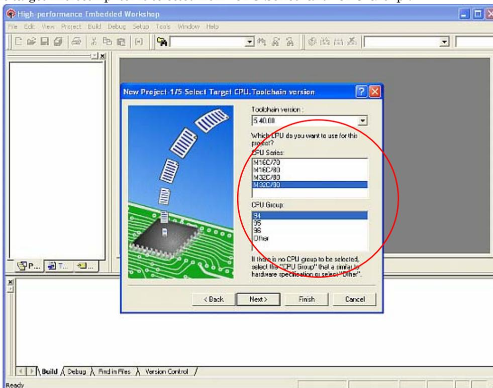
When a type of microcomputer is selected, its corresponding sfr header file is copied to the workspace. Furthermore, a variable vector table (intprg.c) is registered.
