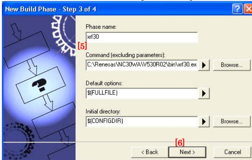
[5] Type xrf30 and its fullpath name in the Phase Name and the Command text box.
