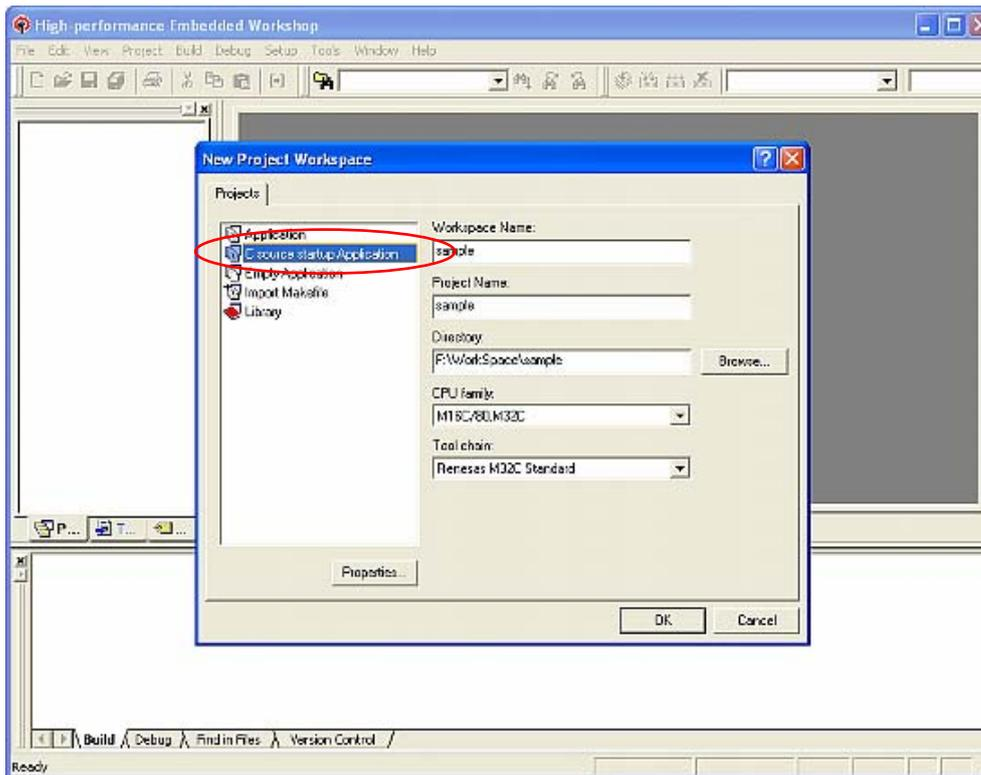
If while multiple compilers are installed in your computer you select another microcomputer for the CPU type after selecting C source startup Application, the focus for C source startup Application will move to Application, with the result that the selected C source startup has no effect. In such a case, therefore, select "C source startup Application" again.
