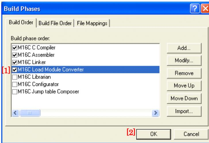
[1] Select the Mxxx Load Module Converter check box from the Order of Build Phases list.
