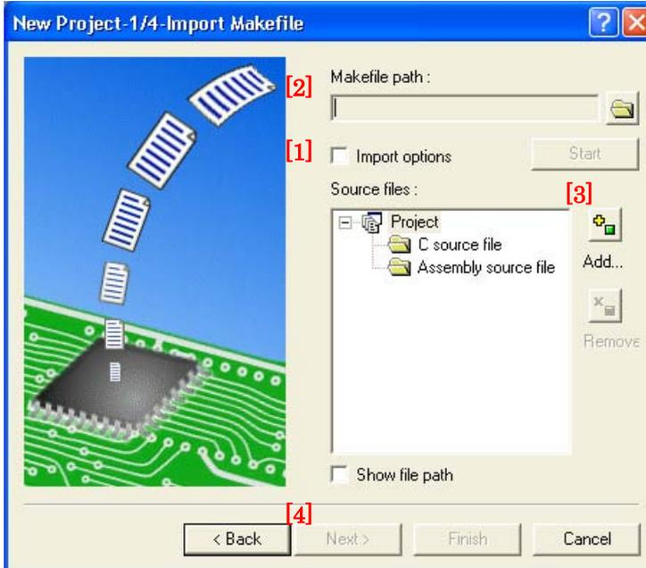
[1] Select the Import options check box; this will enable information on build options (compiling and assembling options etc.) to be used to create High-performance Embedded Workshop projects. If you clear the Import options check box, the above information is neglected and not used in High-performance Embedded Workshop.
