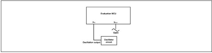
Figure 2.21 External oscillator circuit
