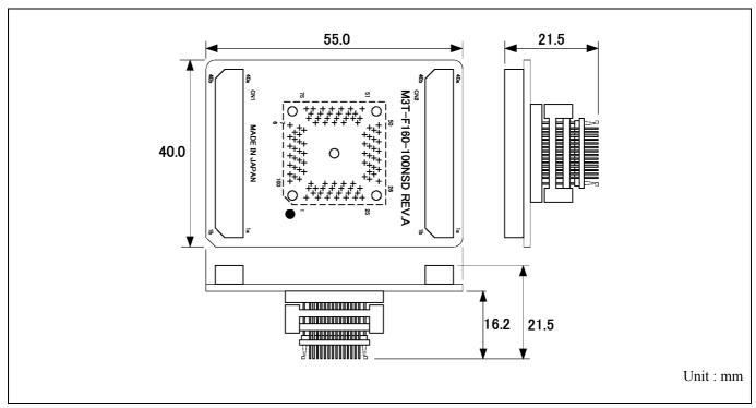
Figure 4.5 External dimensions of the M3T-F160-100NSD
