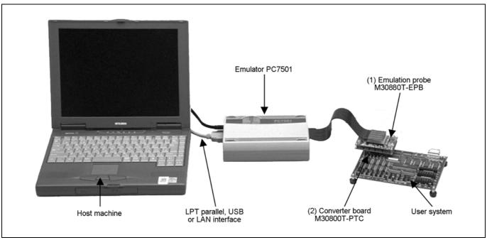
Figure 1.1 System configuration
