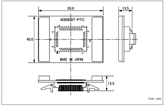
Figure 4.4 External dimensions of the M30800T-PTC
