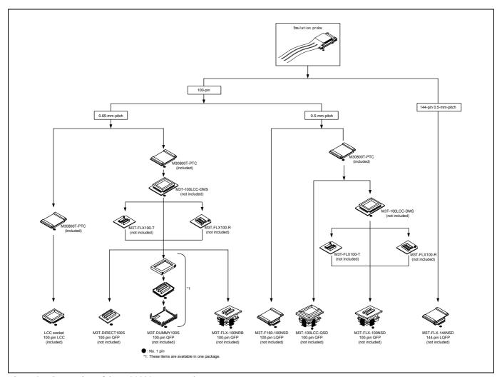
Figure 2.7 Connection of the M30880T-EPB and user system
