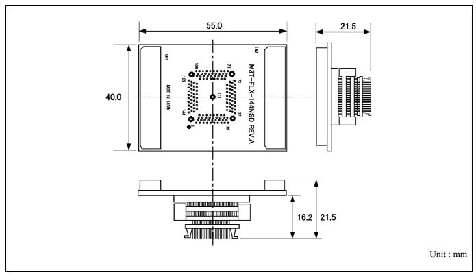
Figure 4.6 External dimensions of the M3T-FLX-144NSD
