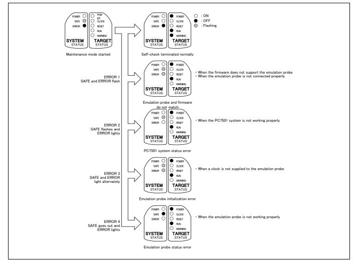
Figure 2.6 Self-check procedure
