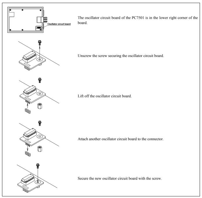
Figure 2.18 Replacing oscillator circuit boards
