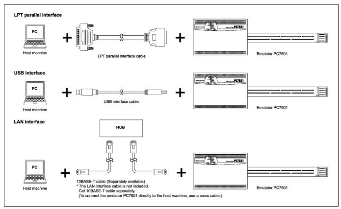
Figure 2.2 Outline for interface cable connections
