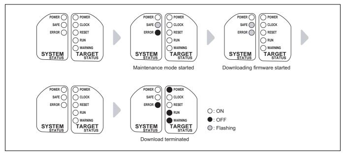
Figure 2.5 Downloading firmware in maintenance mode
