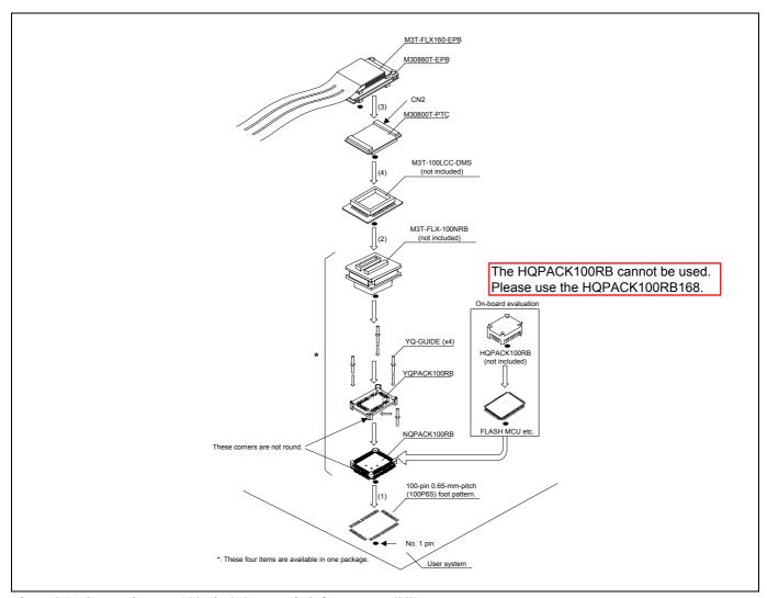
Figure 2.11 Connecting to a 100-pin 0.65-mm-pitch foot pattern (3/3)
