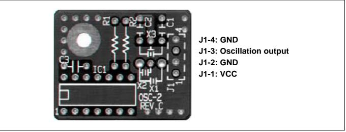
Figure 2.19 External view of the oscillator board OSC-2 (bare board) and connector pin assignments
