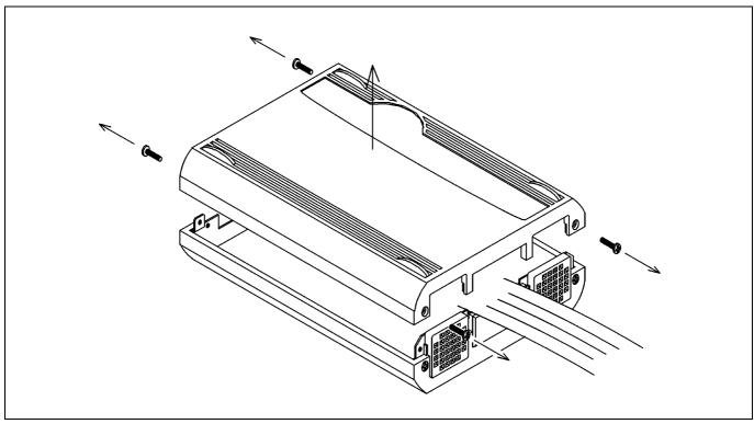
Figure 2.17 Removing the upper cover
