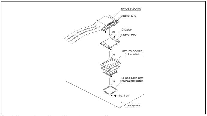
Figure 2.12 Connecting to a 100-pin 0.5-mm-pitch foot pattern (1/3)
