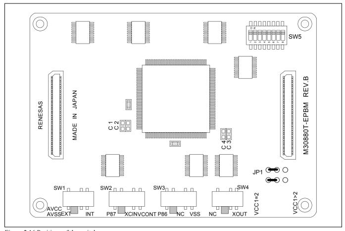
Figure 2.16 Positions of the switches
