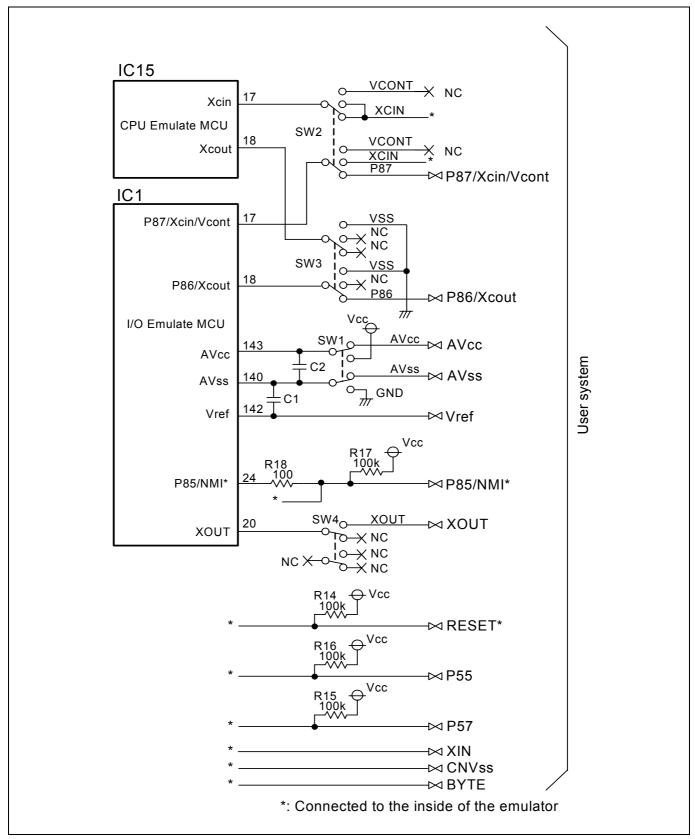
Figure 4.1 Connection diagram (1/2)
