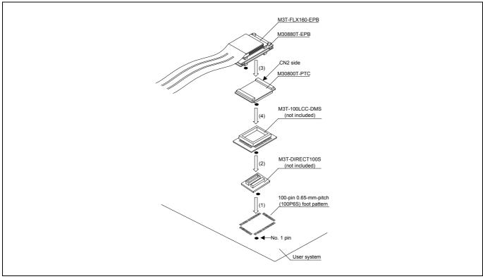
Figure 2.10 Connecting to a 100-pin 0.65-mm-pitch foot pattern (2/3)
