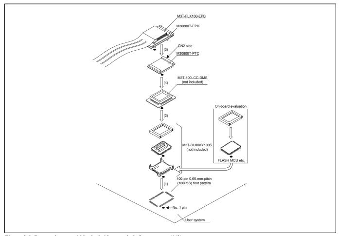
Figure 2.9 Connecting to a 100-pin 0.65-mm-pitch foot pattern (1/3)
