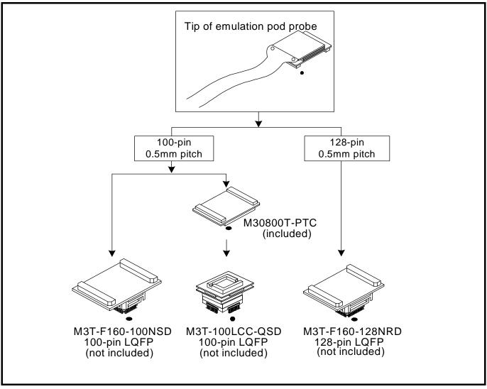
Figure 2.9 Connecting the user system (for M16C/6NK, M16C/6NL, M16C/6NM and M16C/6NN)
