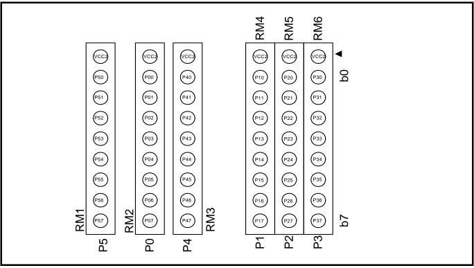
Figure 2.24 Position for mounting network resistors for pullup
