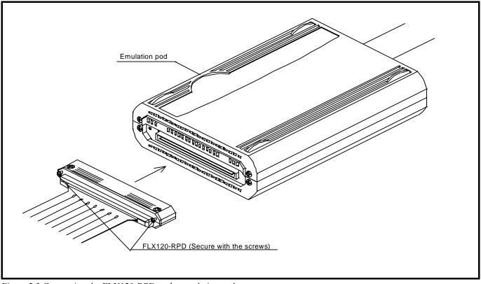
Figure 2.3 Connecting the FLX120-RPD to the emulation pod
