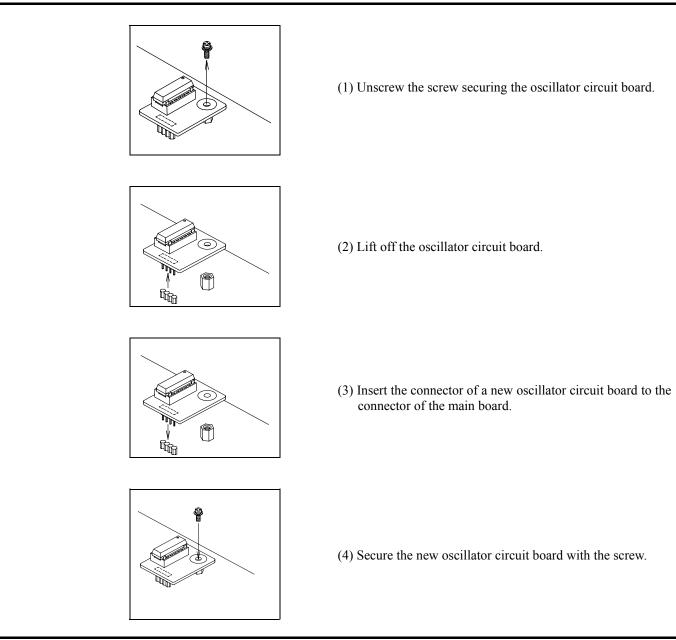
Figure 2.19 Replacing oscillator circuit boards
