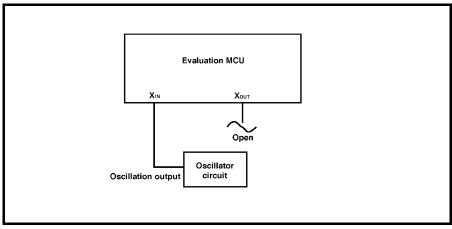
Figure 2.22 External oscillator circuit
