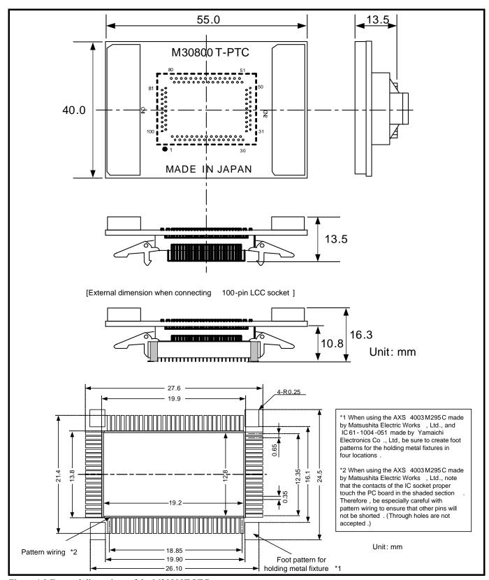
Figure 4.9 External dimensions of the M30800T-PTC
