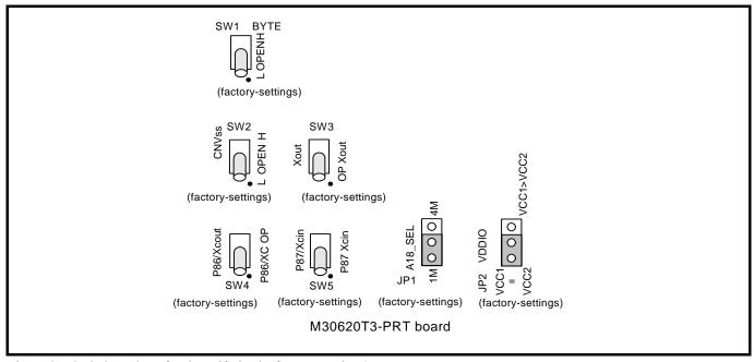
Figure 2.7 Switch settings for the self-check (factory-settings)
