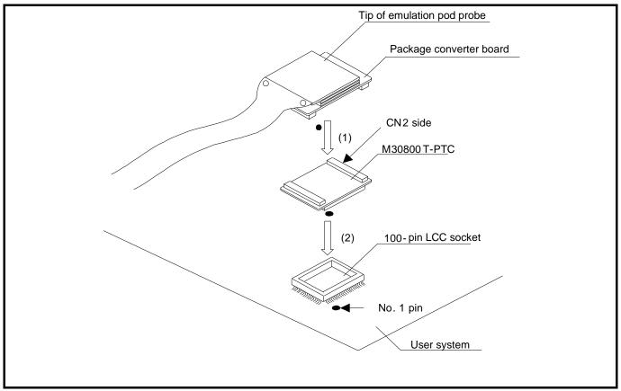
Figure 2.10 Connecting to a 100-pin LCC socket
