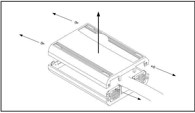
Figure 2.17 Removing the upper cover
