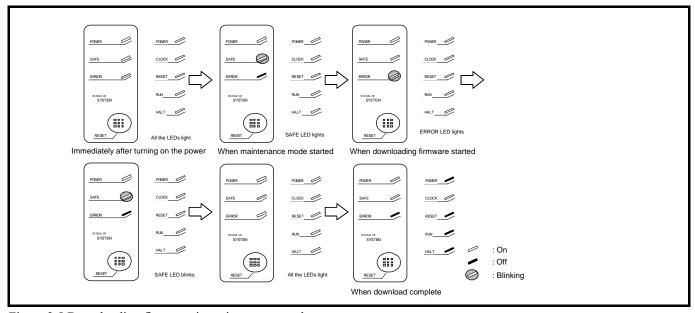
Figure 2.5 Downloading firmware in maintenance mode
