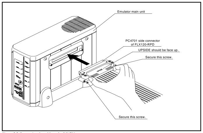
Figure 2.2 Connecting the cable to the PC4701
