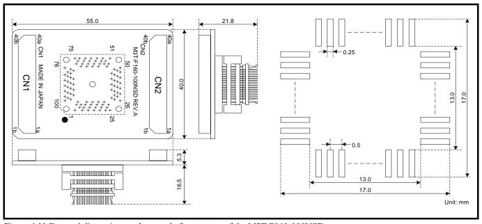
Figure 4.11 External dimensions and a sample foot pattern of the M3T-F160-100NSD
