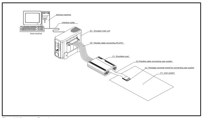
Figure 1.1 System configuration
