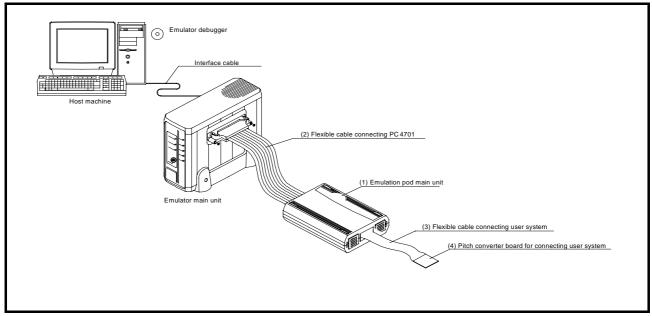
Figure 1.1 System configuration
