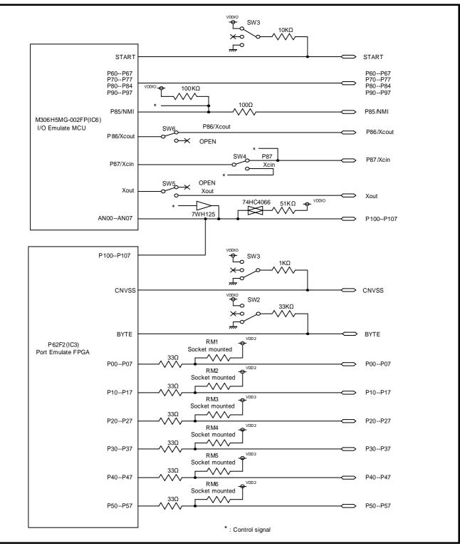
Figure 4.4 Connection diagram
