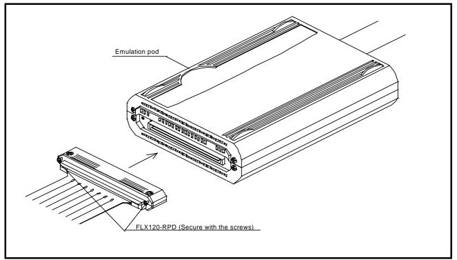
Figure 2.13 Connecting the cable to the emulation pod
