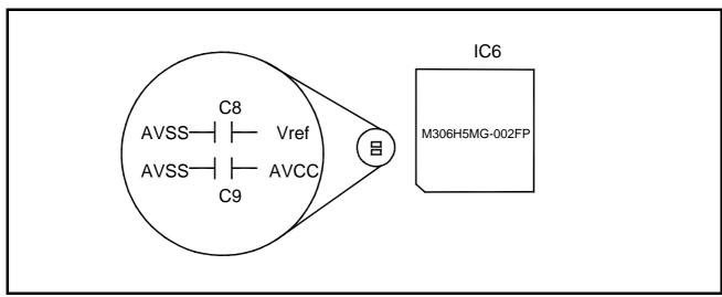
Figure 2.9 Foot patterns of bypass capacitors for A/D converter
