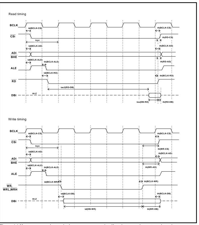
Figure 4.1 Memory expansion and microprocessor modes (3-wait, accessing external area)
