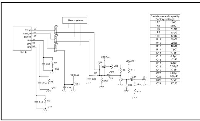
Figure 2.10 Connection diagram of circuits connected to the data slicer
