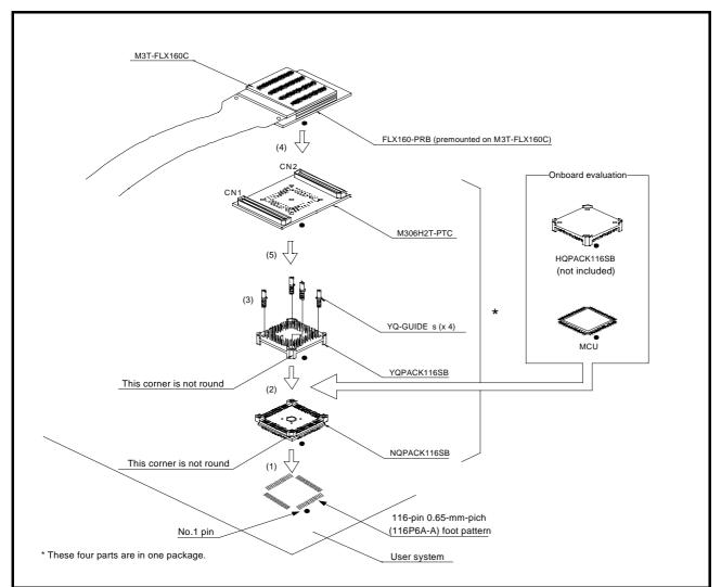
Figure 2.14 Connecting the user system
