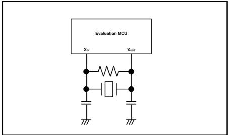
Figure 2.7 Circuit in which oscillation does not occur (same for  $X_{CIN}$ - $X_{COUT}$ )
