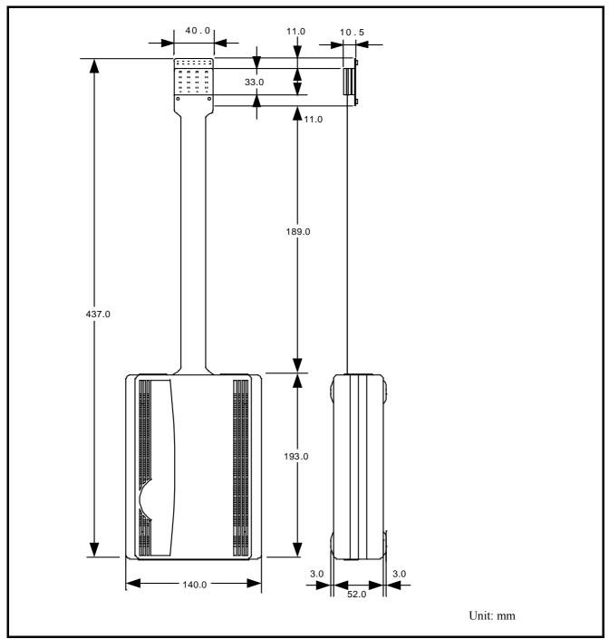
Figure 4.5 External dimensions of the emulation pod
