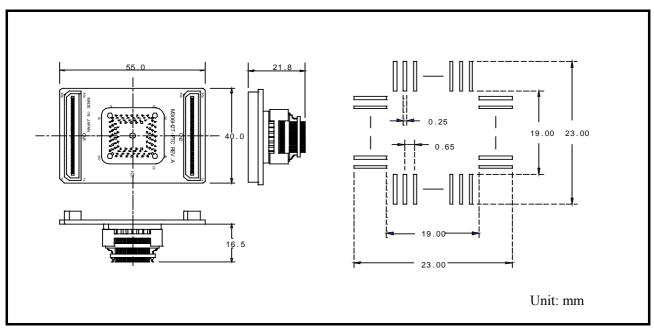
Figure 4.6 External dimensions of the converter board M306H2T-PTC and a sample foot pattern for the NQPACK116SB
