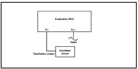
Figure 2.6 External oscillator circuit
