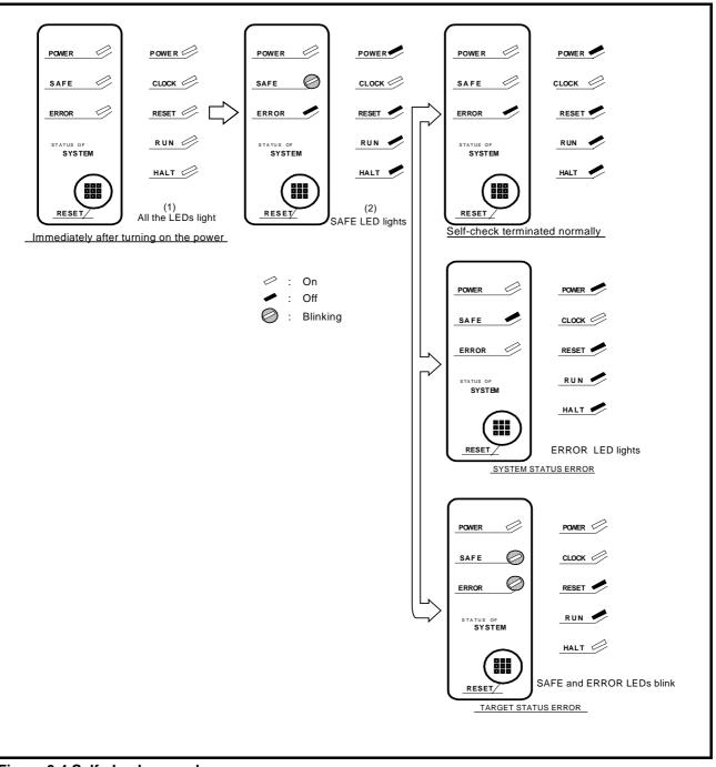
Figure 3.4 Self-check procedure
