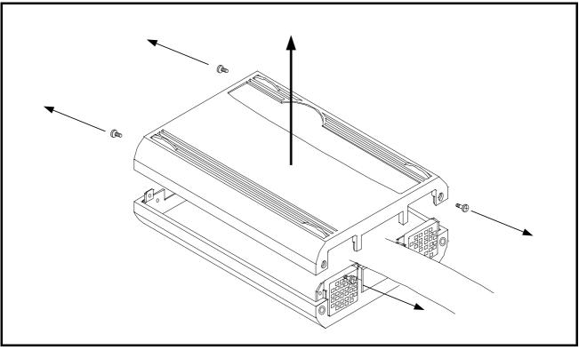
Figure 2.1 Removing the upper cover
