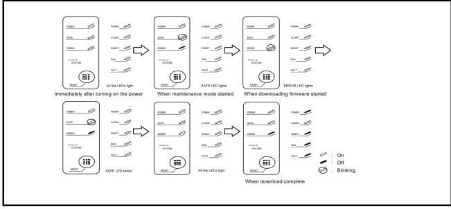
Figure 3.2 Downloading firmware in maintenance mode
