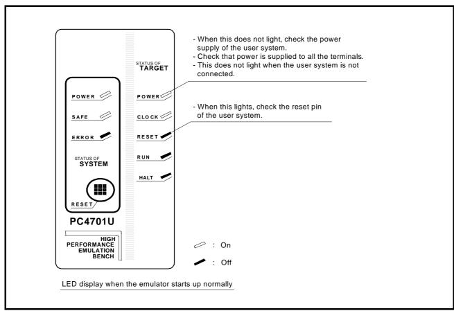
Figure 3.1 LED display when the power turned on
