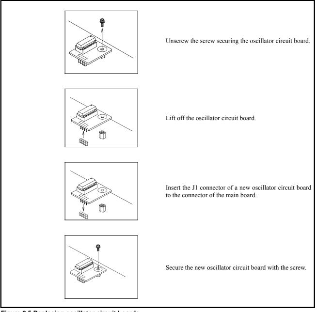
Figure 2.5 Replacing oscillator circuit boards
