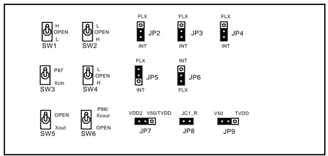
Figure 3.3 Switch settings for the self-check (factory-settings)
