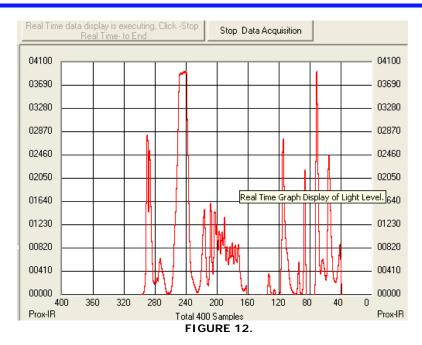
**Collect Data Graphical Real Time Data -** Allows you to sample data (whether ALScont, IRcont, or Proxcont). Samples are now being taken and are being plotted, and appropriate values are displayed on the right in the corresponding box.
