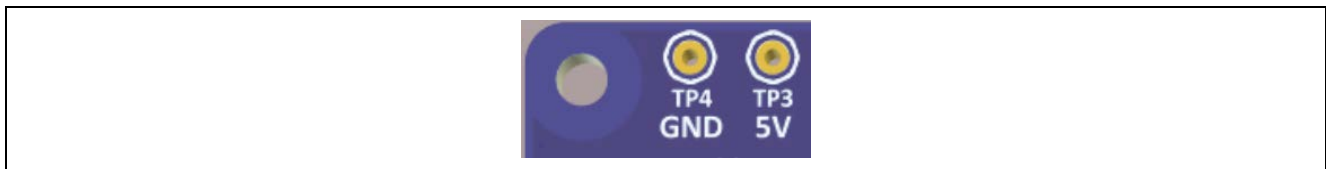
Figure 7. TP3 and TP4 on the Evaluation Kit Board
