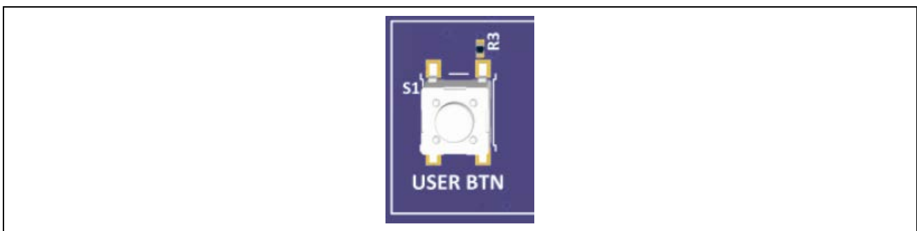
Figure 18. User Switch (S1) on the Evaluation Kit Board
