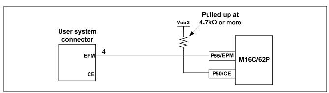
Figure 5.8 Connection of E8a Emulator and Pins P50 and P55 (Dual Power Supply and Single-chip Mode)
