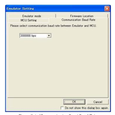
Figure 7.4 [Communication Baud Rate] Tab
