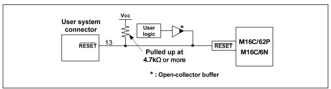
Figure 5.11 Example of a Reset Circuit
