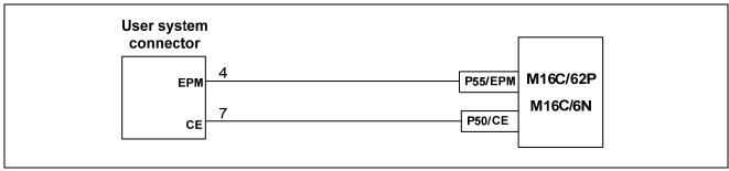
Figure 5.6 Connection of E8a Emulator and Pins P50 and P55 (Single Power Supply and Single-chip Mode)
