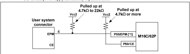
Figure 5.9 Connection of E8a Emulator and Pins P50 and P55 (Dual Power Supply and Memory Expansion Mode)
