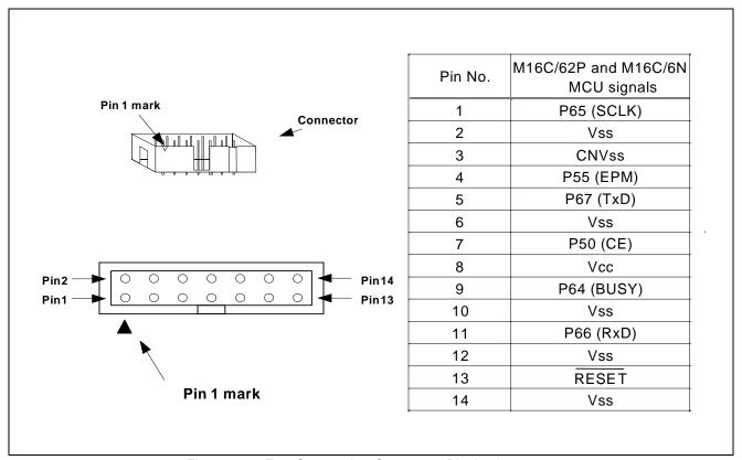
Figure 4.1 E8a Connecting Connector Pin Assignments
