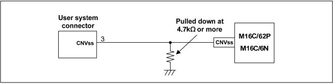
Figure 5.10 E8a Emulator and CNVss Pin Connection
