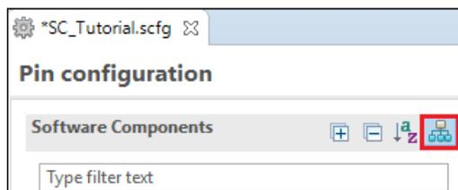
Figure 4-42 Change view to show by Software Components
