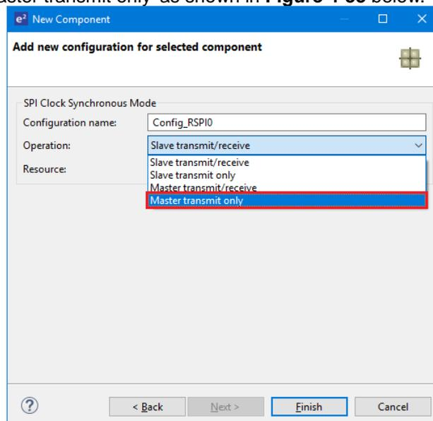
**Figure 4-33 Select Operation – Master transmit only**
