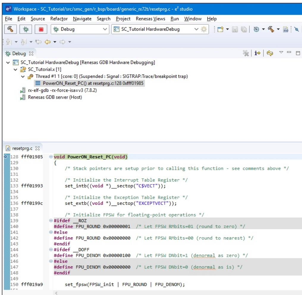
**Figure 6-5 Debugger start up screen**
