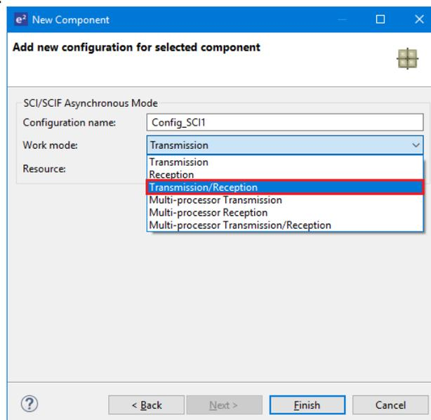
**Figure 4-28 Select Work mode – Transmission/Reception**
