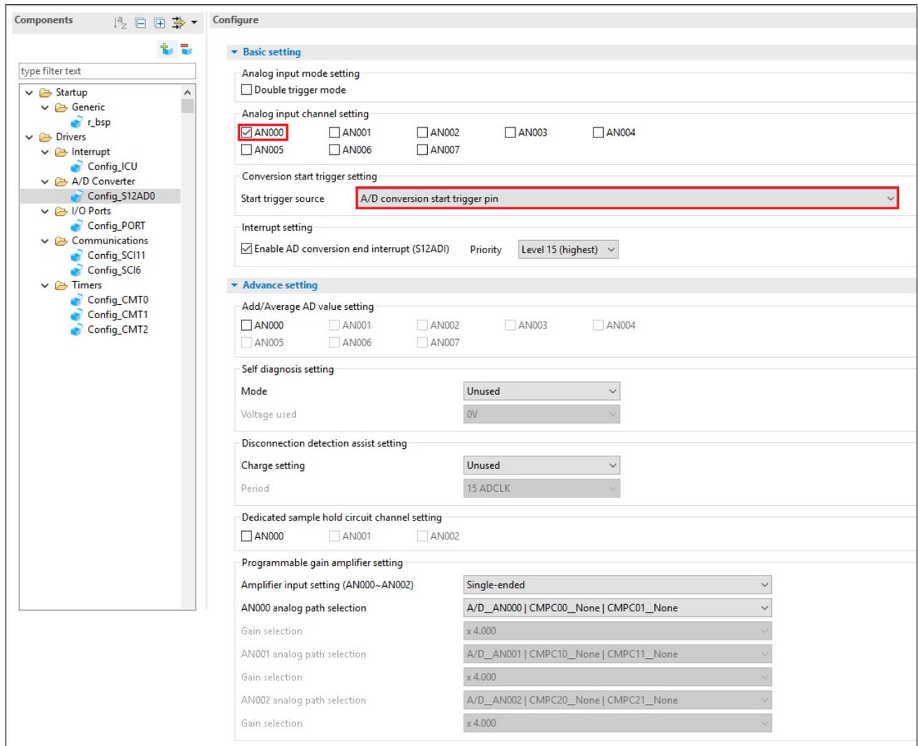
**Figure 4-39 Config\_S12AD0 setting (1)**
