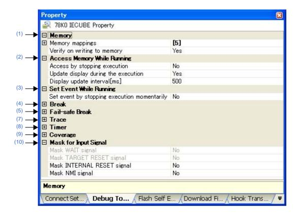
Figure A-10. Property Panel: [Debug Tool Settings] Tab [MINICUBE2][E1][E20][EZ Emulator]
