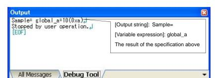
Figure 2-138. Example of Output Result of Printf Event
