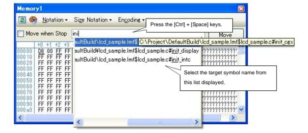
Figure 2-151. Symbol Name Completion Function
