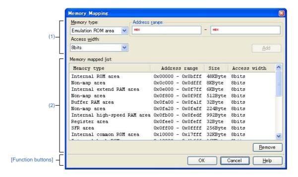
Figure A-33. Memory Mapping Dialog Box [Simulator]
