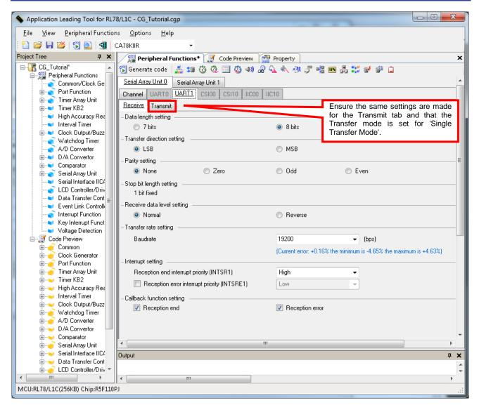
Figure 3-12 Serial Array Unit 0 tab - UART1 settings
