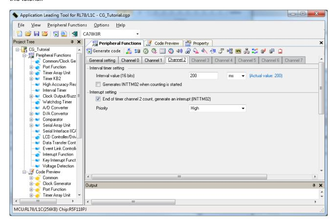
Figure 3-9 Timer Array Unit tab – Channel 2
