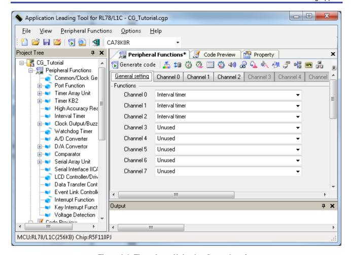
Figure 3-6 Timer Array Unit tab - General setting
