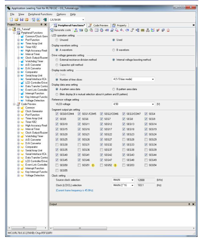
Figure 3-5 LCD Controller/Driver tab
