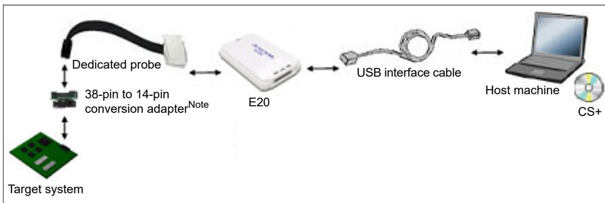
**Note** Use a 38-pin to 14-pin conversion adapter attached to the E20 emulator if you have selected FINE [E20 (Serial)] as the method of communication with the target system.
