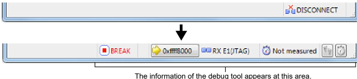
**Remark** When the button on the **Debug toolbar** is clicked, it will download the specified file after connecting to the debug tool (see "2.5.1 Execute downloading").
