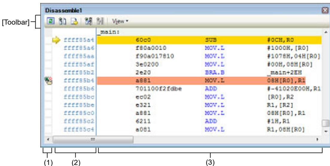
Figure A.8 Disassemble Panel (When Code Coverage Measurement Result is Displayed) [Simulator][E20 [RX71M, RX66x, RX65x, RX64M, RX66T, RX671, RX72T, RX72M, and RX72N]
