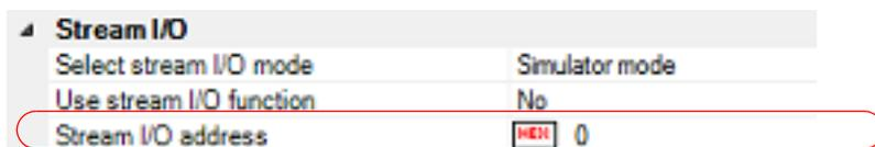
Upon detecting "Branch to subroutine" instruction (BSR, JSR) to a specified address while executing instructions of the program, the simulator performs an I/O process using the contents of the R1 and R2 registers as parameters.
