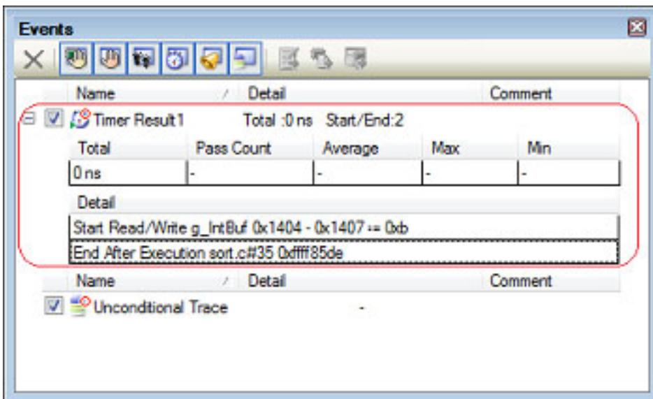
Figure 2.164 Example of a Measurement Result by Timer Measurement Event (Timer Start and End Events) [Simulator]
