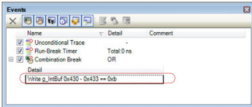
Figure 2.112 Example of Setting a Break Event (Access-related) on a Variable in the Source Text [Simulator]
