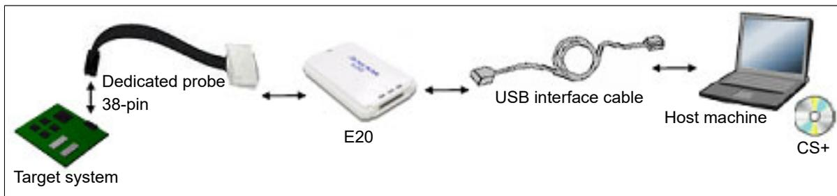
Figure 2.3 Connection Example [E20(Serial)]
