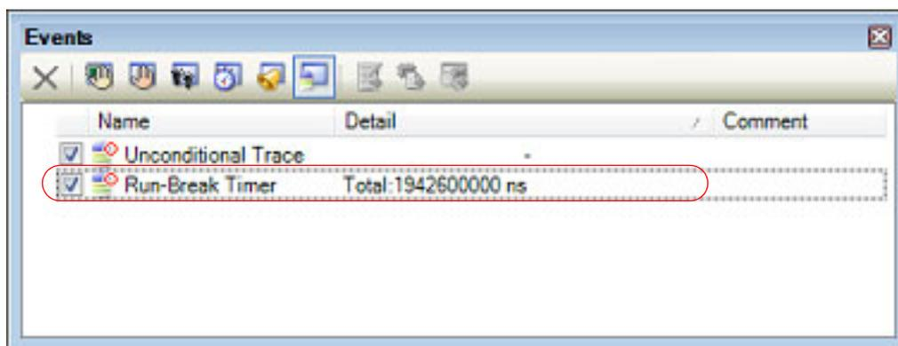
Figure 2.156 Example of a Run-Break Timer Event Measurement Result (Events Panel) [Simulator]
