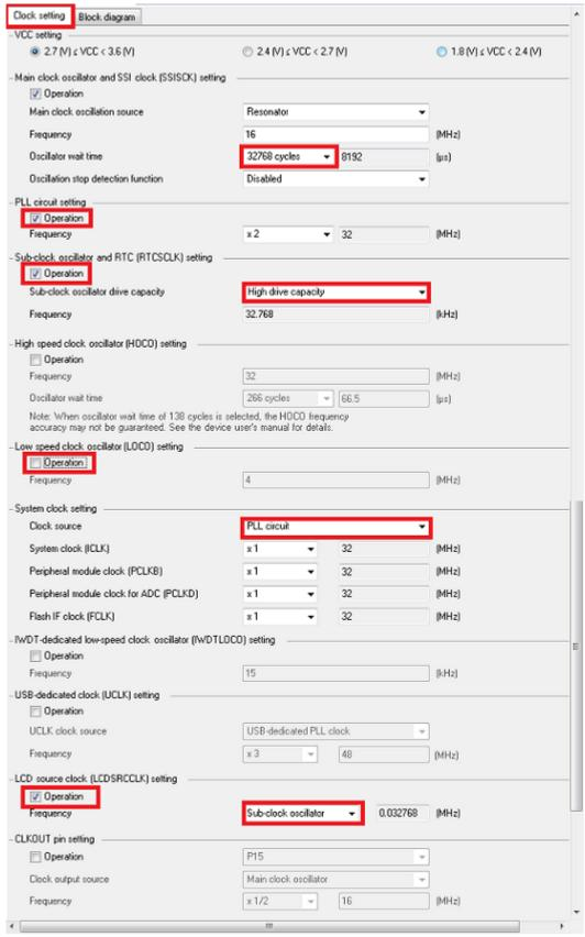
Figure 4-2 Clock setting tab
