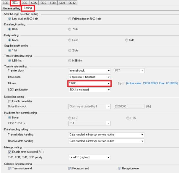
Figure 4-7 SCI1 Setting tab
