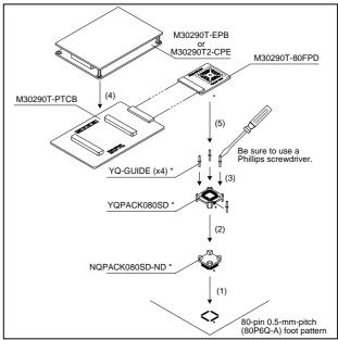
Figure 3 Connection procedure of the M30290T-80FPD
