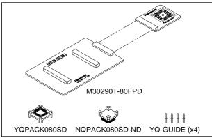
Figure 1 Package components of the M30290T-80FPD
