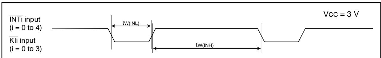
**Figure 35.17 Input Timing Diagram for External Interrupt  $\overline{\text{INT}}_i$  and Key Input Interrupt  $\overline{\text{K}}_i$  when Vcc = 3 V**
