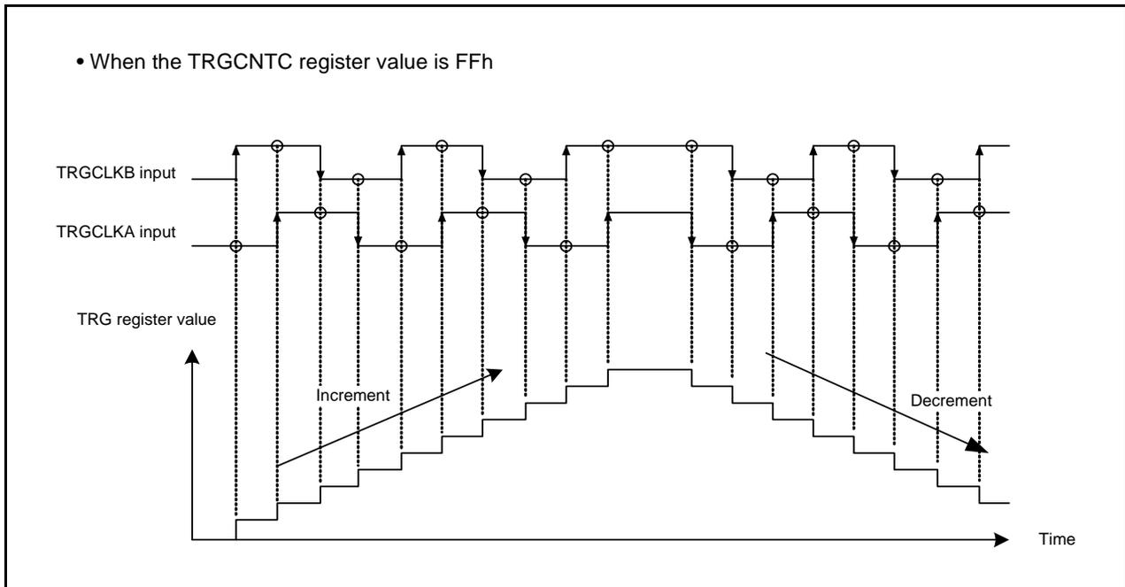
Figure 23.17 Operating Example 1 in Phase Counting Mode
