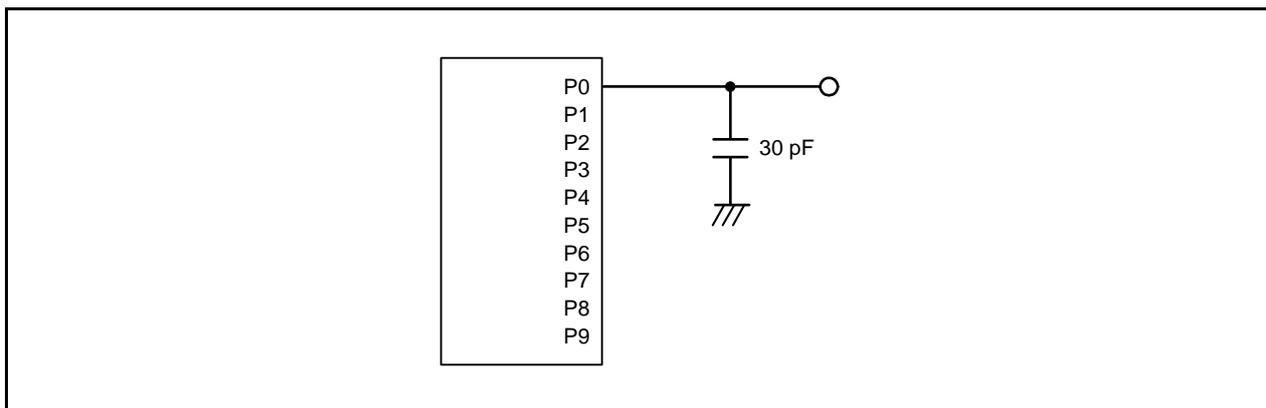
Figure 35.1 Ports P0 to P9 Timing Measurement Circuit
