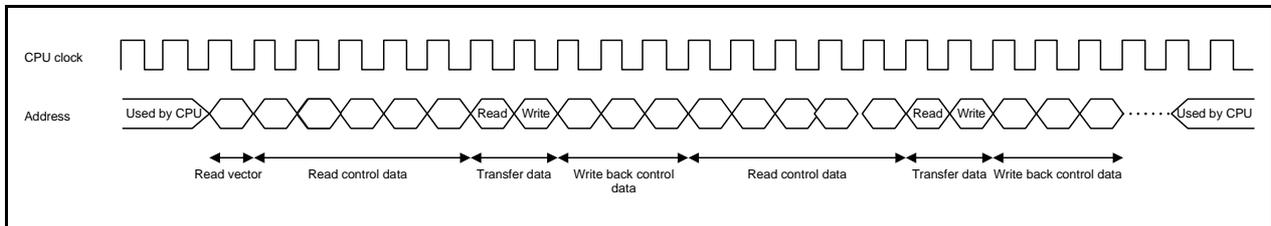
Figure 15.12 Example of DTC Operation Timings in Chain Transfers
