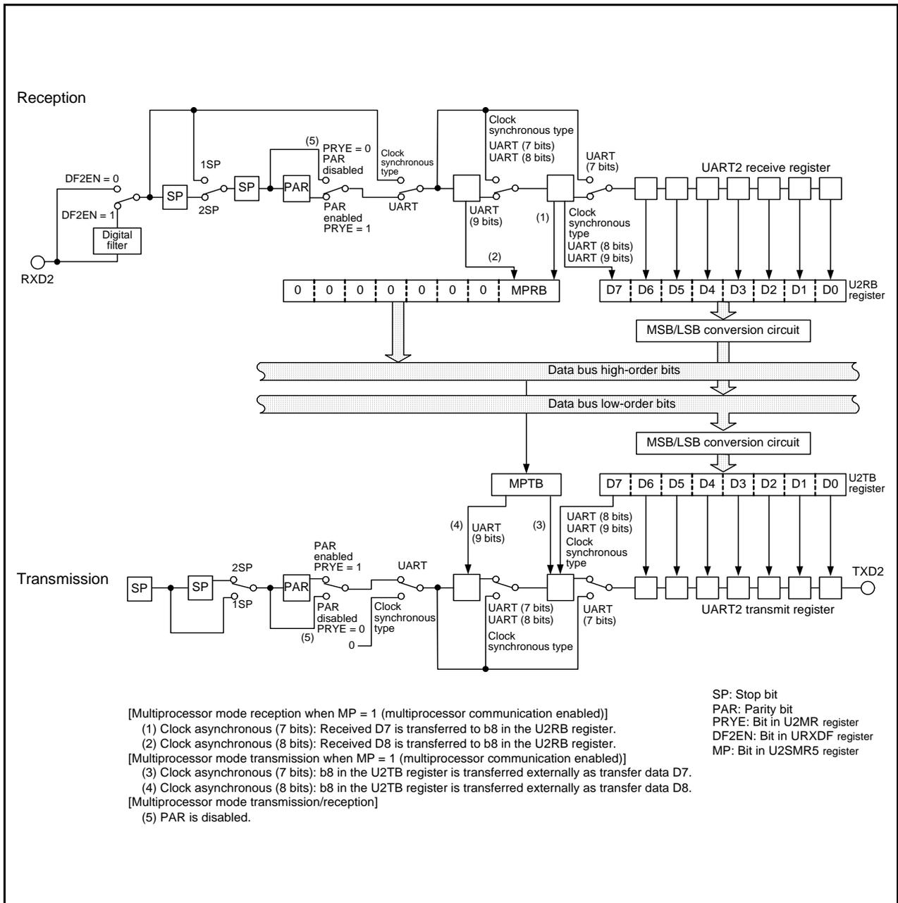
Figure 25.18 Block Diagram of Multiprocessor Communication Function
