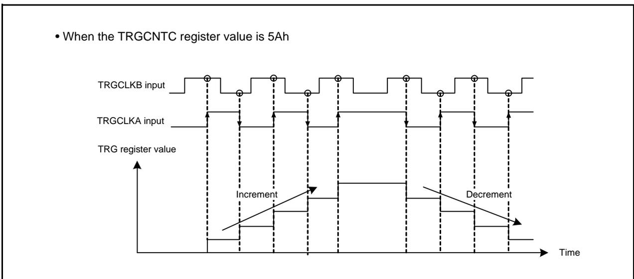
Figure 23.20 Operating Example 4 in Phase Counting Mode
