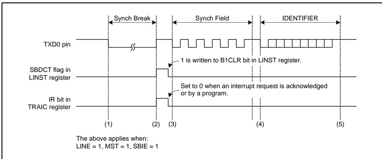
**Figure 29.2 Operating Example during Header Field Transmission**
