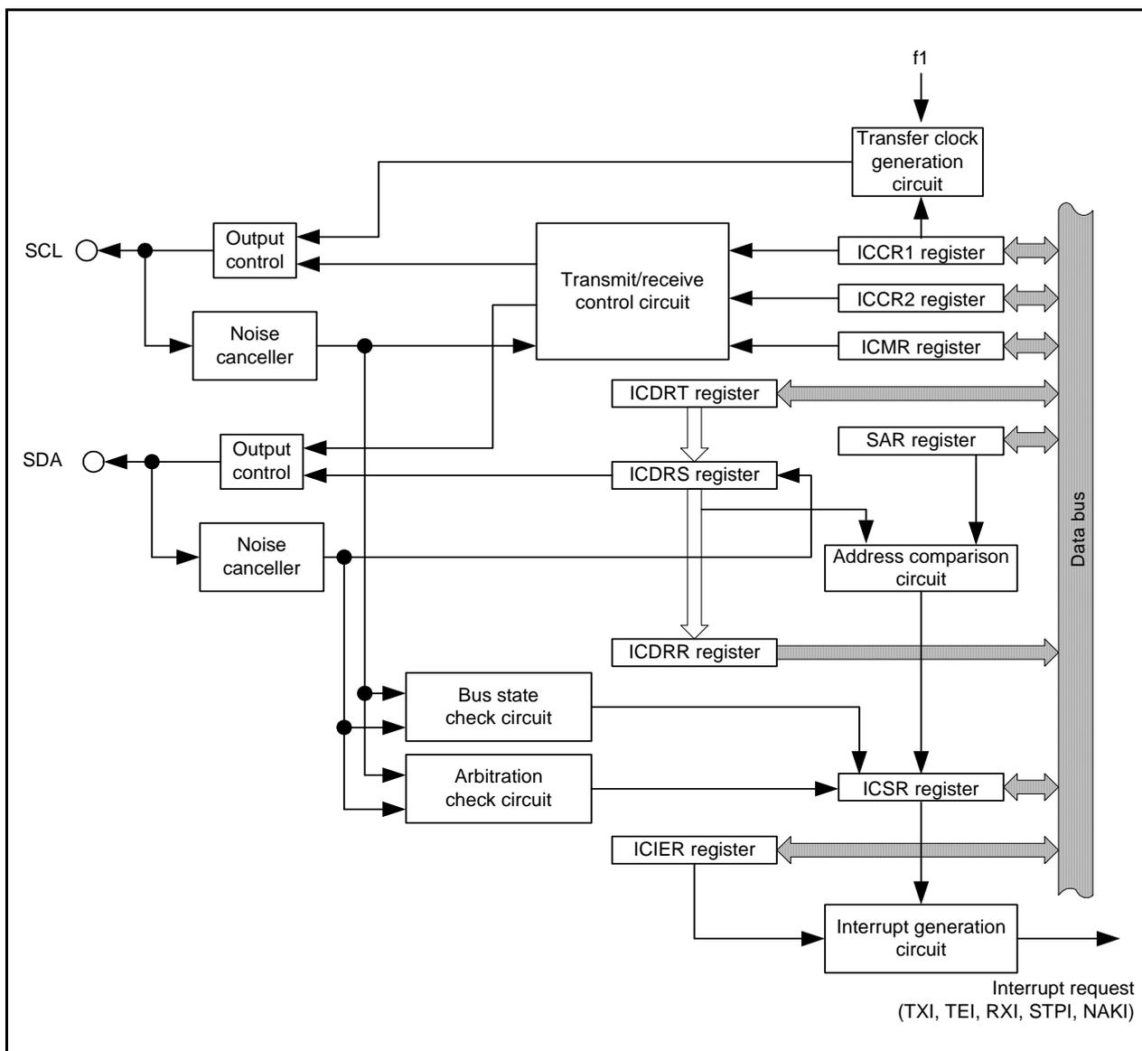
Figure 28.1 I<sup>2</sup>C bus interface Block Diagram
