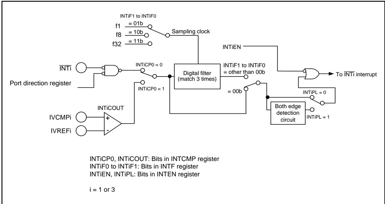
Figure 32.3 Configuration of Comparator Bi Digital Filter
