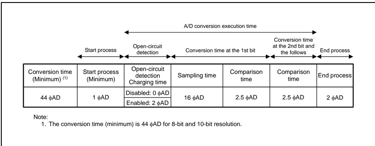
Figure 30.3 A/D Conversion Cycles ( $\phi_{AD} = f_{AD}$ )
