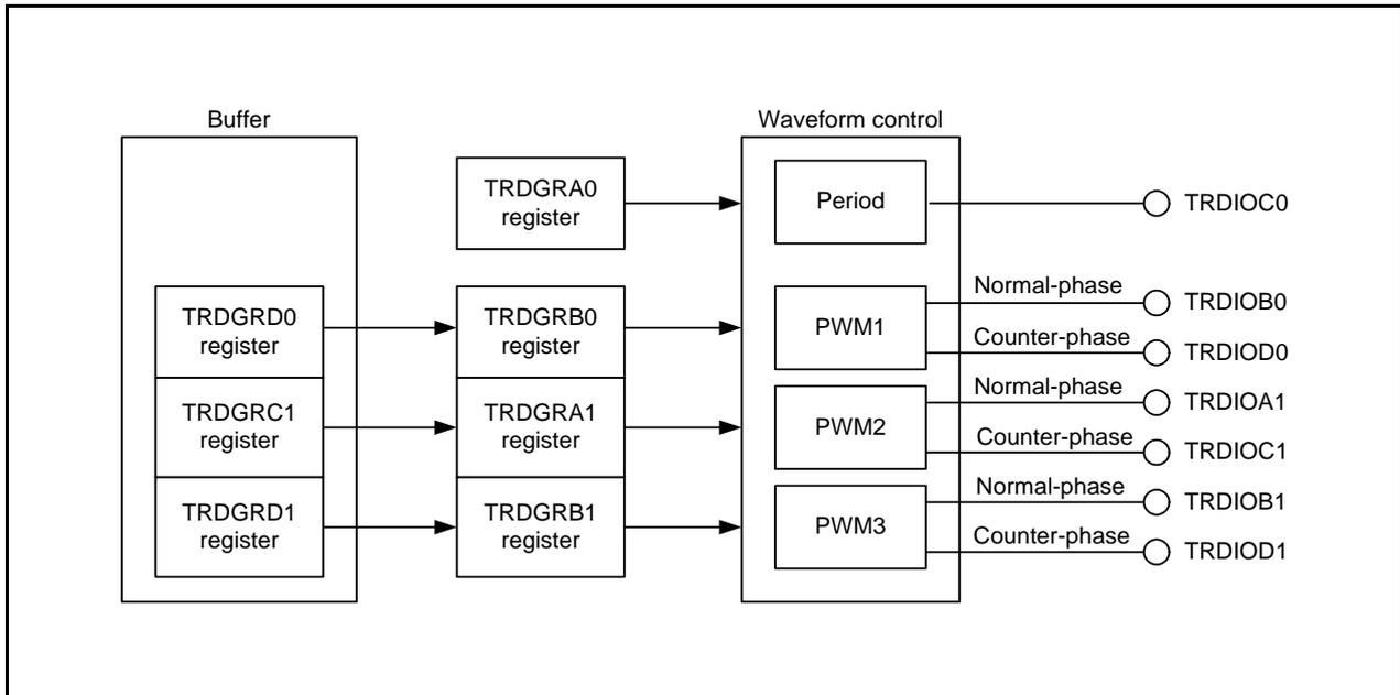
Figure 20.19 Block Diagram of Complementary PWM Mode
