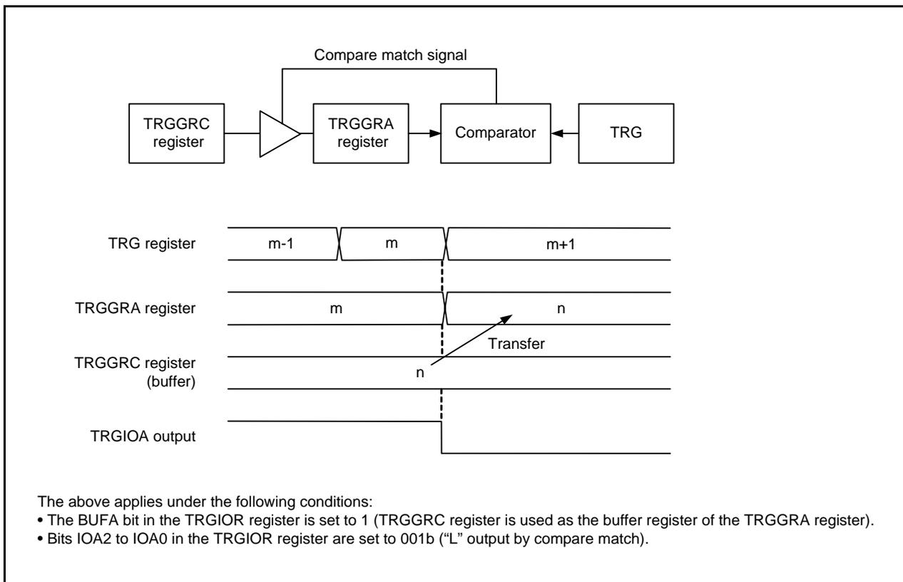
**Figure 23.4** Buffer Operation for Output Compare Function
