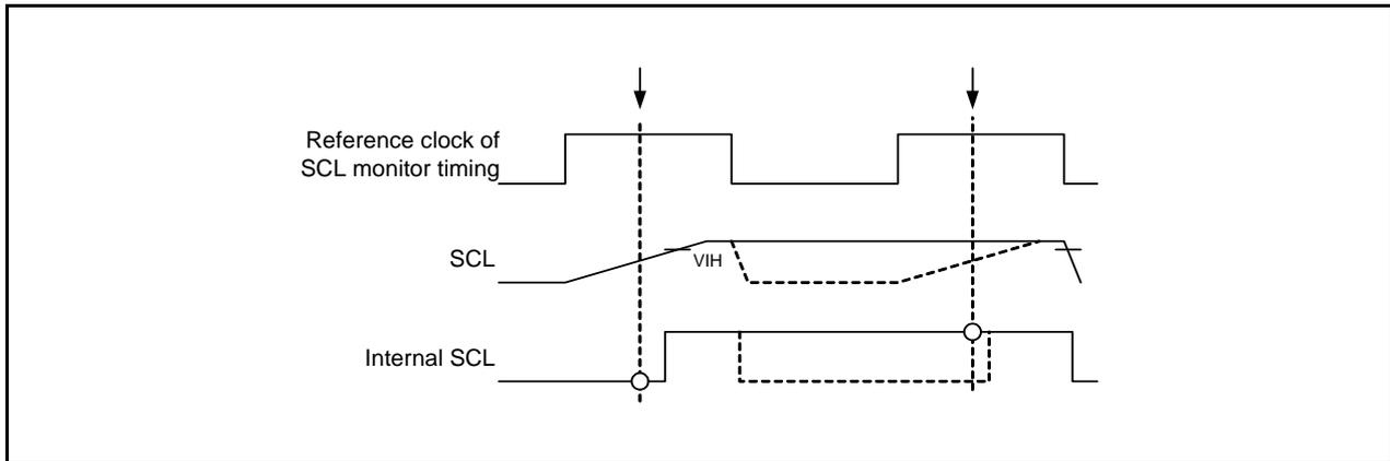
Figure 28.21 Bit Synchronization Circuit Timing
