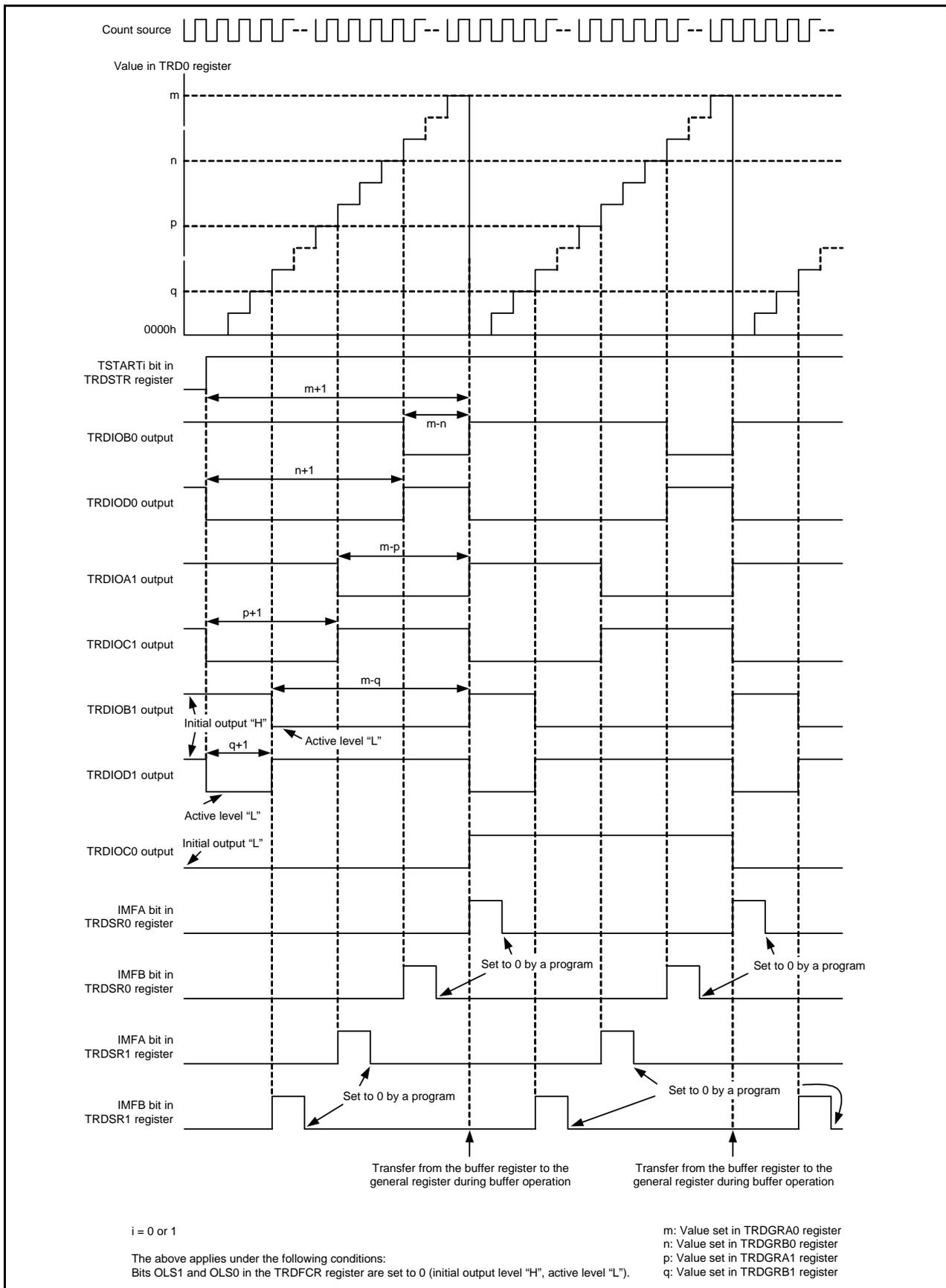
Figure 20.18 Operating Example of Reset Synchronous PWM Mode
