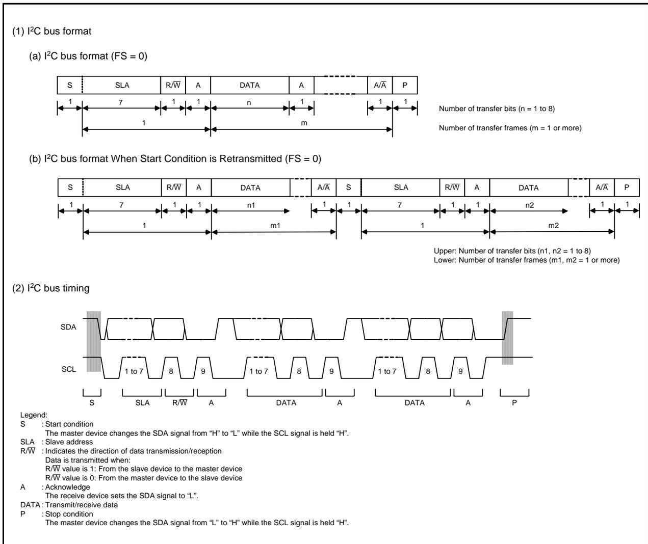
Figure 28.4 I<sup>2</sup>C bus Format and Bus Timing
