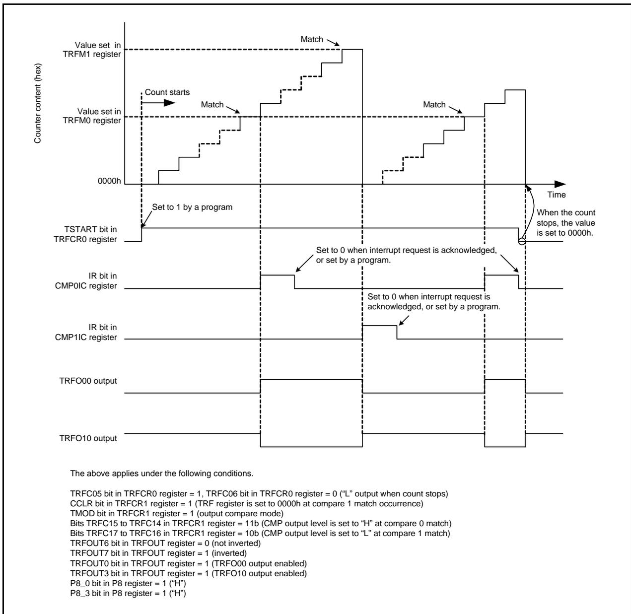
**Figure 22.6 Operating Example in Output Compare Mode**
