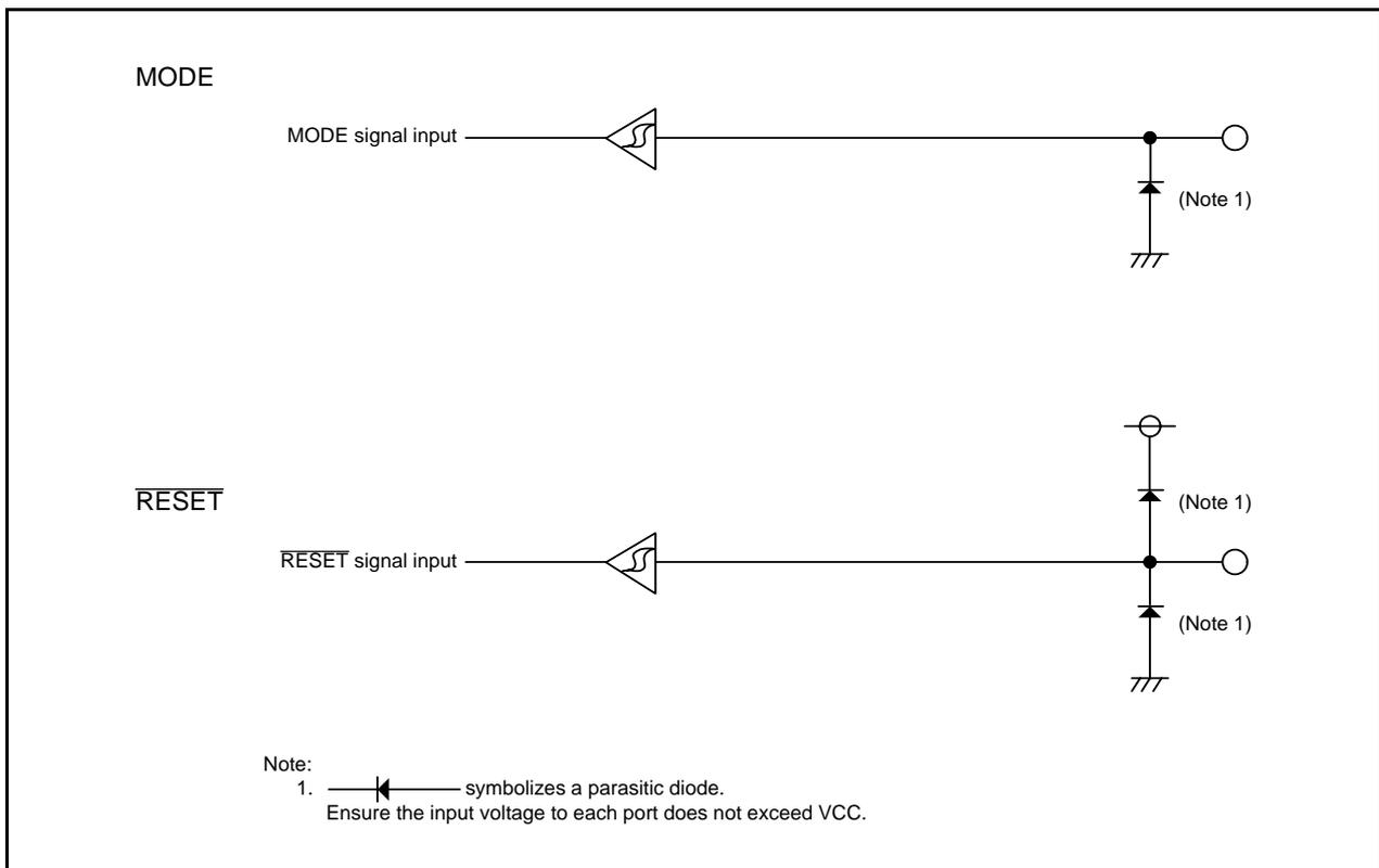
Figure 7.22 Configuration of I/O Pins
