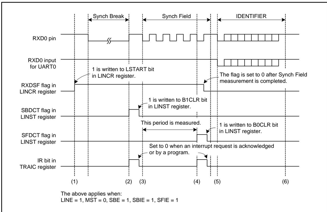
**Figure 29.5 Operating Example during Header Field Reception**
