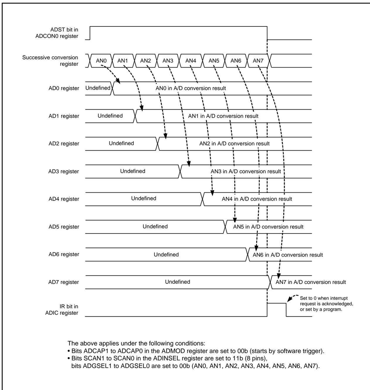
**Figure 30.8** Operating Example of Single Sweep Mode
