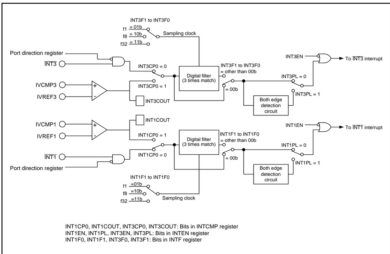
**Figure 32.1 Comparator B Block Diagram**
