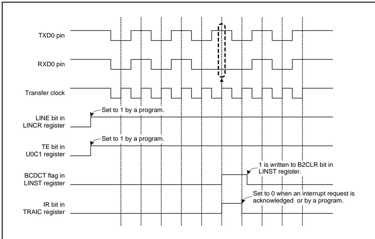
Figure 29.9 Operating Example When Bus Collision is Detected
