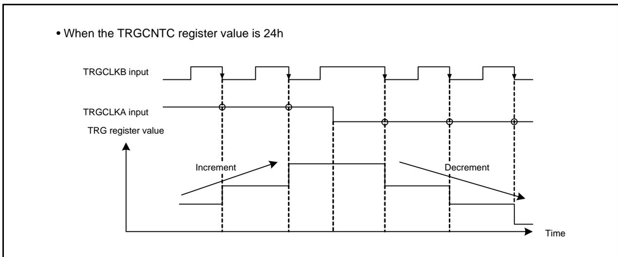
Figure 23.18 Operating Example 2 in Phase Counting Mode
