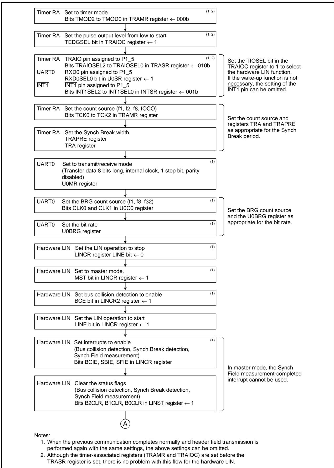
Figure 29.3 Header Field Transmission Flowchart Example (1)
