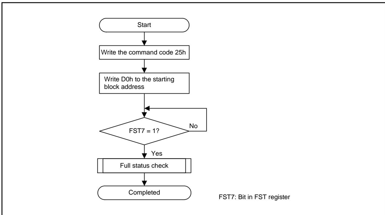
**Figure 33.16** Block Blank Check Flowchart
