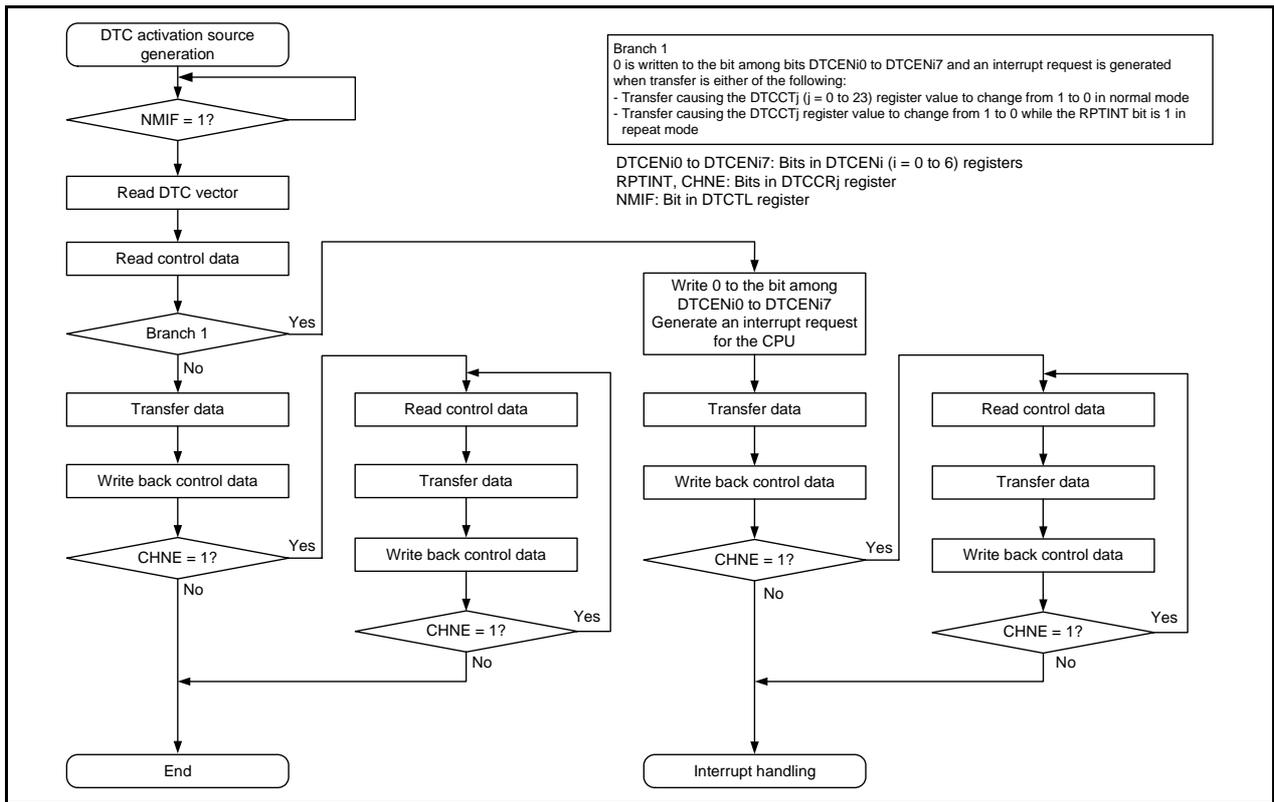
**Figure 15.3 DTC Internal Operation Flowchart When DTC Activation Source is not SSU/I<sup>2</sup>C bus, Timer RC, Timer RD, Timer RG, or Flash Memory Interrupt Source**
