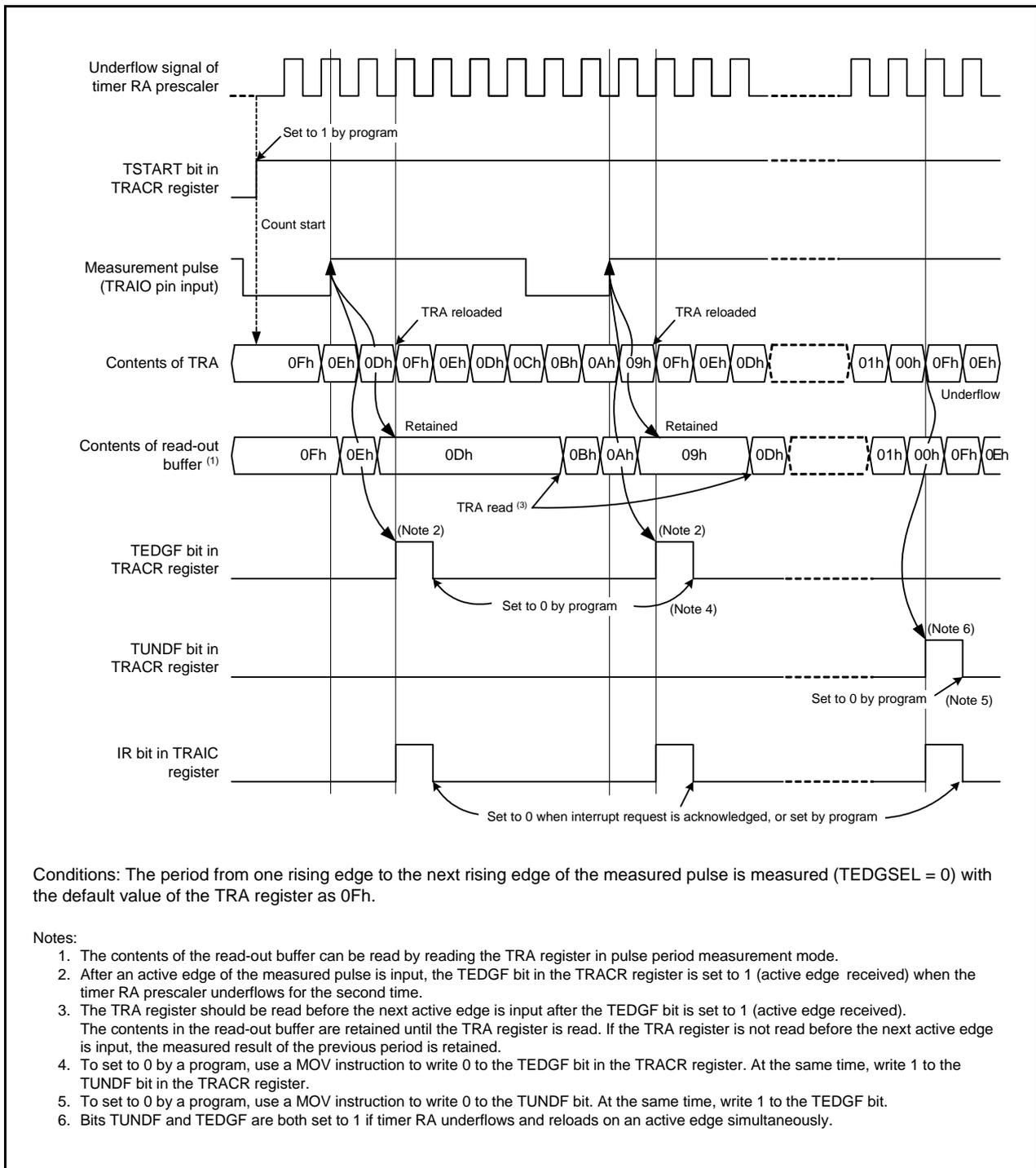
Figure 17.4 Operating Example of Pulse Period Measurement Mode
