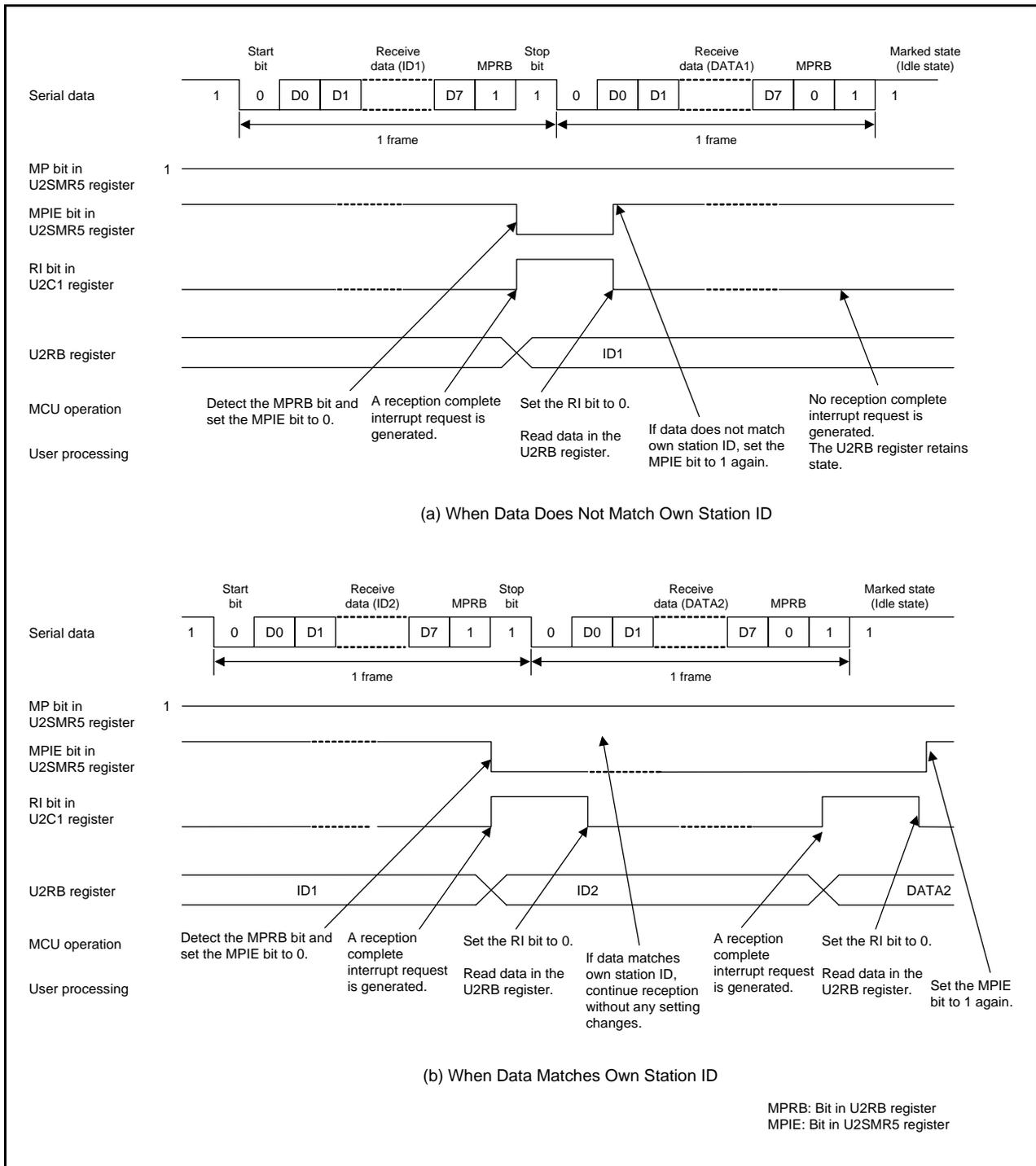
Figure 25.21 Receive Operation Example during Multiprocessor Communication (with 8-Bit Data/Multiprocessor Bit/One-Stop Bit)
