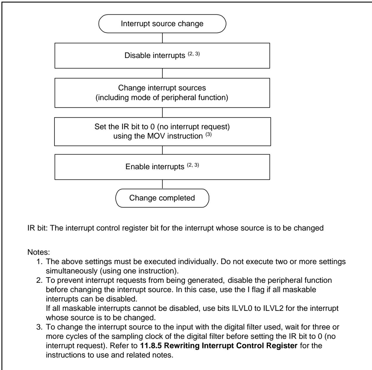
Figure 36.1 Procedure Example for Changing Interrupt Sources
