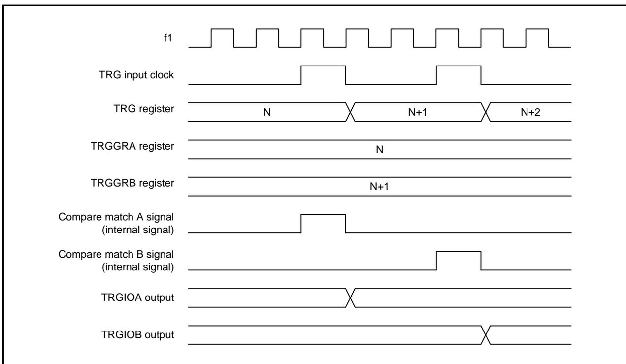
Figure 23.10 Output-Compare Output Timing
