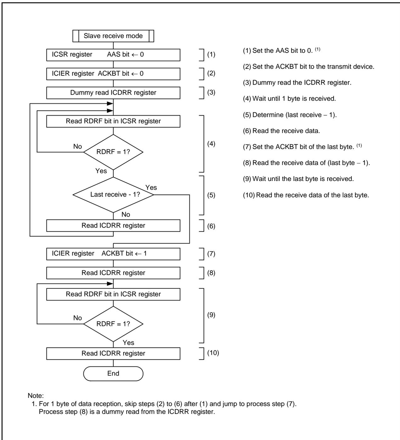
**Figure 28.19 Register Setting Example in Slave Receive Mode (I<sup>2</sup>C bus Interface Mode)**
