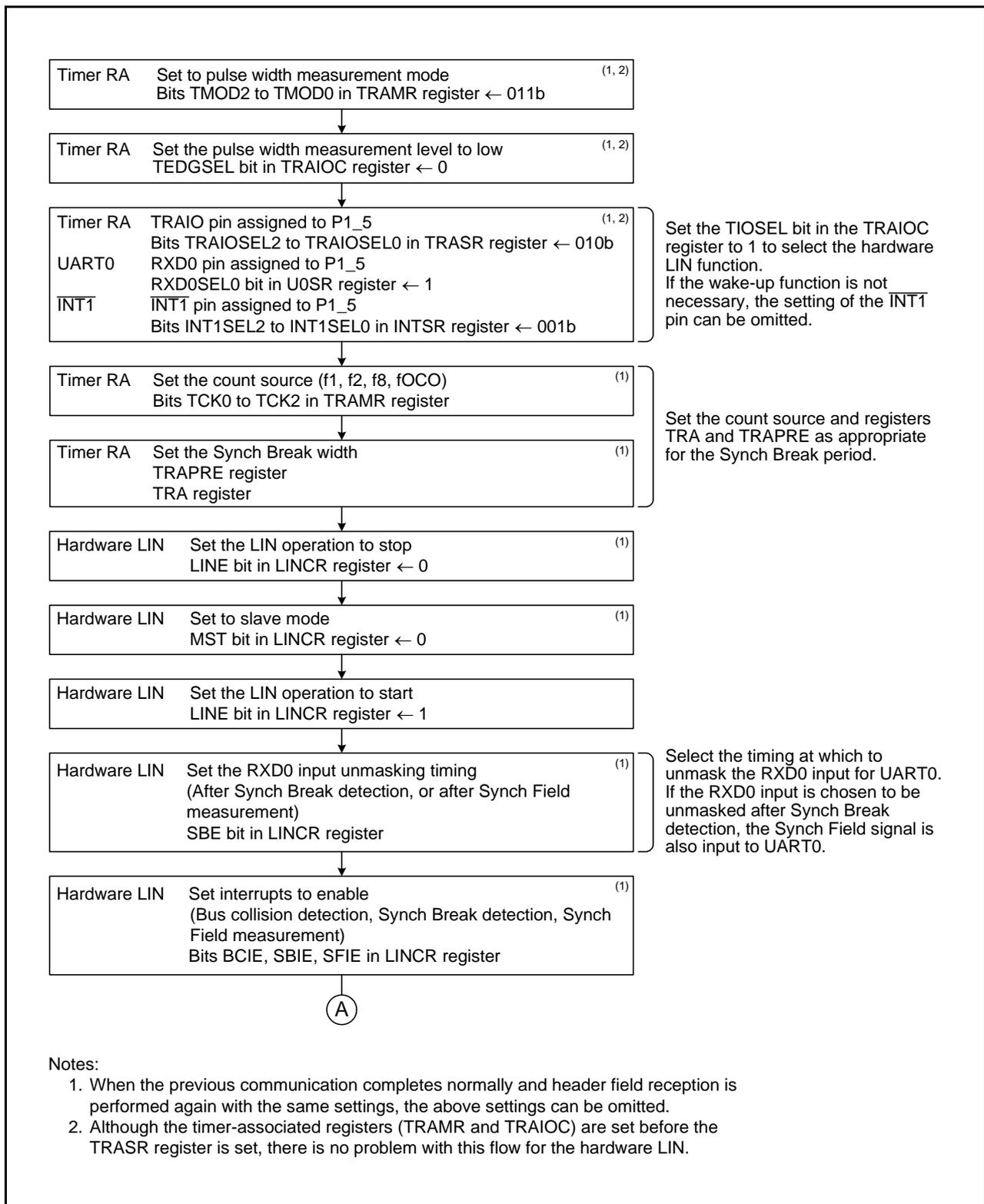
Figure 29.6 Header Field Reception Flowchart Example (1)
