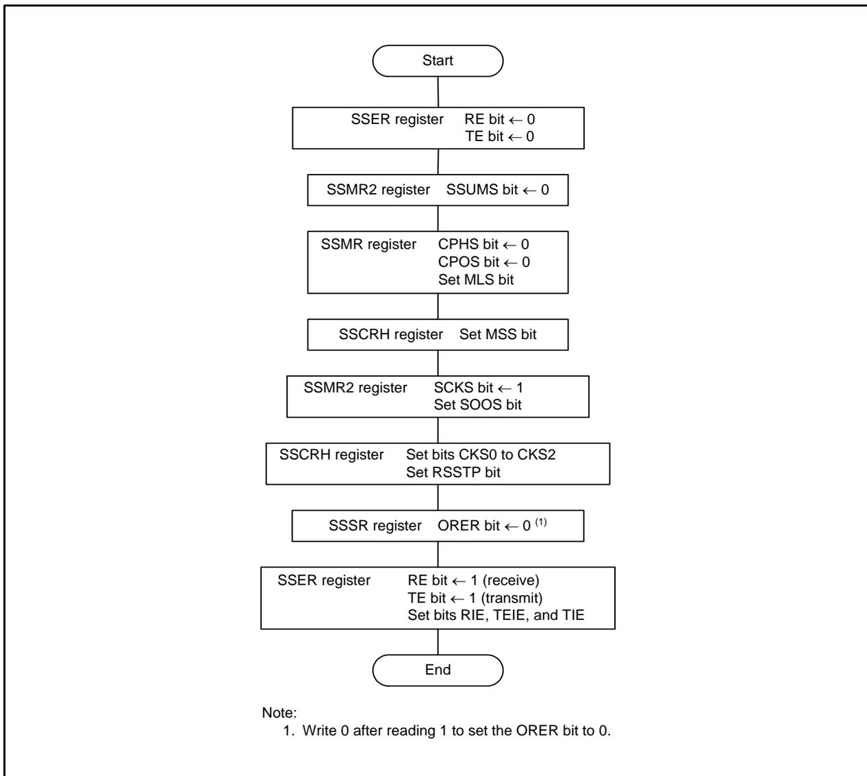
Figure 27.4 Initialization in Clock Synchronous Communication Mode
