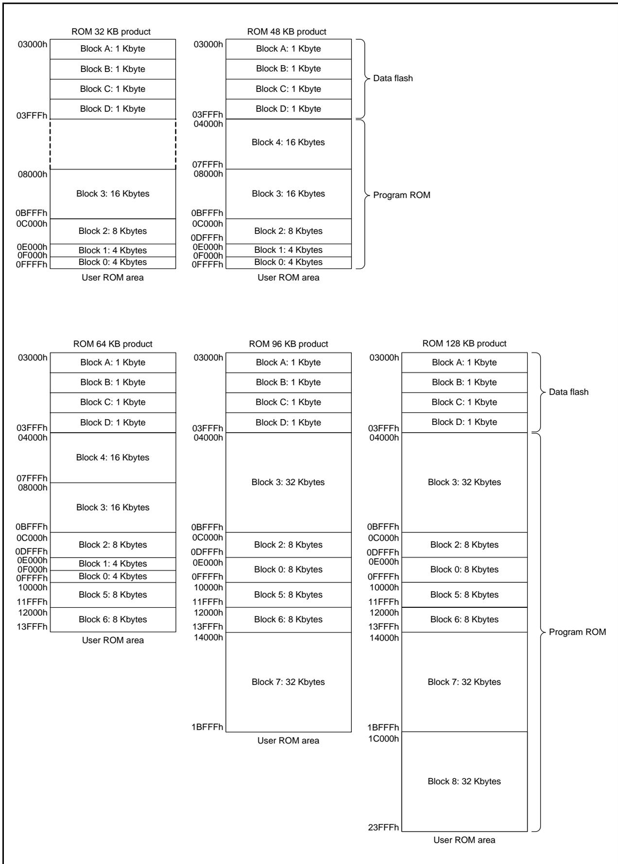
Figure 33.2 R8C/38C Group Flash Memory Block Diagram (2)
