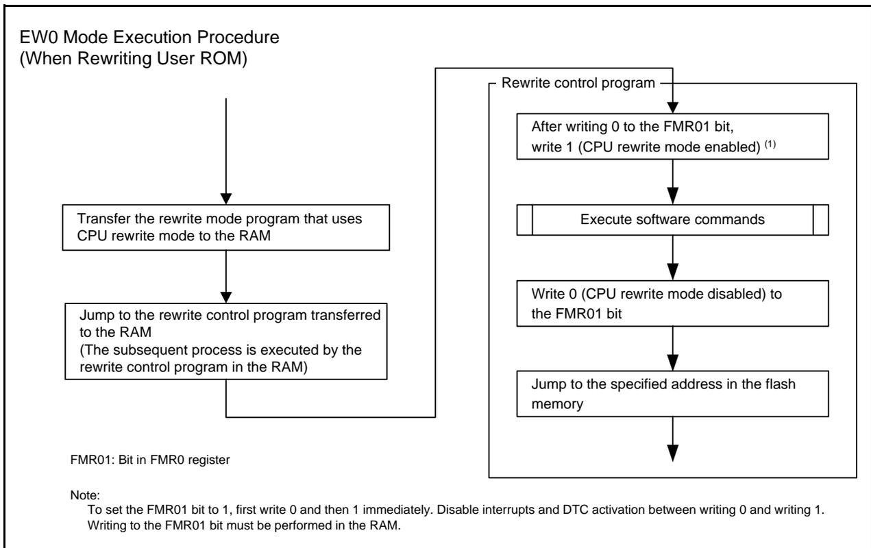
**Figure 33.5 How to Set and Exit EW0 Mode**
