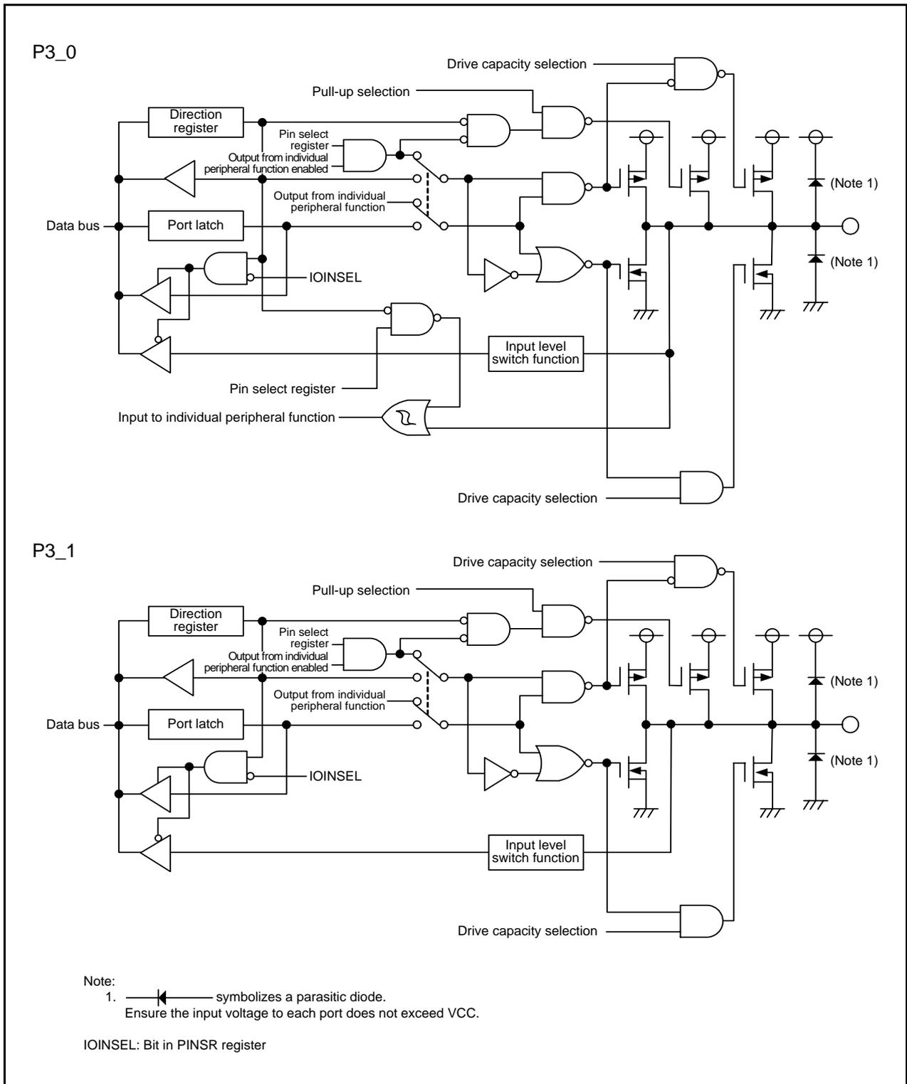
Figure 7.6 Configuration of I/O Ports (6)
