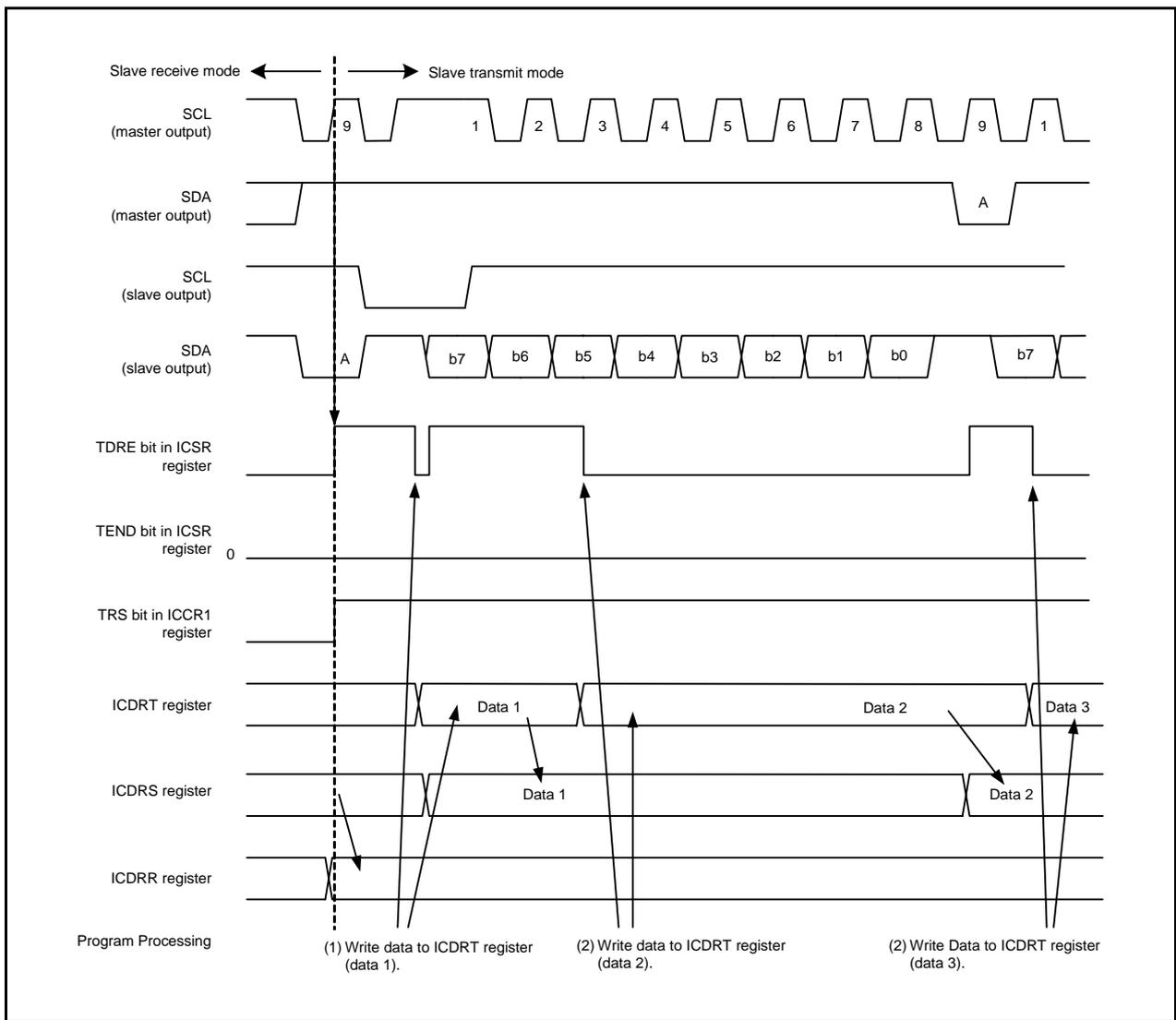
**Figure 28.9 Operating Timing in Slave Transmit Mode (I<sup>2</sup>C bus Interface Mode) (1)**
