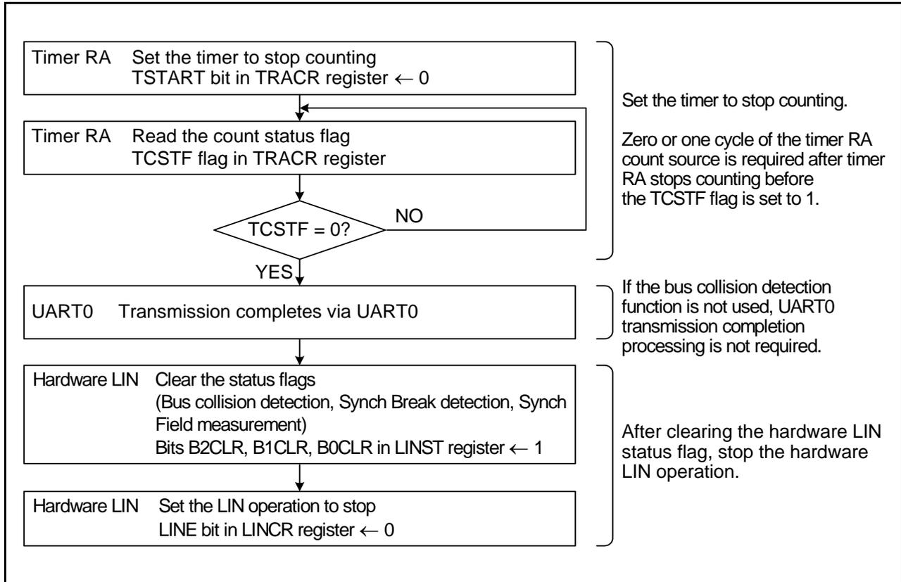
Figure 29.10 Example of Hardware LIN Communication Completion Flowchart
