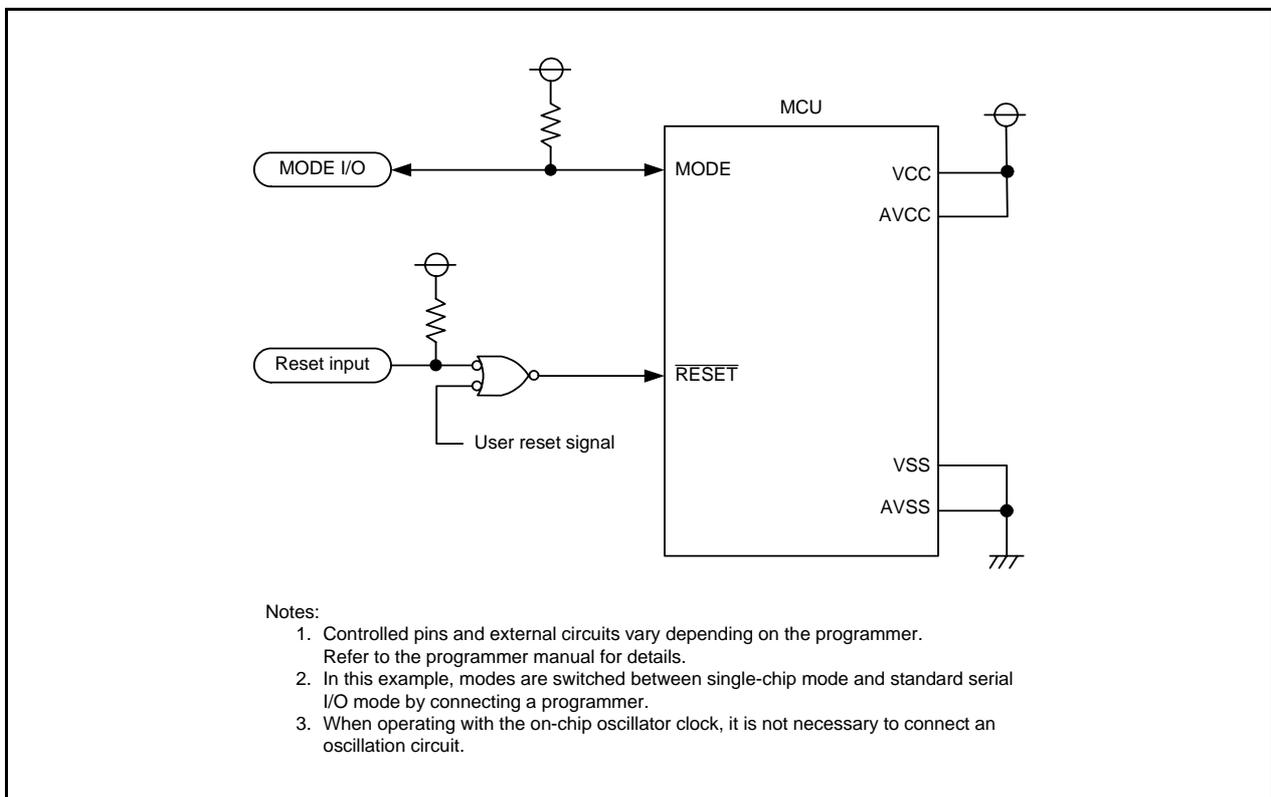
**Figure 33.19 Pin Handling in Standard Serial I/O Mode 3**
