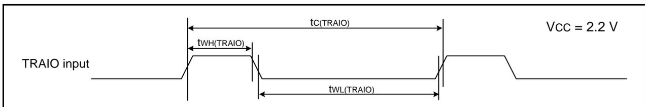
**Figure 35.19 TRAIO Input Timing Diagram when  $V_{CC} = 2.2\text{ V}$**
