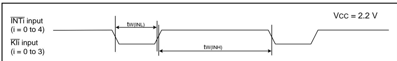
**Figure 35.22 Input Timing Diagram for External Interrupt  $\overline{\text{INT}}_i$  and Key Input Interrupt  $\overline{\text{KLI}}_i$  when  $V_{cc} = 2.2 \text{ V}$**
