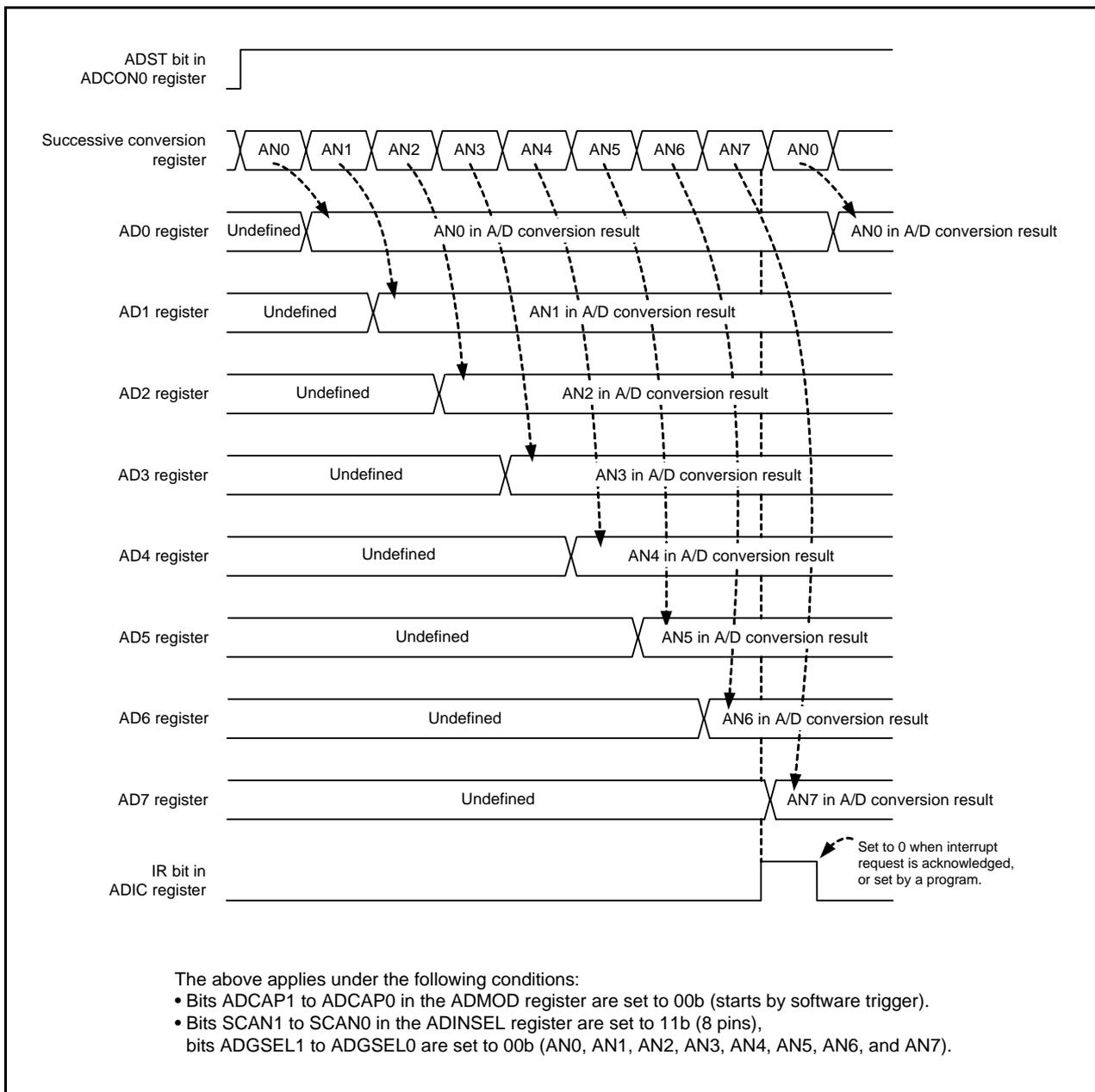
**Figure 30.9** Operating Example of Repeat Sweep Mode
