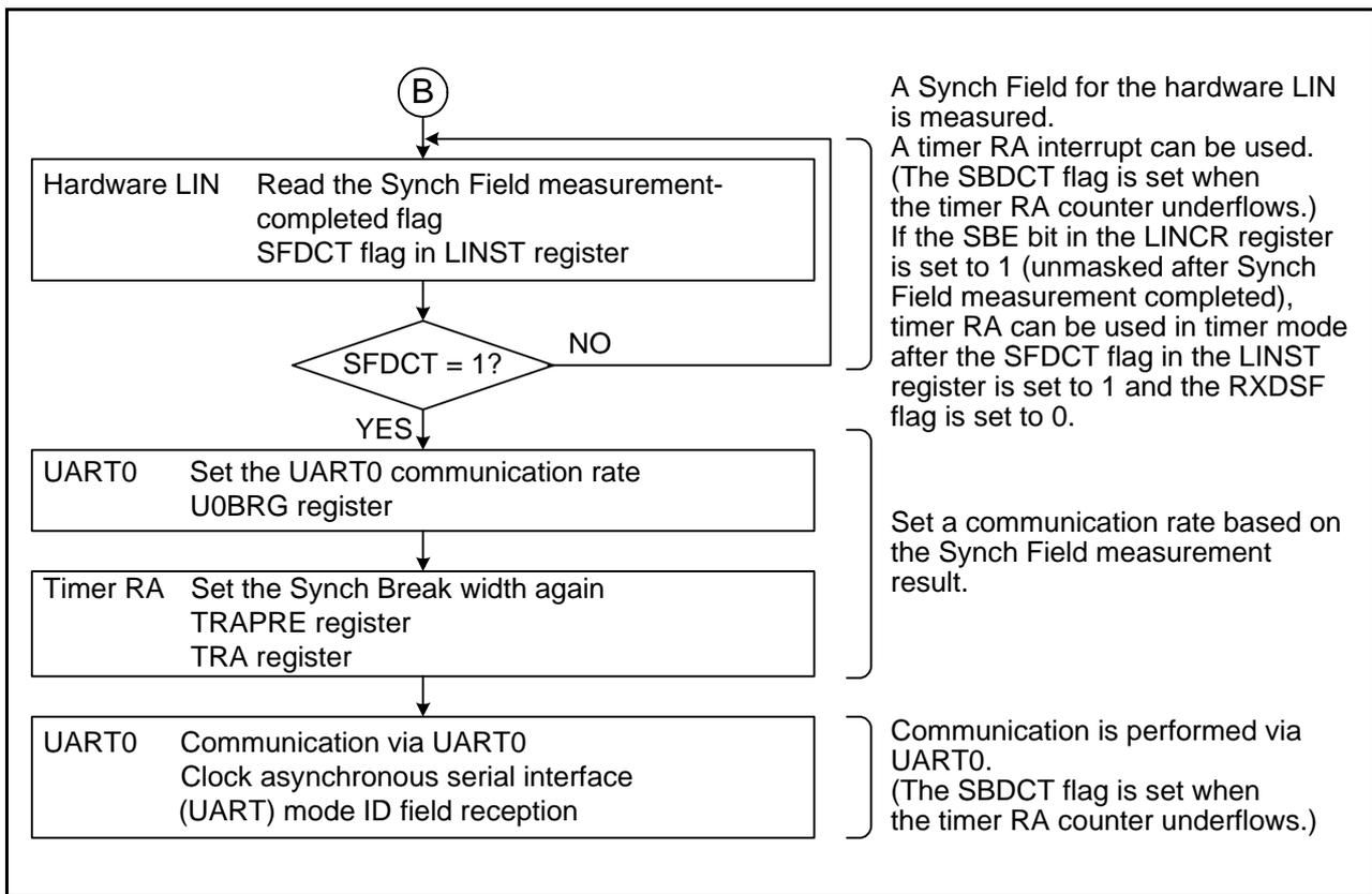
Figure 29.8 Header Field Reception Flowchart Example (3)
