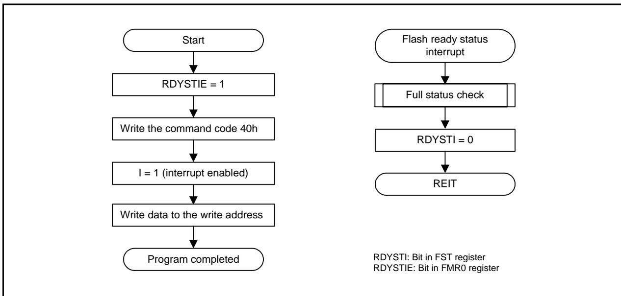
**Figure 33.10 Program Flowchart (Flash Ready Status Interrupt Enabled)**
