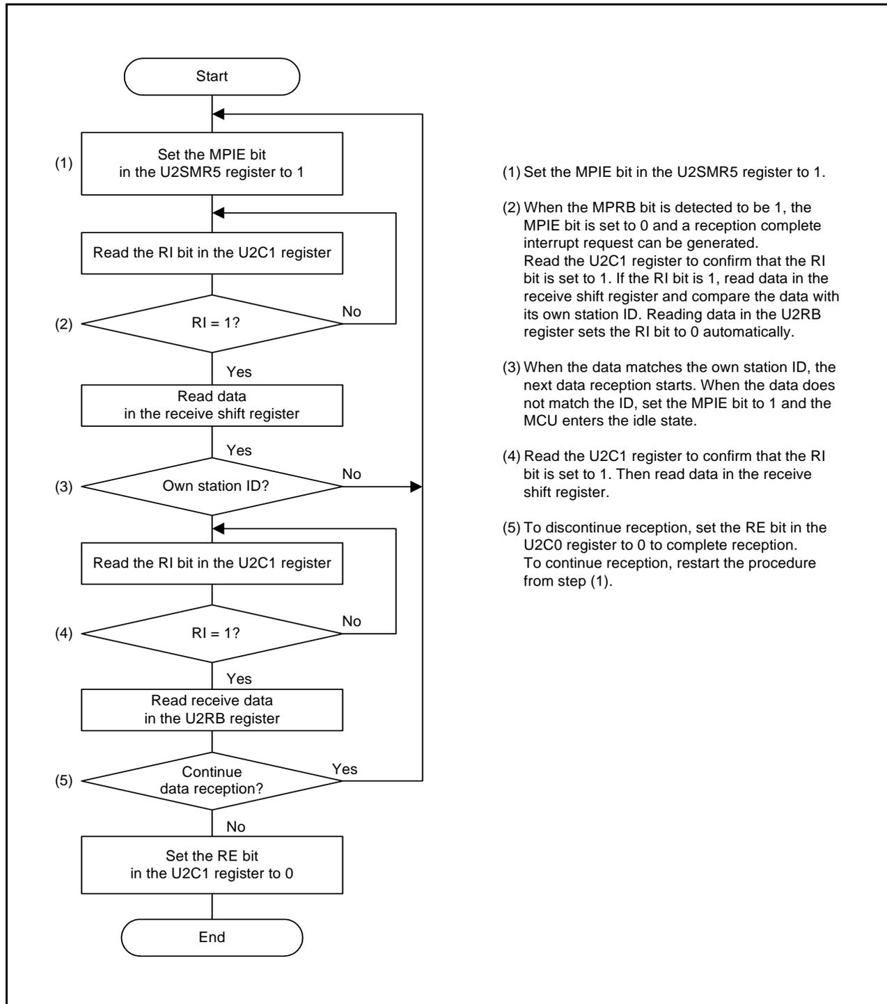
Figure 25.20 Sample Flowchart of Multiprocessor Data Reception
