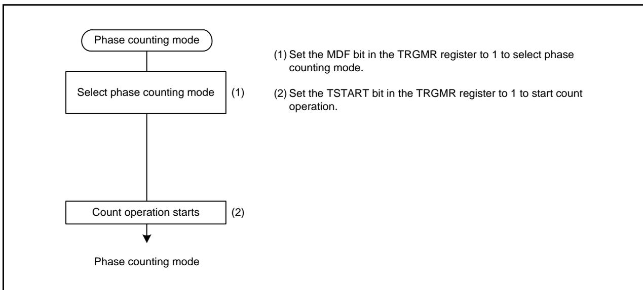
Figure 23.16 Procedure Example for Setting Phase Counting Mode
