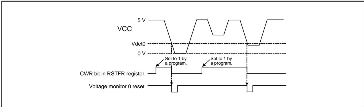
Figure 5.8 Operating Example of Cold Start-Up/Warm Start-Up Function
