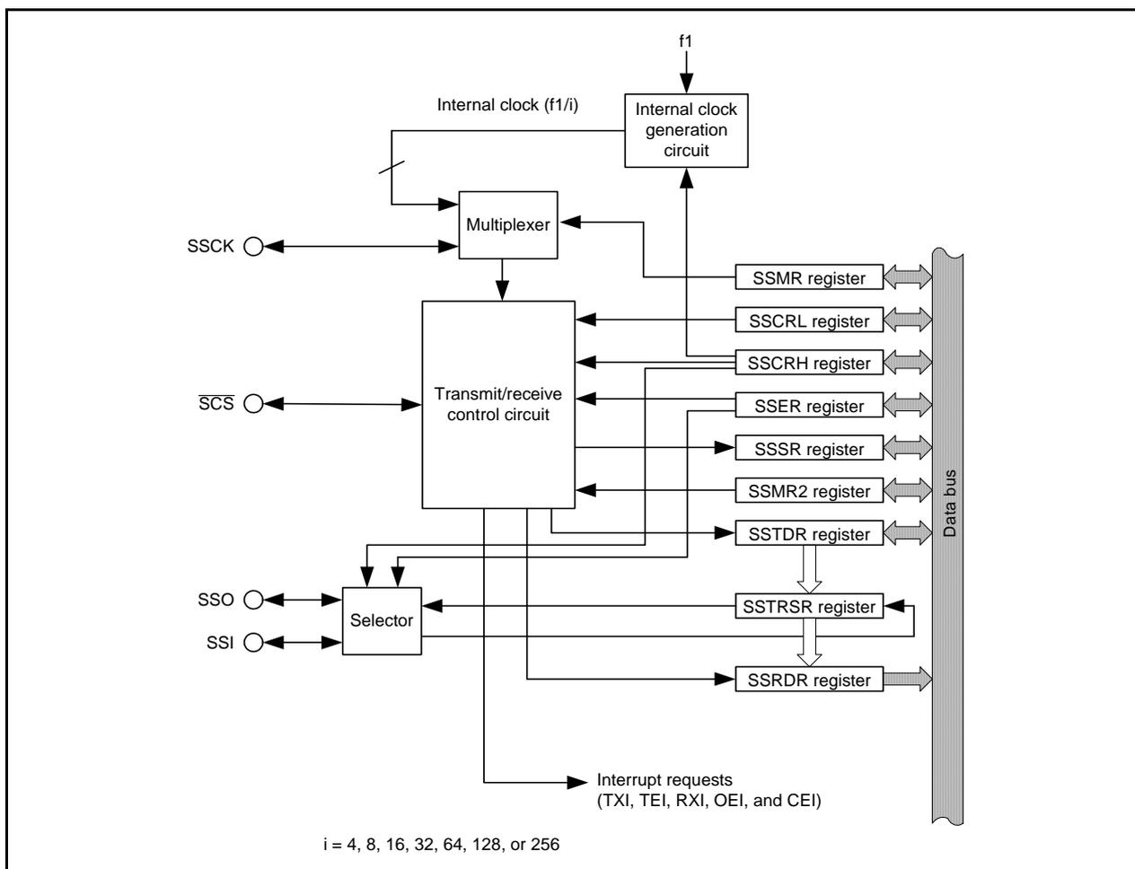
Figure 27.1 Block Diagram of Synchronous Serial Communication Unit
