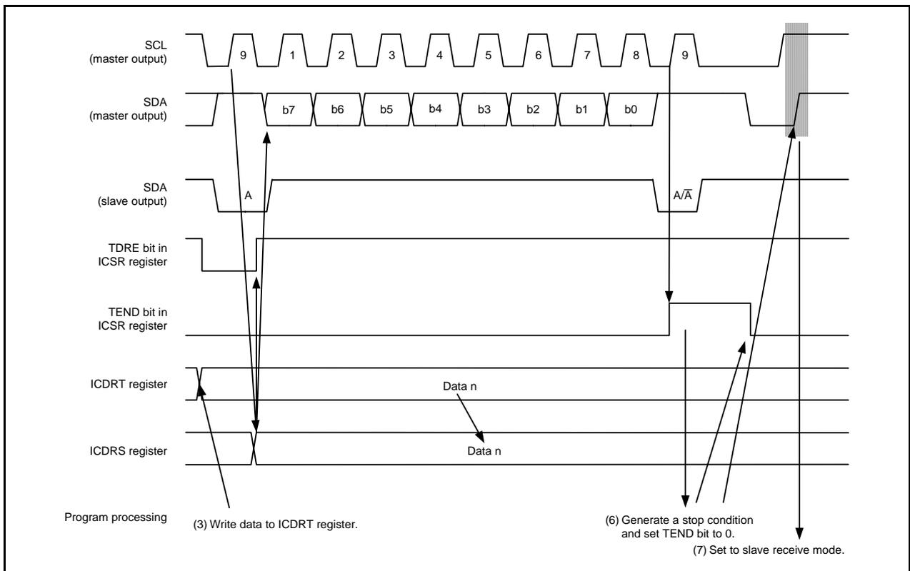
Figure 28.6 Operating Timing in Master Transmit Mode (I<sup>2</sup>C bus Interface Mode) (2)
