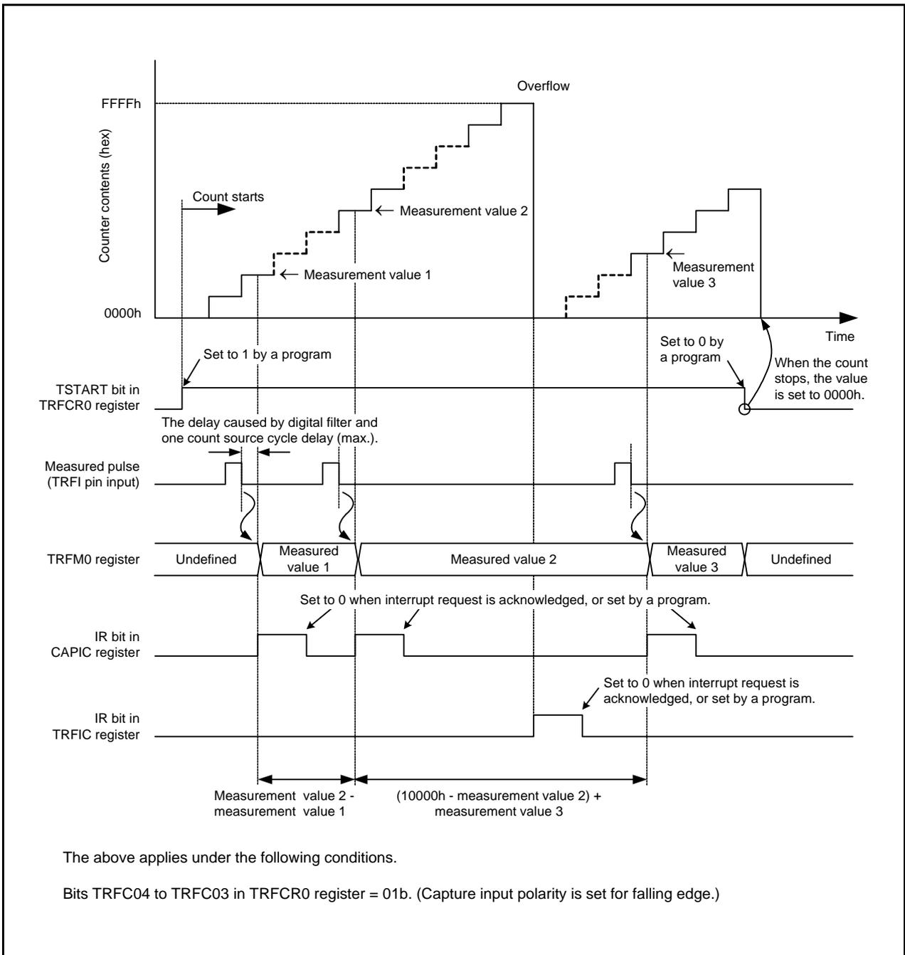
Figure 22.4 Operating Example in Input Capture Mode
