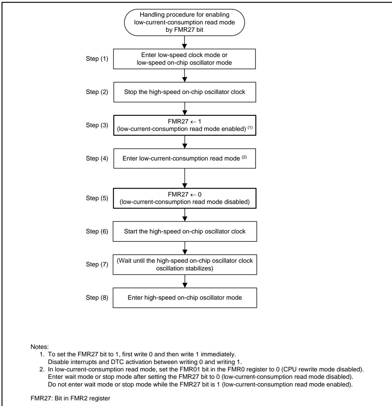
**Figure 34.3 Handling Procedure Example of Low-Current-Consumption Read Mode**
