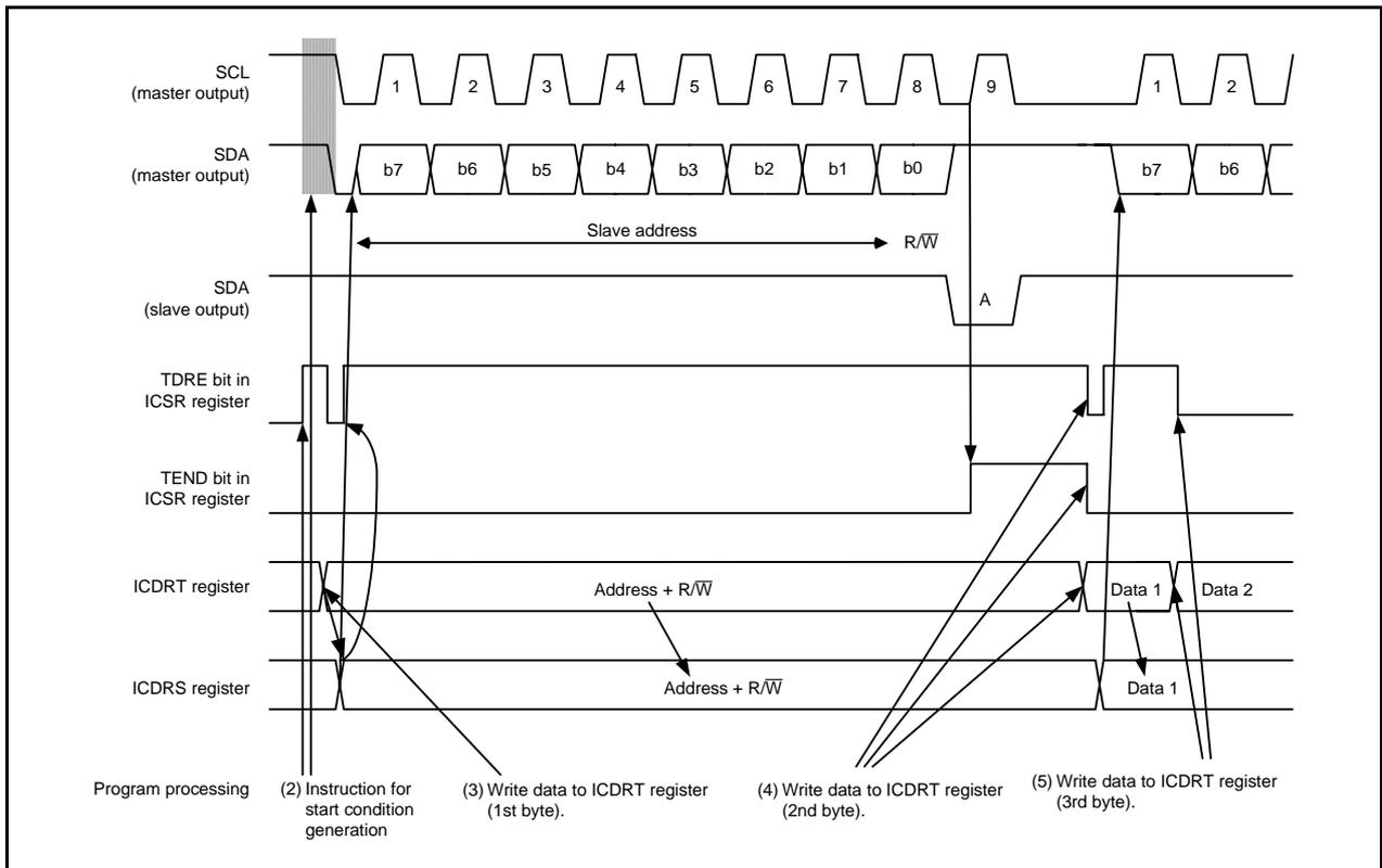
Figure 28.5 Operating Timing in Master Transmit Mode (I<sup>2</sup>C bus Interface Mode) (1)
