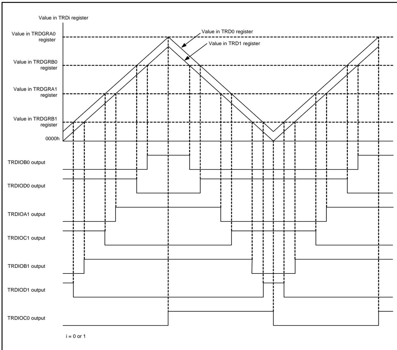
Figure 20.20 Output Model of Complementary PWM Mode
