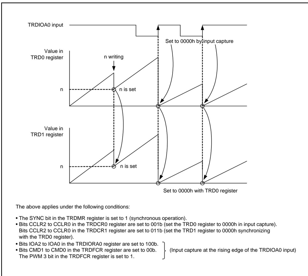
Figure 20.5 Synchronous Operation
