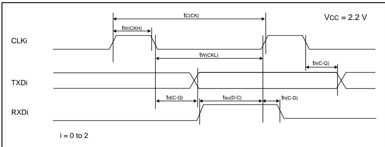
**Figure 35.21 Serial Interface Timing Diagram when  $V_{cc} = 2.2 \text{ V}$**
