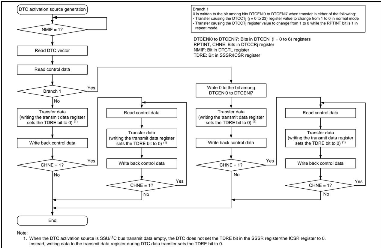
**Figure 15.6 DTC Internal Operation Flowchart When DTC Activation Source is SSU/I<sup>2</sup>C bus Transmit Data Empty**
