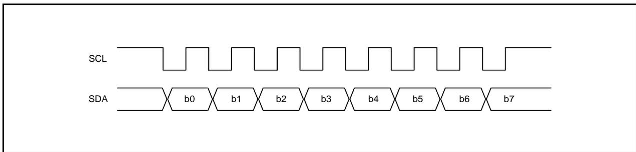
Figure 28.13 Transfer Format of Clock Synchronous Serial Format
