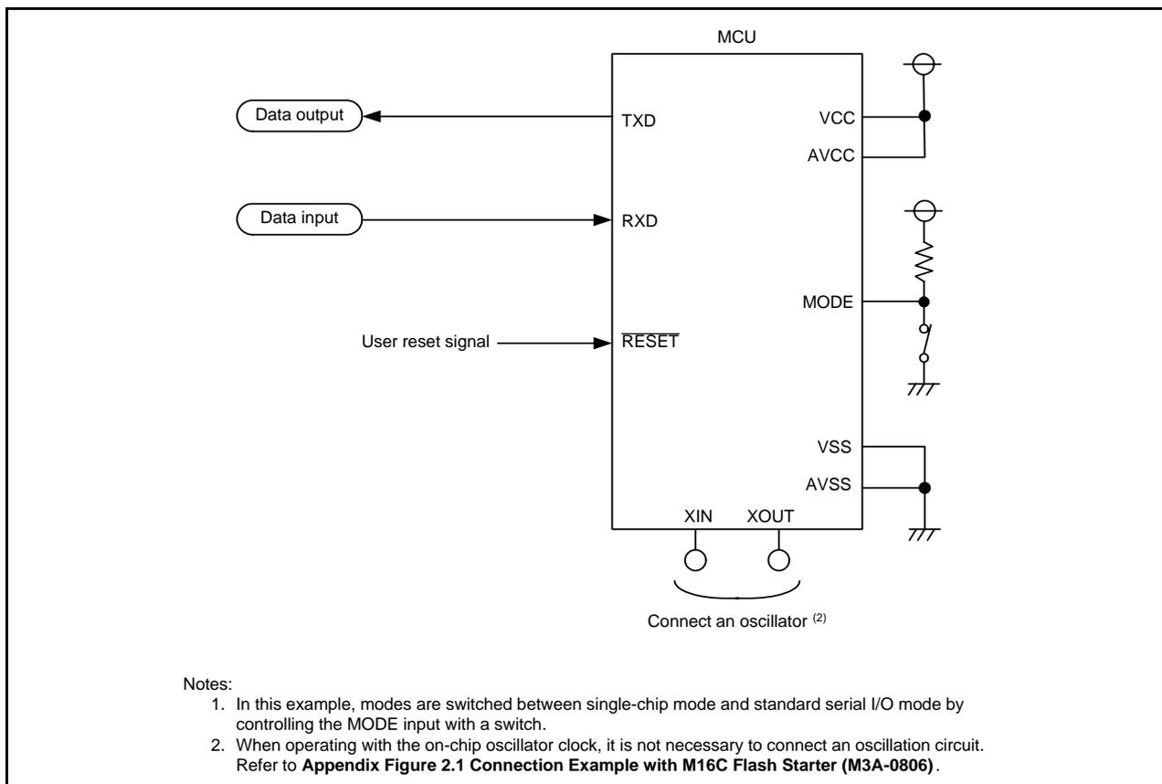
**Figure 33.18 Pin Handling in Standard Serial I/O Mode 2**
