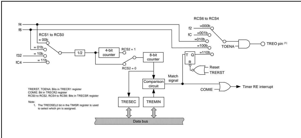
Figure 21.4 Block Diagram of Output Compare Mode
