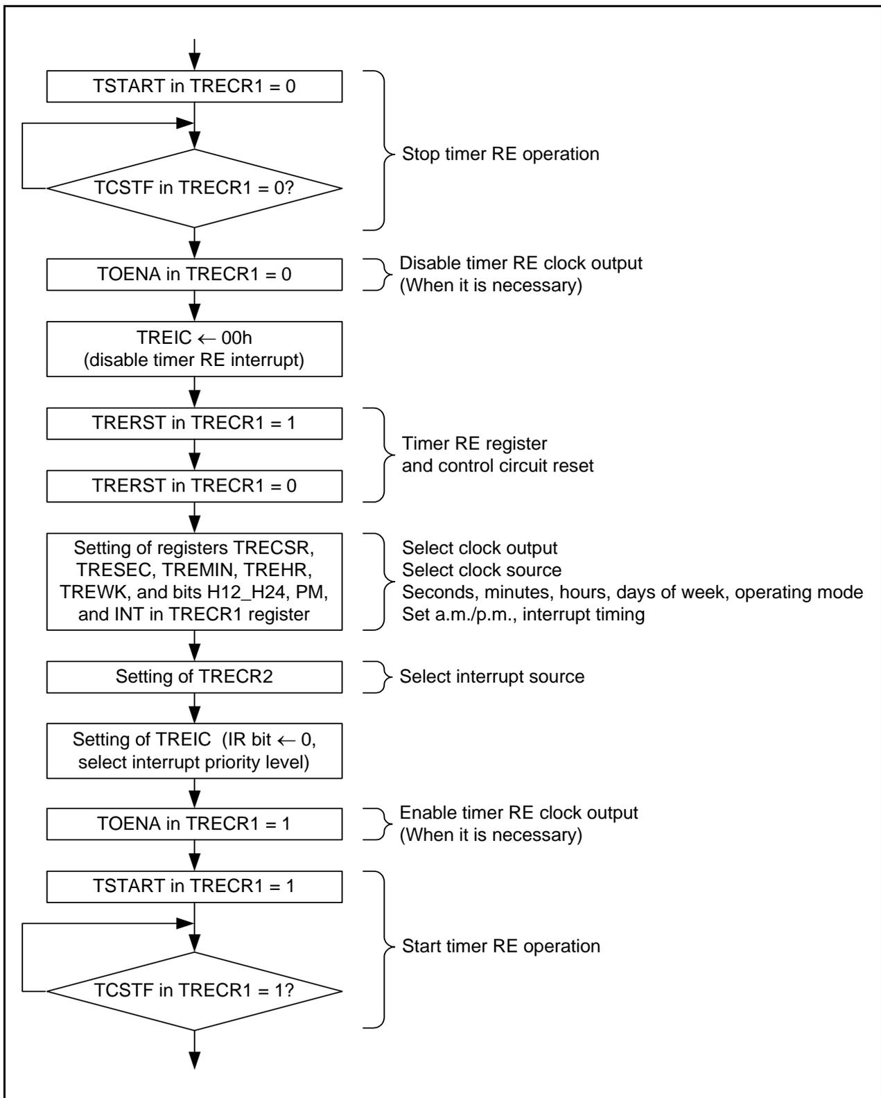
Figure 21.6 Setting Example in Real-Time Clock Mode
