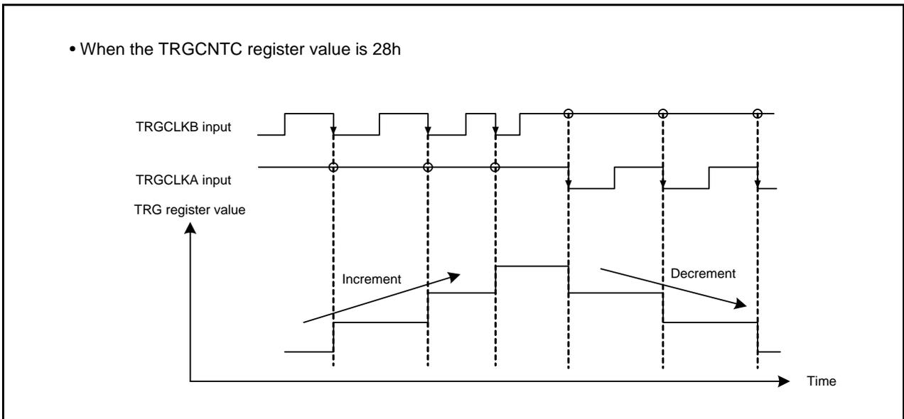
Figure 23.19 Operating Example 3 in Phase Counting Mode
