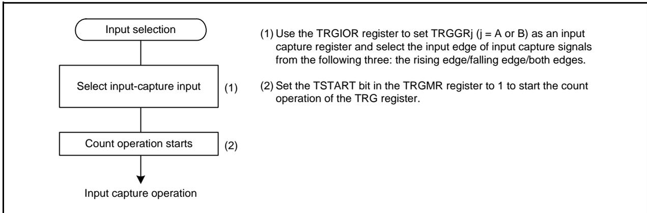
Figure 23.6 Procedure Example for Setting Input Capture Operation
