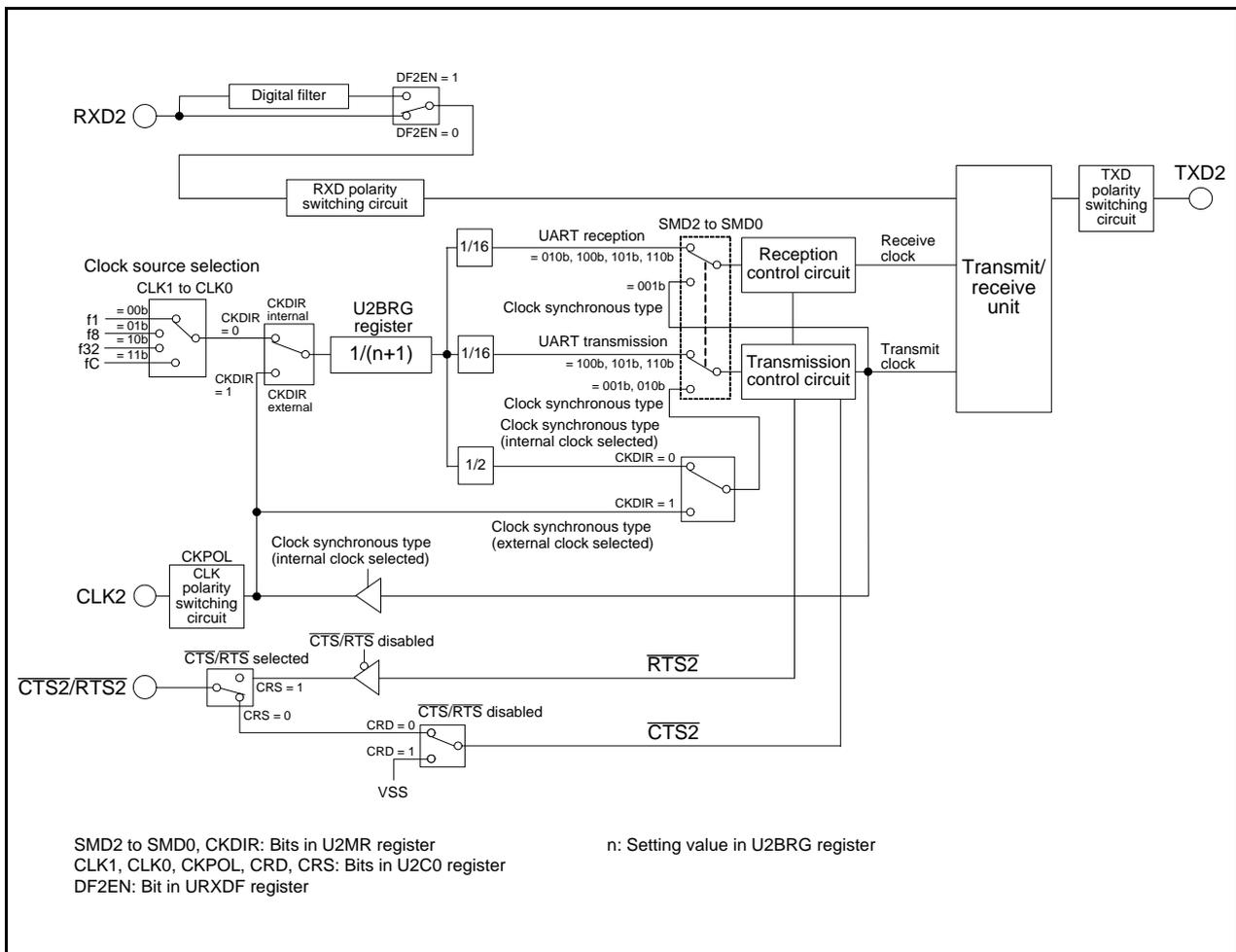
Figure 25.1 UART2 Block Diagram
