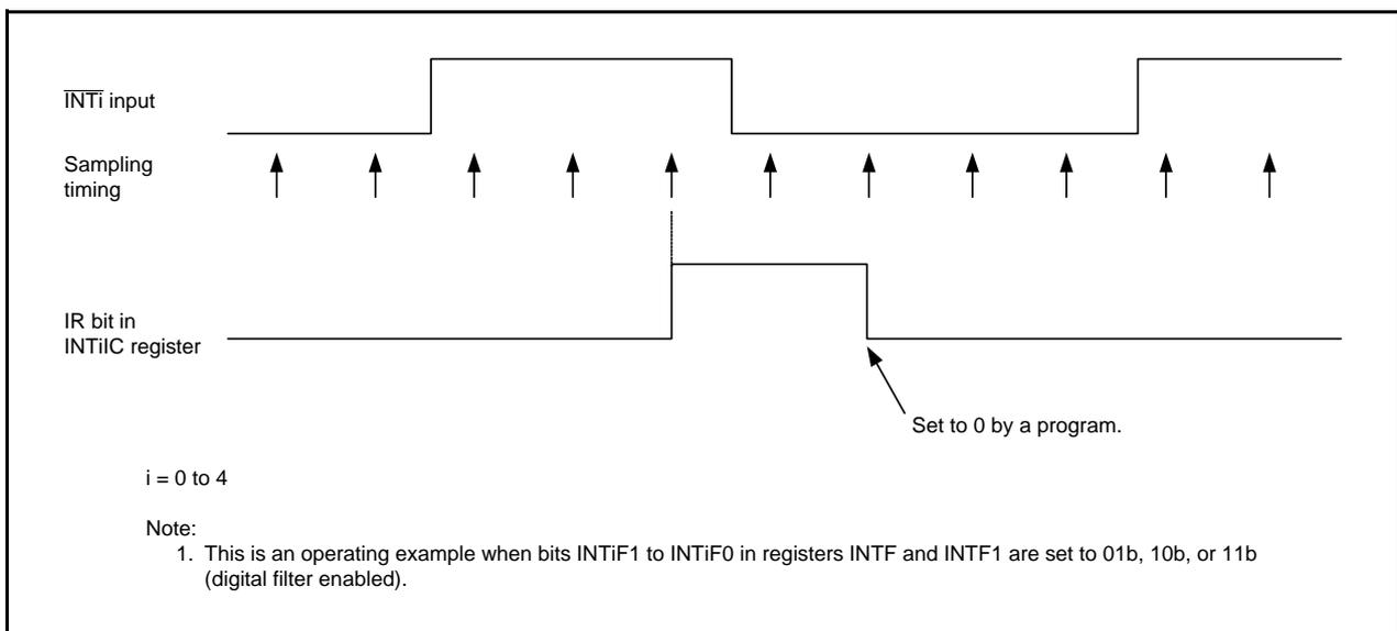
Figure 11.10 Operating Example of  $\overline{\text{INT}}_i$  Input Filter
