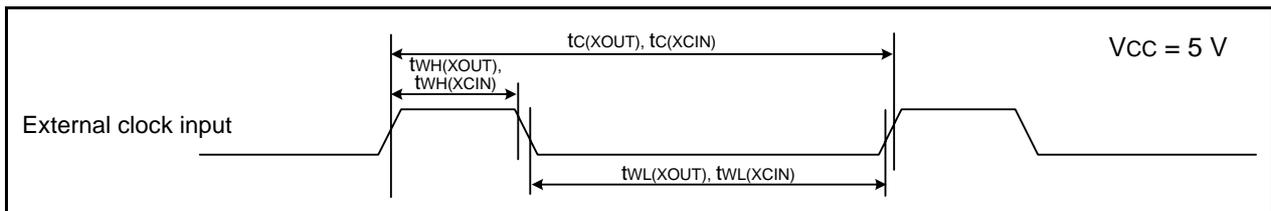
**Figure 35.8 External Clock Input Timing Diagram when  $V_{CC} = 5\text{ V}$** **Table 35.20 TRAI0 Input**
