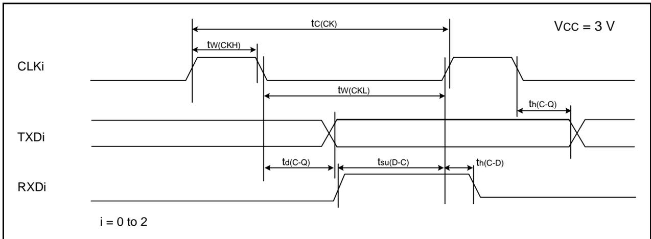
**Figure 35.16 Serial Interface Timing Diagram when Vcc = 3 V**
