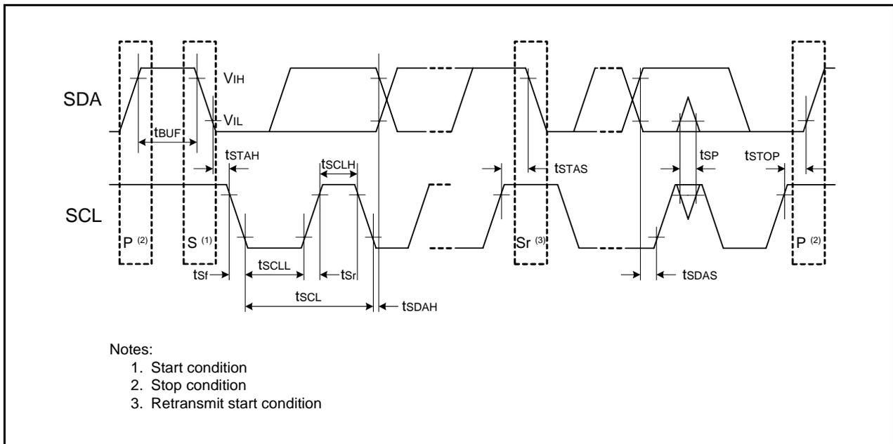
**Figure 35.7 I/O Timing of I<sup>2</sup>C bus Interface**
