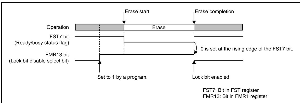
**Figure 33.8 FMR13 Bit Operation Timing**
