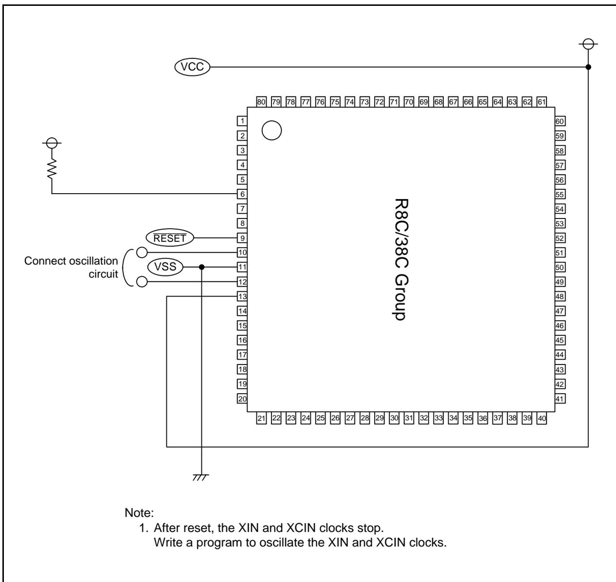
Appendix Figure 3.1 Example of Oscillation Evaluation Circuit
