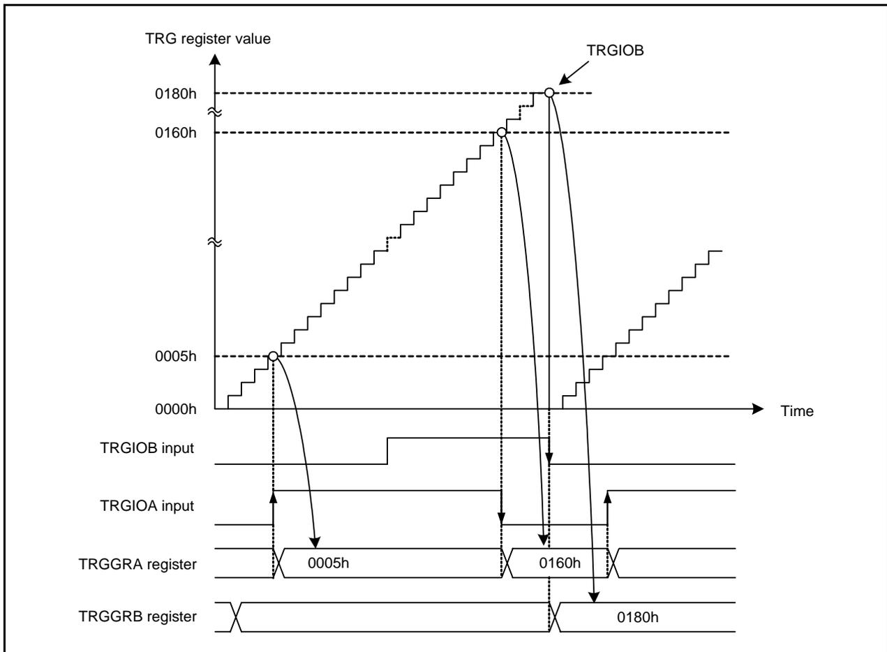
Figure 23.8 Operating Example of Input Capture
