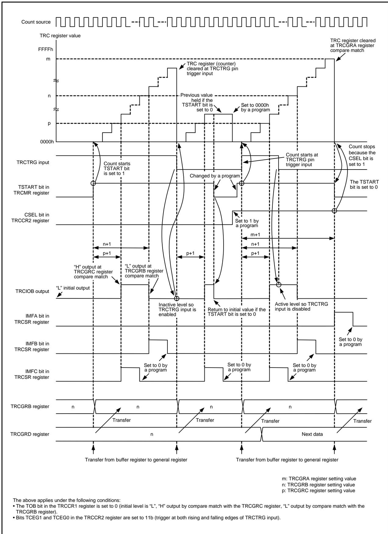
Figure 19.18 Operating Example of PWM2 Mode (TRCTRG Trigger Input Enabled)
