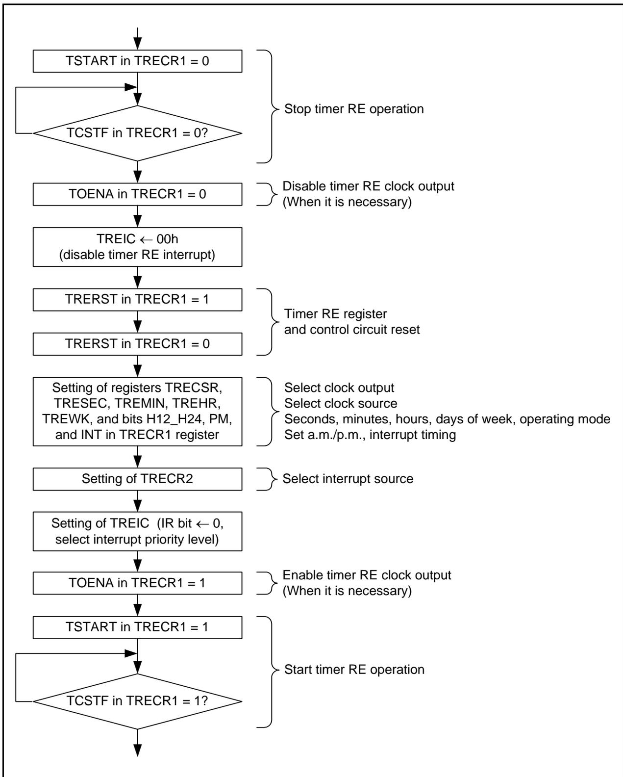
Figure 36.6 Setting Example in Real-Time Clock Mode
