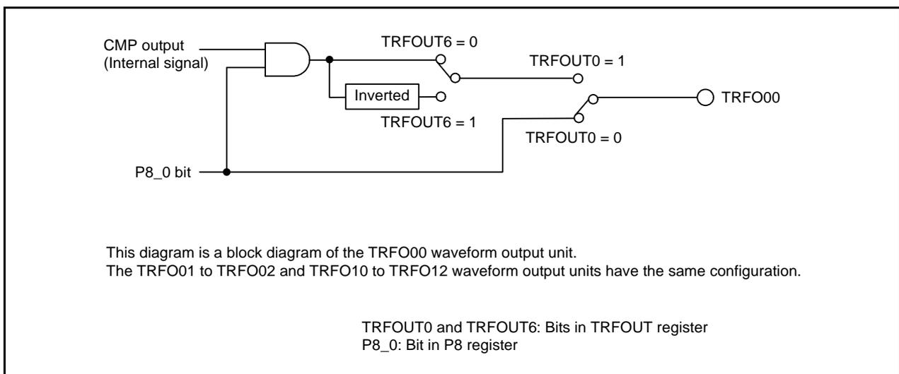
**Figure 22.3 Block Diagram of CMP Waveform Output Unit**
