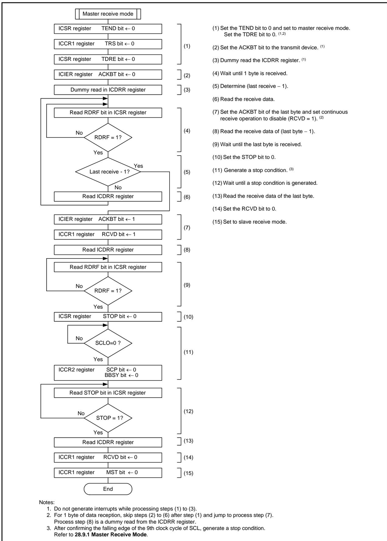
Figure 28.17 Register Setting Example in Master Receive Mode (I<sup>2</sup>C bus Interface Mode)
