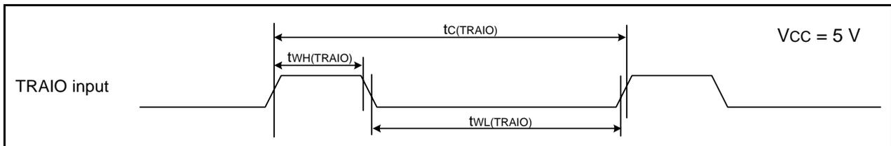
**Figure 35.9 TRAI0 Input Timing Diagram when  $V_{CC} = 5\text{ V}$** **Table 35.21 TRFI Input**
