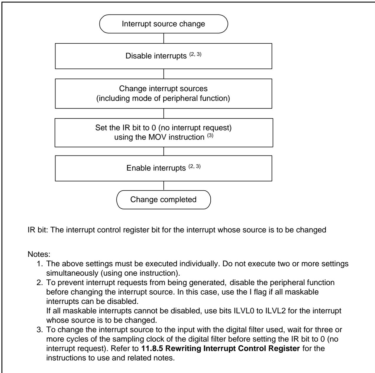
Figure 11.13 Procedure Example for Changing Interrupt Sources
