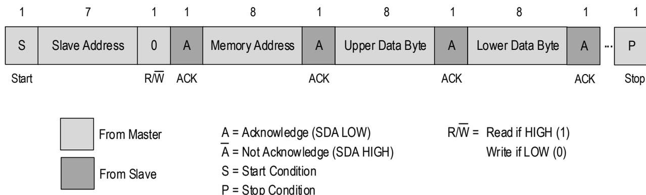
Figure 25. I2C Data BURST WRITE to Slave(s)
