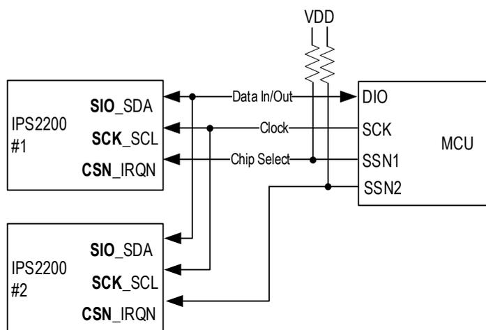
Figure 5. Half Duplex 3-3 Wire SPI Multi-slave Interface
