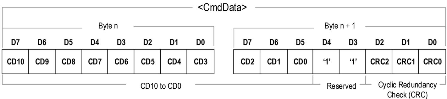
Figure 23. I2C 11-Bit Data Structure
