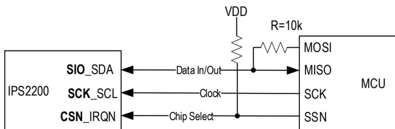
**Figure 7. Half Duplex 3-4 Wire SPI Interface**
