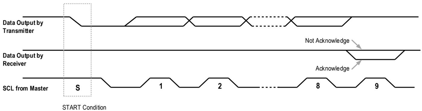
Figure 19. I2C Acknowledge Signal State
