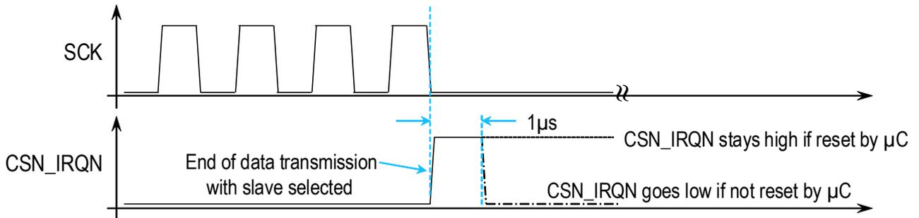
Figure 14. Half Duplex SPI IRQN Diagnostic Detection – End of the Frame
