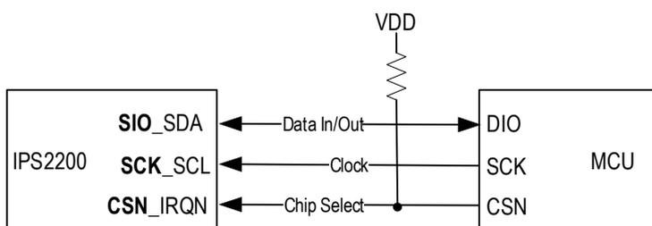
Figure 4. Half Duplex 3-3 Wire SPI Interface
