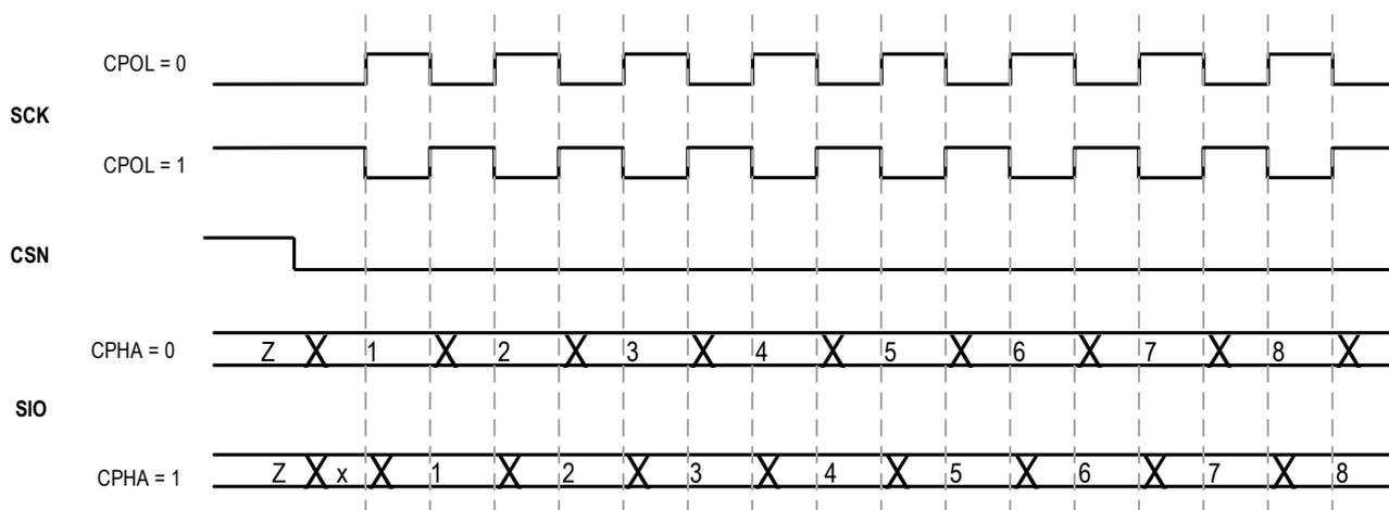
**Figure 6. SPI 3-Wire Operating Mode**
