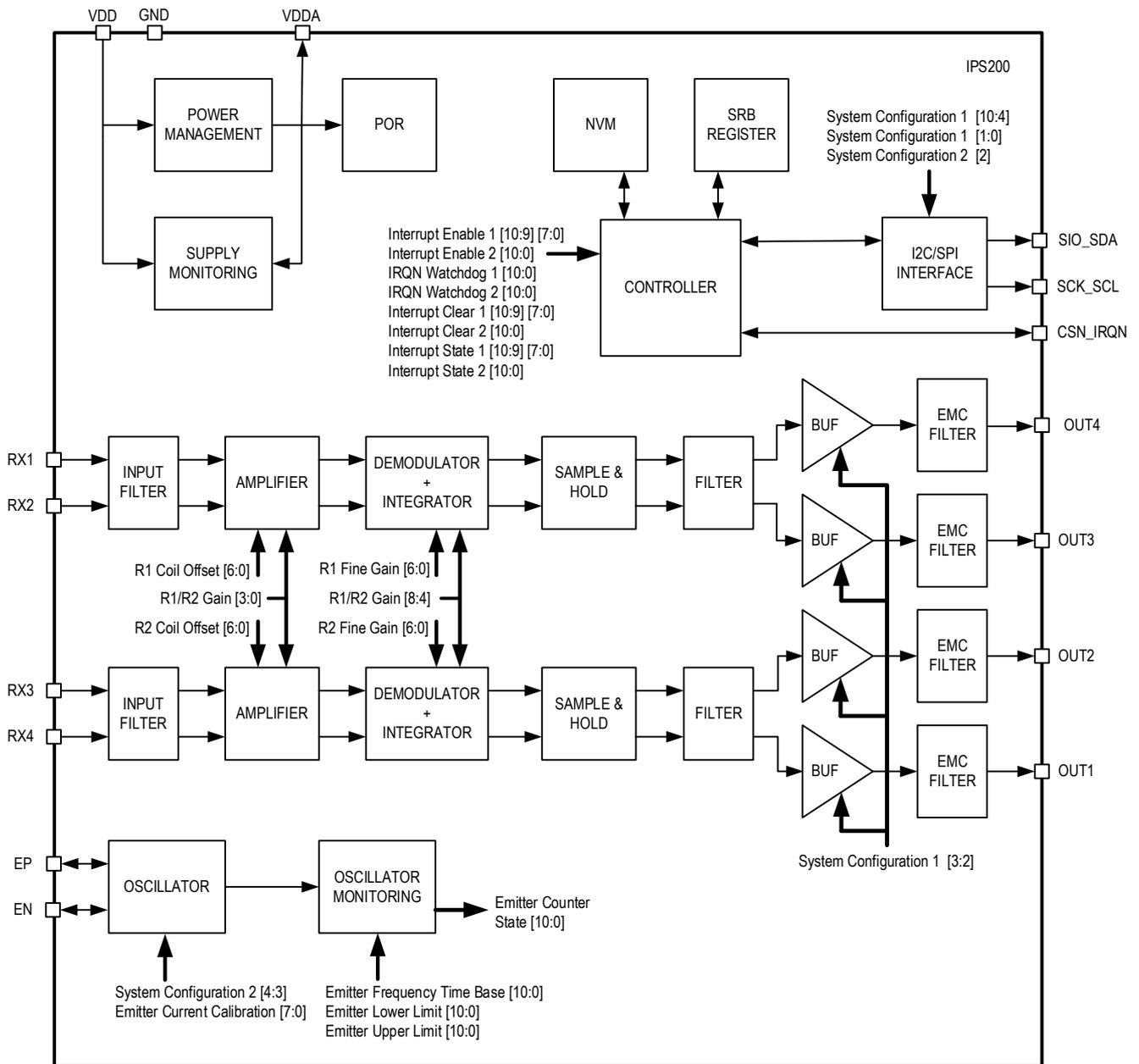
Figure 1. Block Diagram
