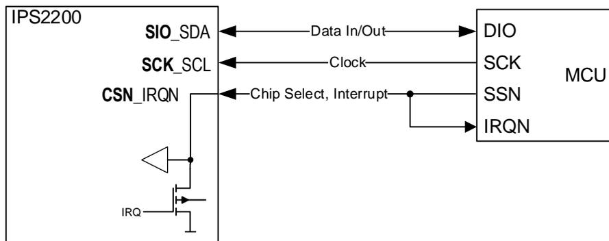
Figure 16. Half Duplex 3-3 Wire SPI Interface with CSN\_IRQN and IRQN Separated at MCU
