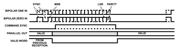
FIGURE 5. DECODER TIMING
