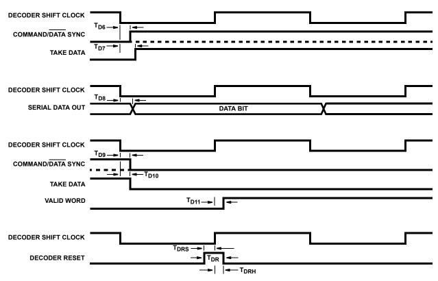
FIGURE 11. DECODER TIMING
