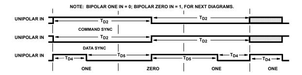
FIGURE 12. DECODER TIMING
