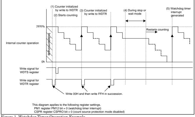
Figure 1 shows an operation timing diagram.
