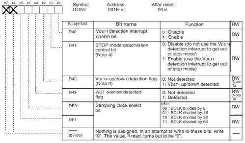
Note 1: Write to this register after the PRCR register's PRC3 bit is set to "1" (write enabled). Note 2: Useful when the VCR2 register's VC27 bit = 1 (VDET4 detection circuit enabled). If the VC27 bit is cleared to 0 (VDET4 detection circuit disabled), the D42 bit is set to 0 (Not detected).
