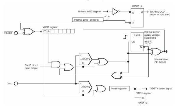
Figure 1 Reset circuit block
