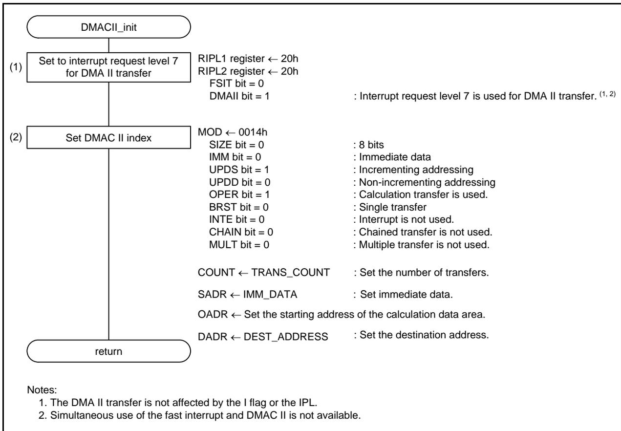
**Figure 5.5 DMAC II Initial Setting**
