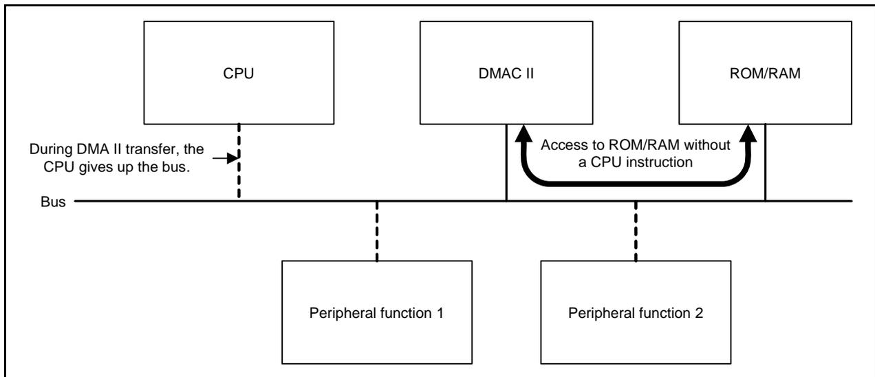
**Figure 1.1 Block Diagram**
