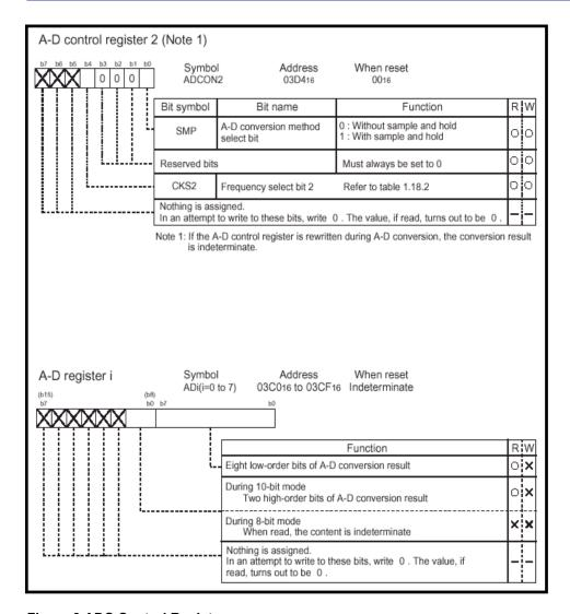
Figure 3 ADC Control Registers
