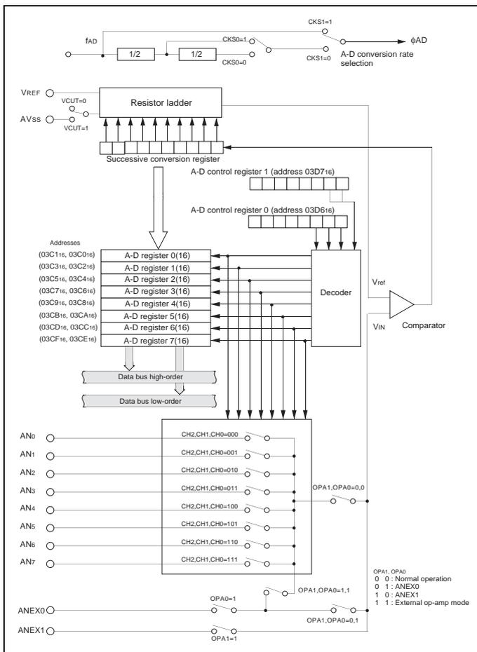
Figure 1 Internal Circuitry for ADC Block—Overview
