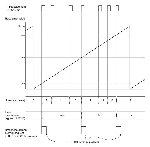
Note: This applies to the second period that the G1TPR6 register decrements after setting the PR bit in the G1TMCR6 register to "1" (prescaler used).
