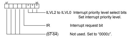
(\*) Use "OR" instruction so that interrupt request bit is not changed when setting the interrupt priority level.
