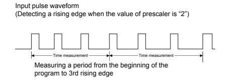
When using the prescaler function, the trigger input is counted, and the time measurement is executed every trigger input of the setting value in the G1TPR6 + 1.
