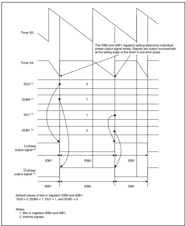
Figure 3.3 U-Phase Output Signal Operation Example
