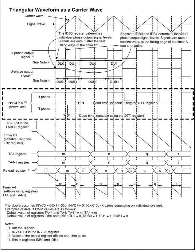
Figure 3.1 Triangular Wave Modulation (Three-phase Mode 1) Operation
