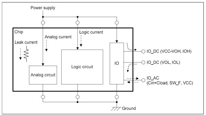
Figure 3.1 Current Path Configuration Diagram
