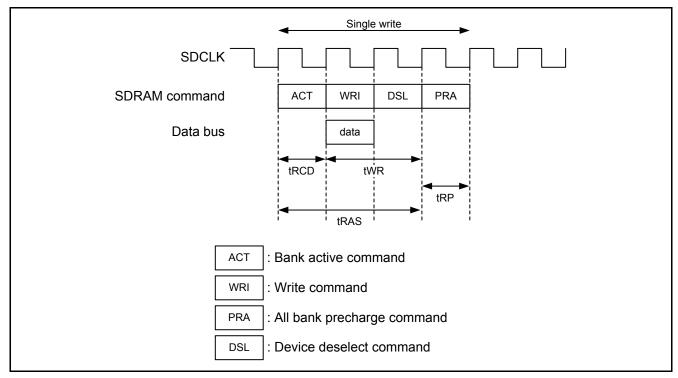
Figure 6.5 Write Timing when the SDRAMC with Setting in Table 6.4 is Used
