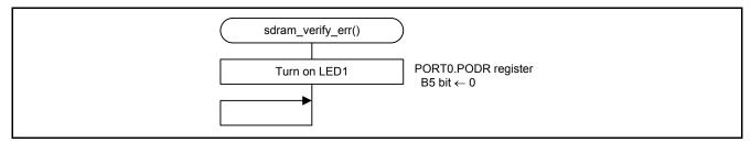
Figure 6.12 SDRAM Verification Error Processing
