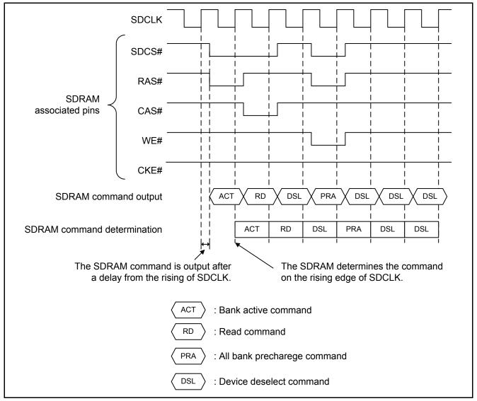
Figure 4.1 Output on Pins Associated with the SDRAM and the Timing of Command Determination
