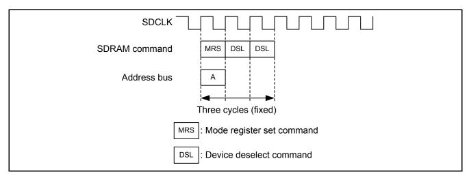
Figure 6.2 Timing Diagram of the Mode Register Set Command
