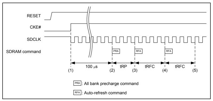
Figure 6.1 Timing of SDRAM (MT48LC8M16A2P-75) Initialization
