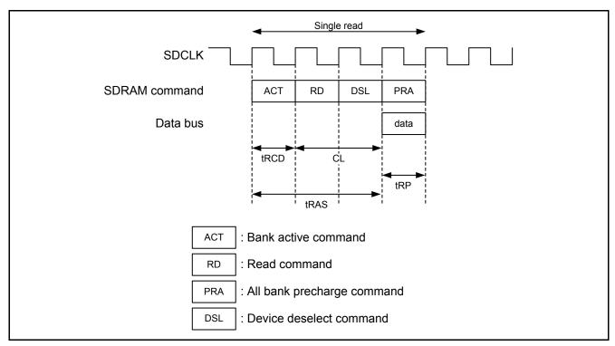
Figure 6.4 Read Timing when the SDRAMC with Setting in Table 6.4 is Used
