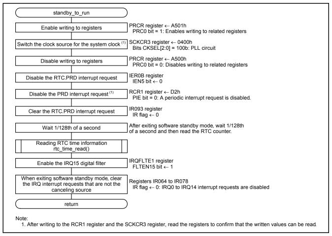
Figure 5.11 Exiting Software Standby Mode
