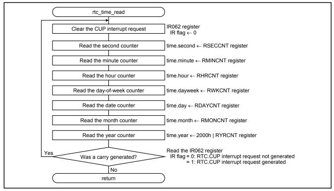
Figure 5.9 Reading RTC Time Information
