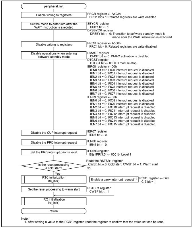
Figure 5.6 Peripheral Function Initialization
