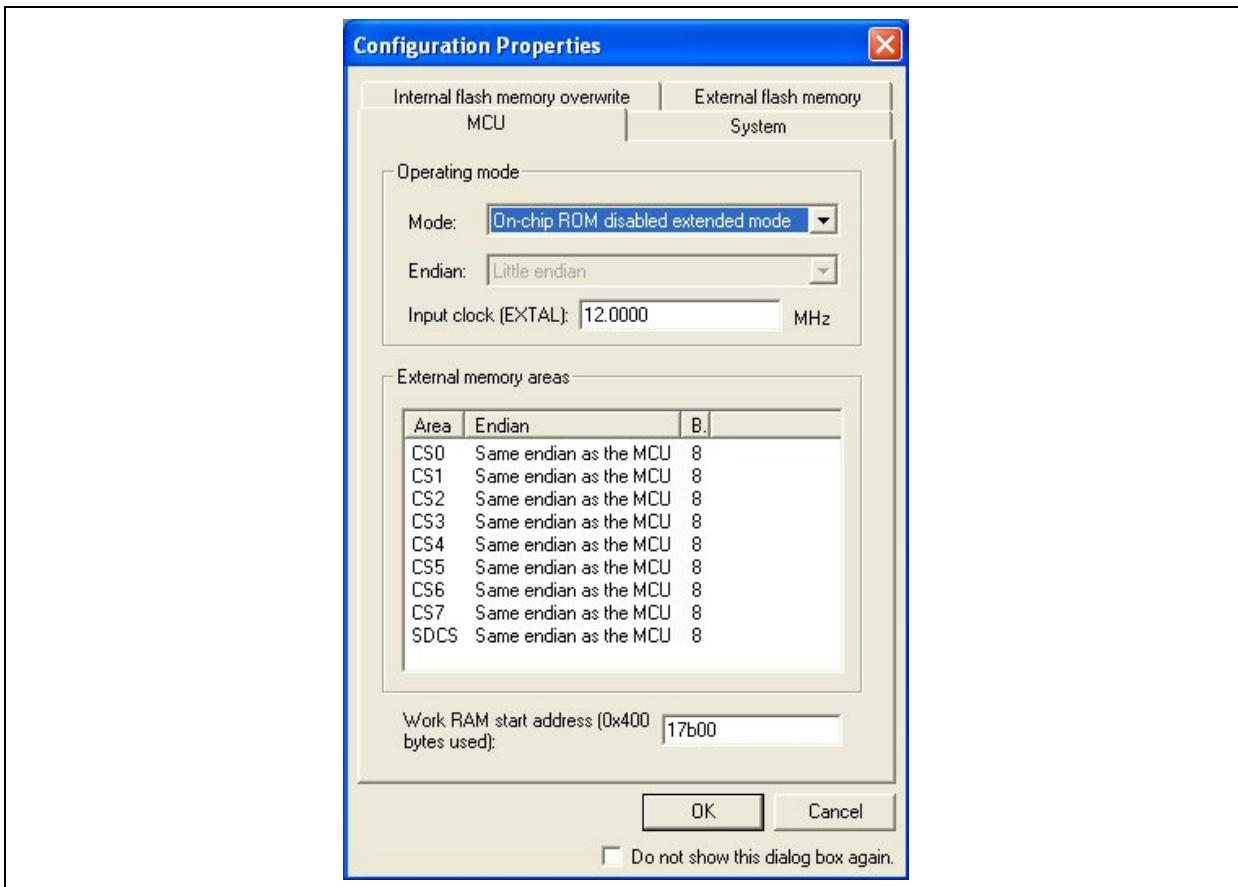
Note that the Work RAM start address should be: 17b00.
