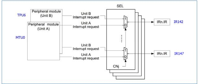
**Figure 2 - Interrupt Unit Selection**
